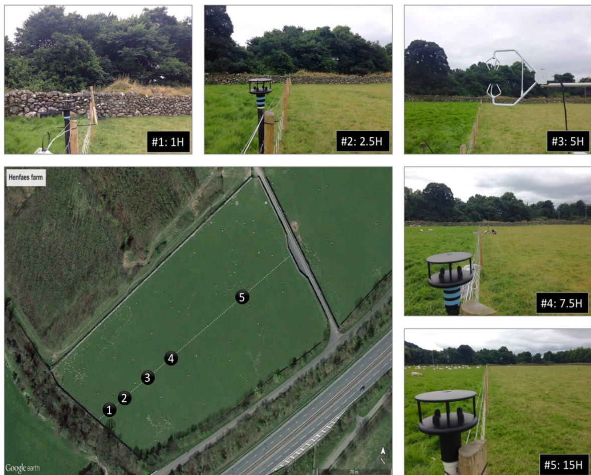
Figure 3 Site map at Henfaes and downwind locations (in barrier height H ) of the five sonic anemometers. Photo taken by Y. He on 2 Aug. 2016, reproduced by Y. Xuan. Map credit: Google Earth.
