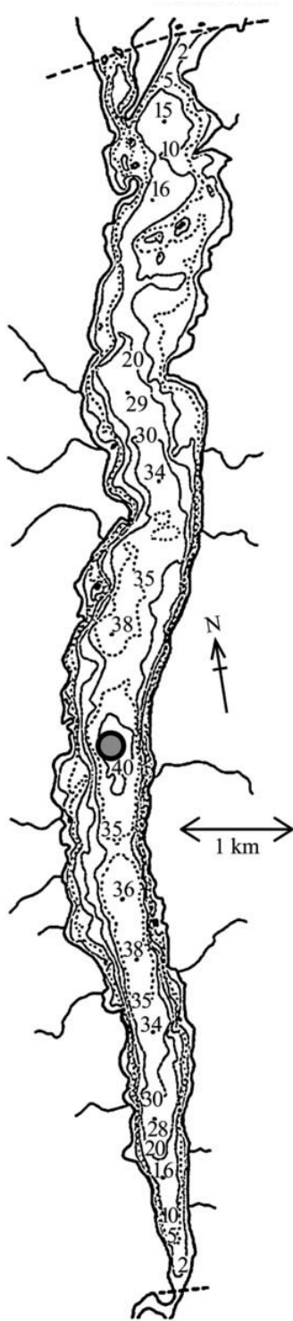
Figure 1. Bathymetric map, with contours in metres, of Windermere South Basin (after Ramsbottom 1976) showing the location of the instruments (filled circle; depth ~ 40 m) used in the investigation.
