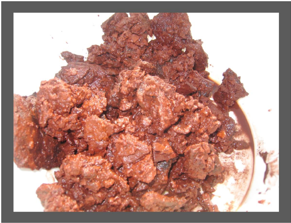
Figure S2. Internal texture of DFS structure represented by amorphous ferrihydrite-type Fe-oxyhydroxides occurring as an extensive slime-like material.
