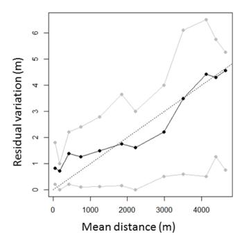
Figure 1. The residual variation of range measurements as a function of distance to a fixed, 1  $\text{m}^2$  target, as measured by the VOD (n = 120 fixes, 10 fixes per distance interval). The standard deviations are given in black, while the minimum and maximum deviations are given in grey for each distance. The dashed line indicates the variance that would be equivalent to 0.1% of the distance value.
