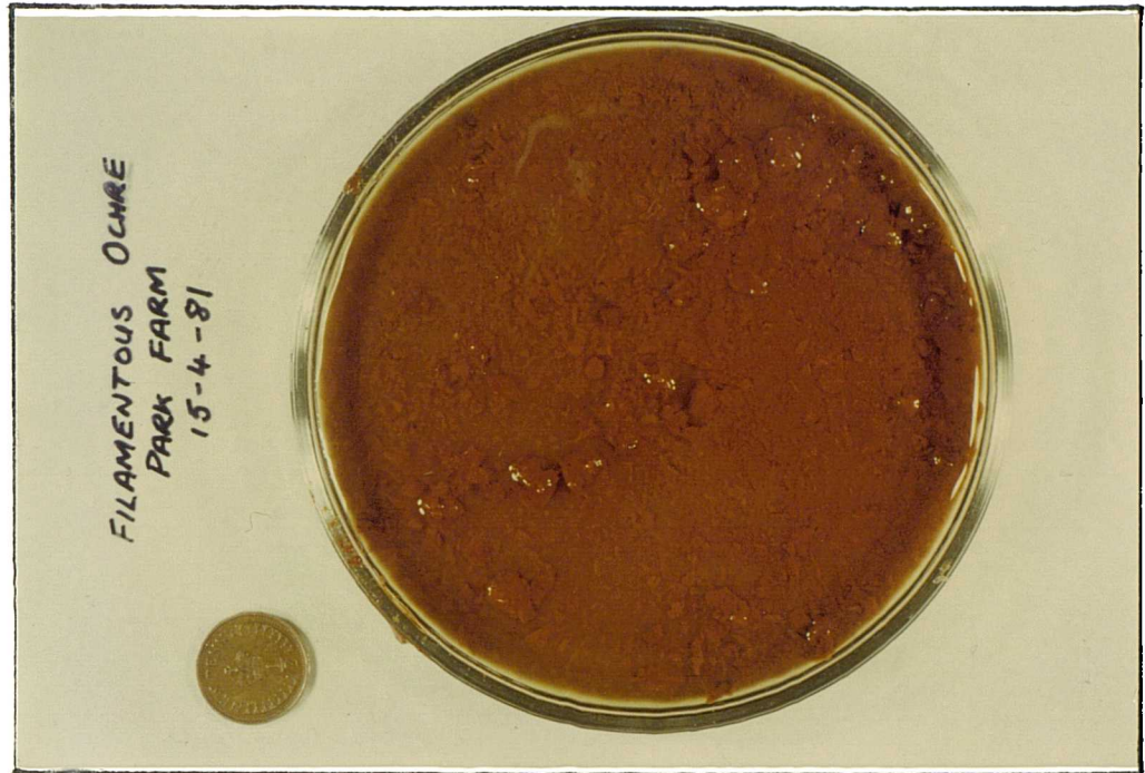
Plate 3:27 Petri dish containing ochre from a field drain outfall from Park Farm.
