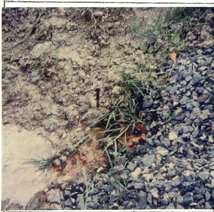
Plate 3:13 Machynlleth site 1 : gravel coated with ferric iron deposits.
