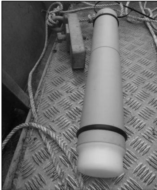
Figure 1.12 Photograph of a C-POD prior to deployment attached to a rope and weights.
