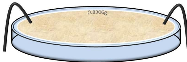
Figure 5.3 | The sediment trap. Filter papers were used to trap any sediment deposited on the marsh surface. The filter papers were held off the marsh surface using an upside down petri dish and held in place using tent pegs.
