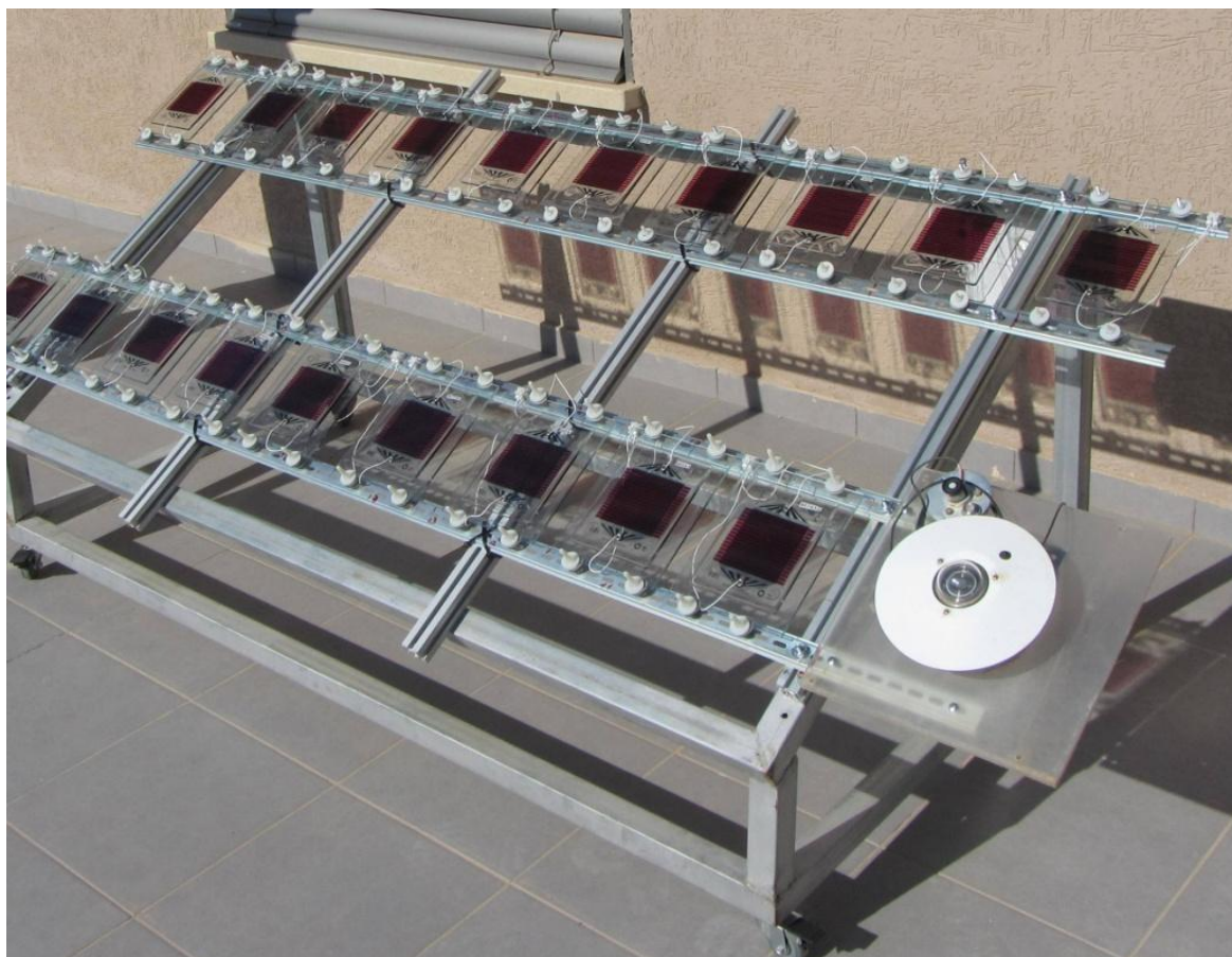
Figure 4.25: Outdoor OPV rack at Jacob Blaustein Institutes for Desert Research, in the Negev Desert.
