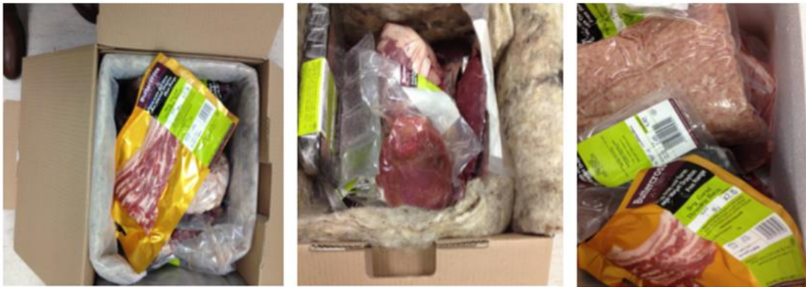
Figure 1. Sample boxes with meat (left-right: Woolcool ® lined, Woolcool ® unlined, expanded polystyrene ).
