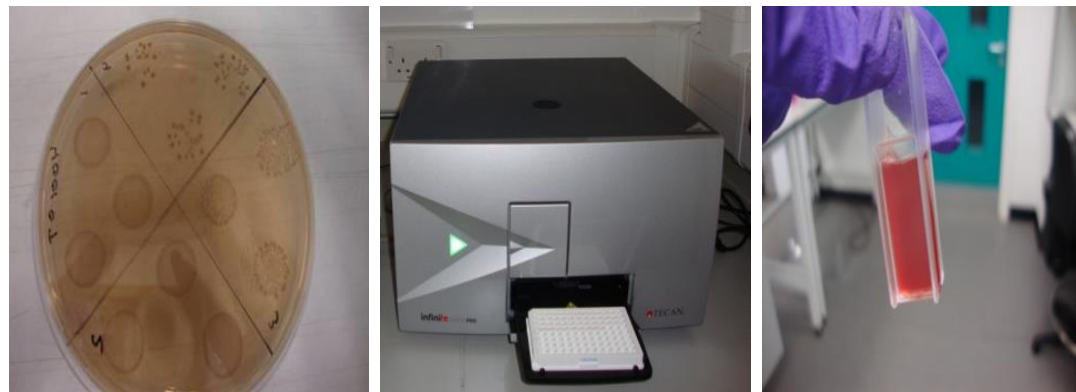
Figure 7. Procedure of microbial assessments of Ch-arg; A: cell count, B: luminescence, C: OD
