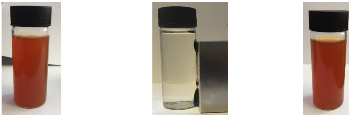
Figure 4.5 SPIONs in the absence of a magnetic field (left); in the presence of a 1T magnet (middle) and in the absence of a magnetic field after magnetic exposure (right).
