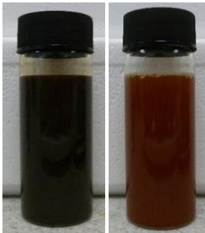
Figure 4.1 SPION produced from the Massart method 6 (Left) SPIONs after initial co-precipitation, (Right) SPIONs after magnetic and centrifugal separation and final stabilisation in TMAOH.
