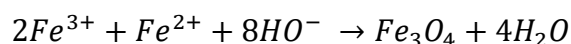
Equation 2.1 Formation of magnetite from aqueous iron ions in a non-oxidising environment
