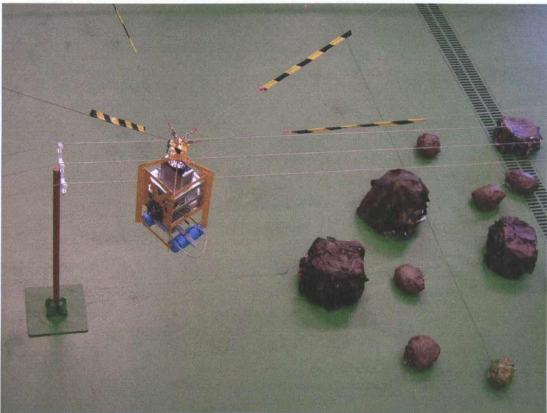
Figure 7.40: The AVS Pod suspended above a Model Power Line.
