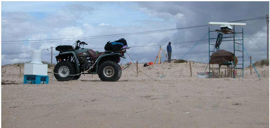
Figure 4.4.1 The two radars deployed simultaneously during a storm on Faro beach in 2002. The mm wave radar can be seen on the left, and the X-band radar on the right, the photograph being taken looking approximately inshore.
