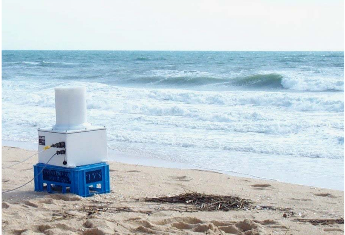
Figure 3.7.1 The Navtech mm wave radar deployed on an improvised mounting on the beach in Faro 2002.
