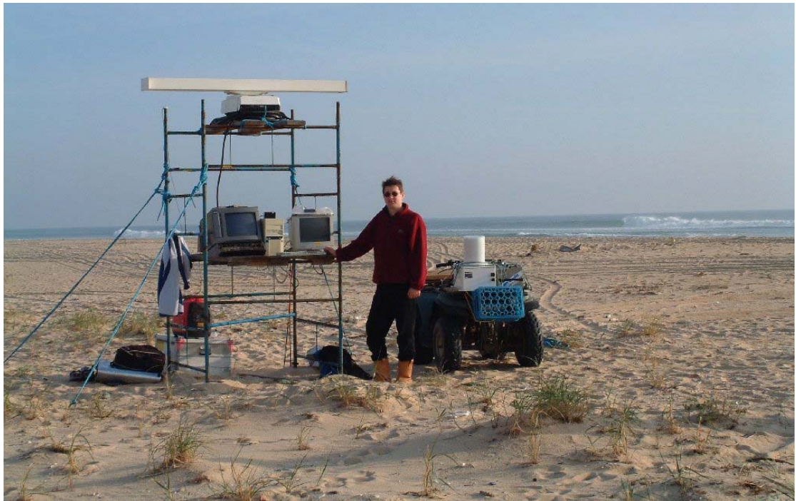
Figure 4.5.1 The X-band radar set up at the end of the Ancao peninsula overlooking the inlet during the Faro 2003 deployment.
