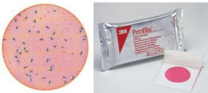
Fig.3. Petrifilm plates for the enumeration of E. coli and coliforms.
