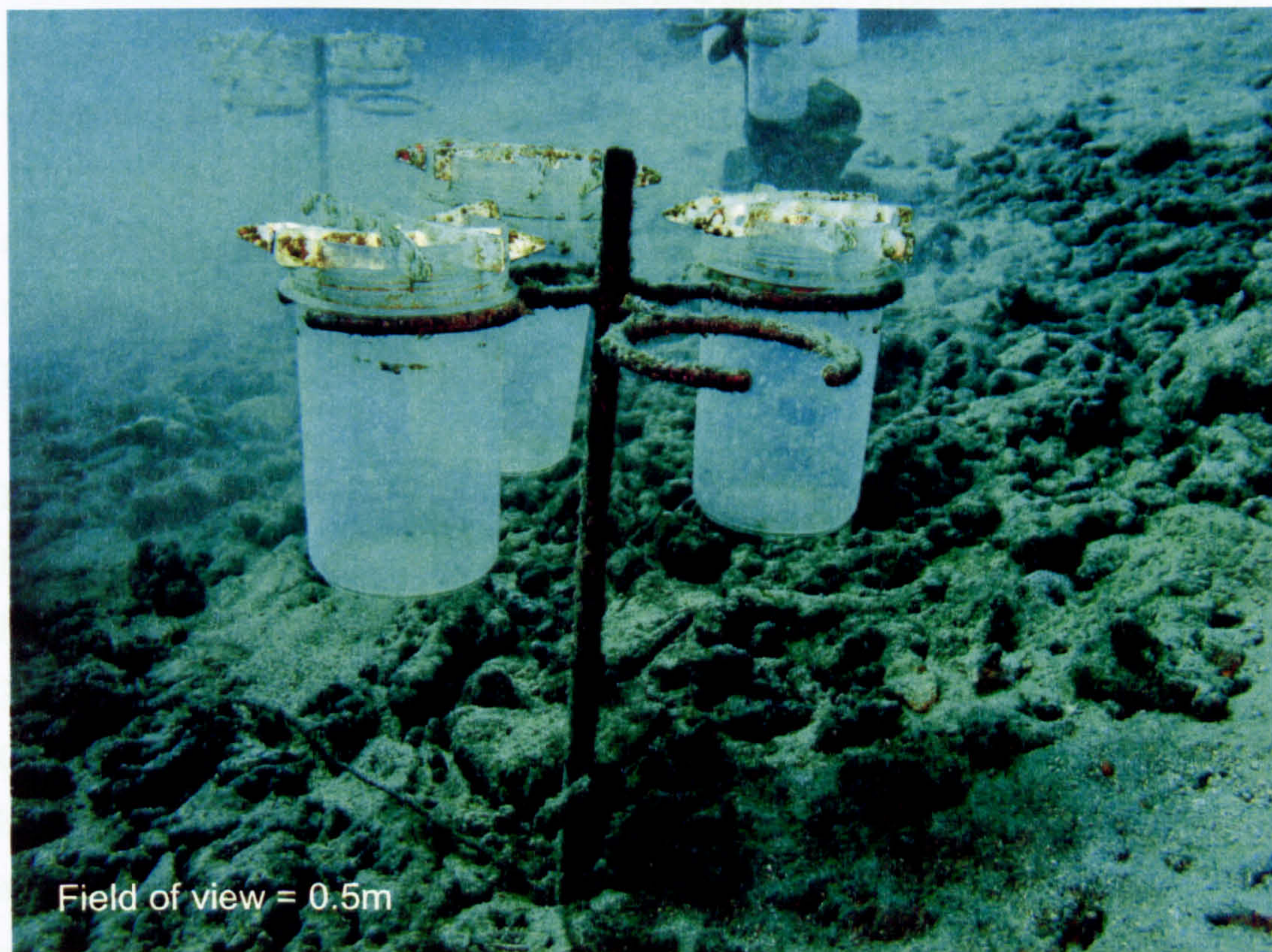
Plate 2.1 A sediment trap stand containing 3 sediment traps on the reef at Trou Malabar.
