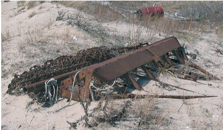
Figure 1. 3 Picture of a standard Newhaven scallop dredge (from Kaiser et al. 2006a) (Photograph ©Michel Kaiser)
