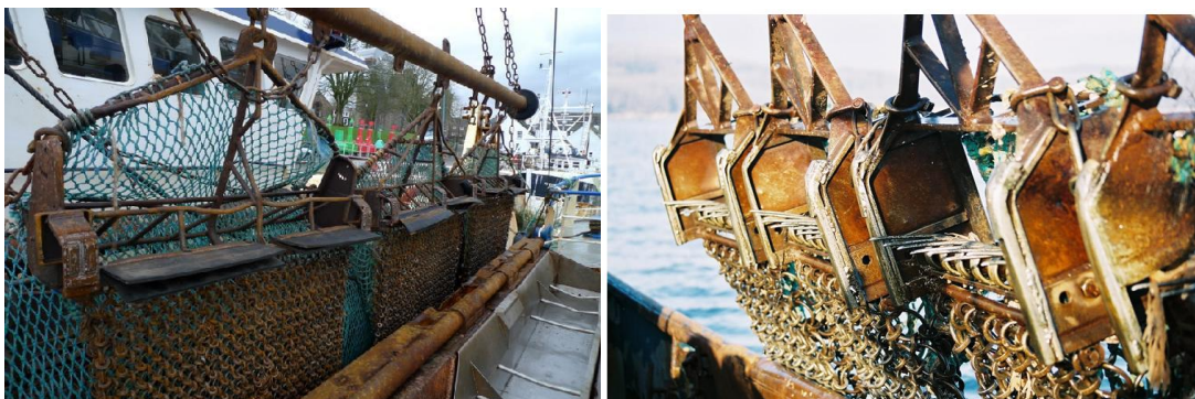
Figure 1. 4 Modified dredges. Left: New scallop dredge used around the Isle of Man (Andrews et al. 2011); right: N-Viro dredge ( http://www.n-virodredge.com/ )
