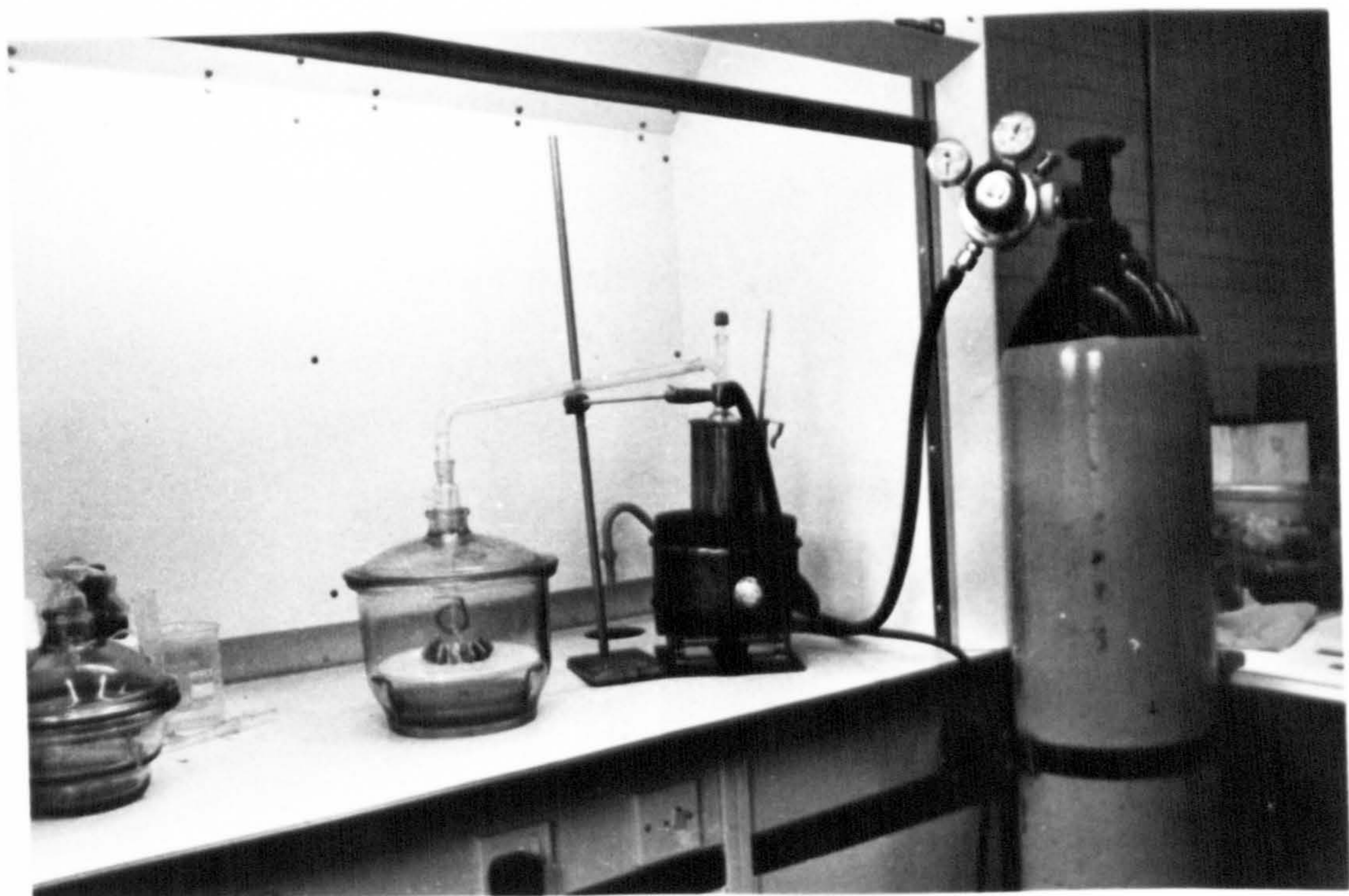
Figure 4.2. Silanation of wafer specimens by vapour phase.
