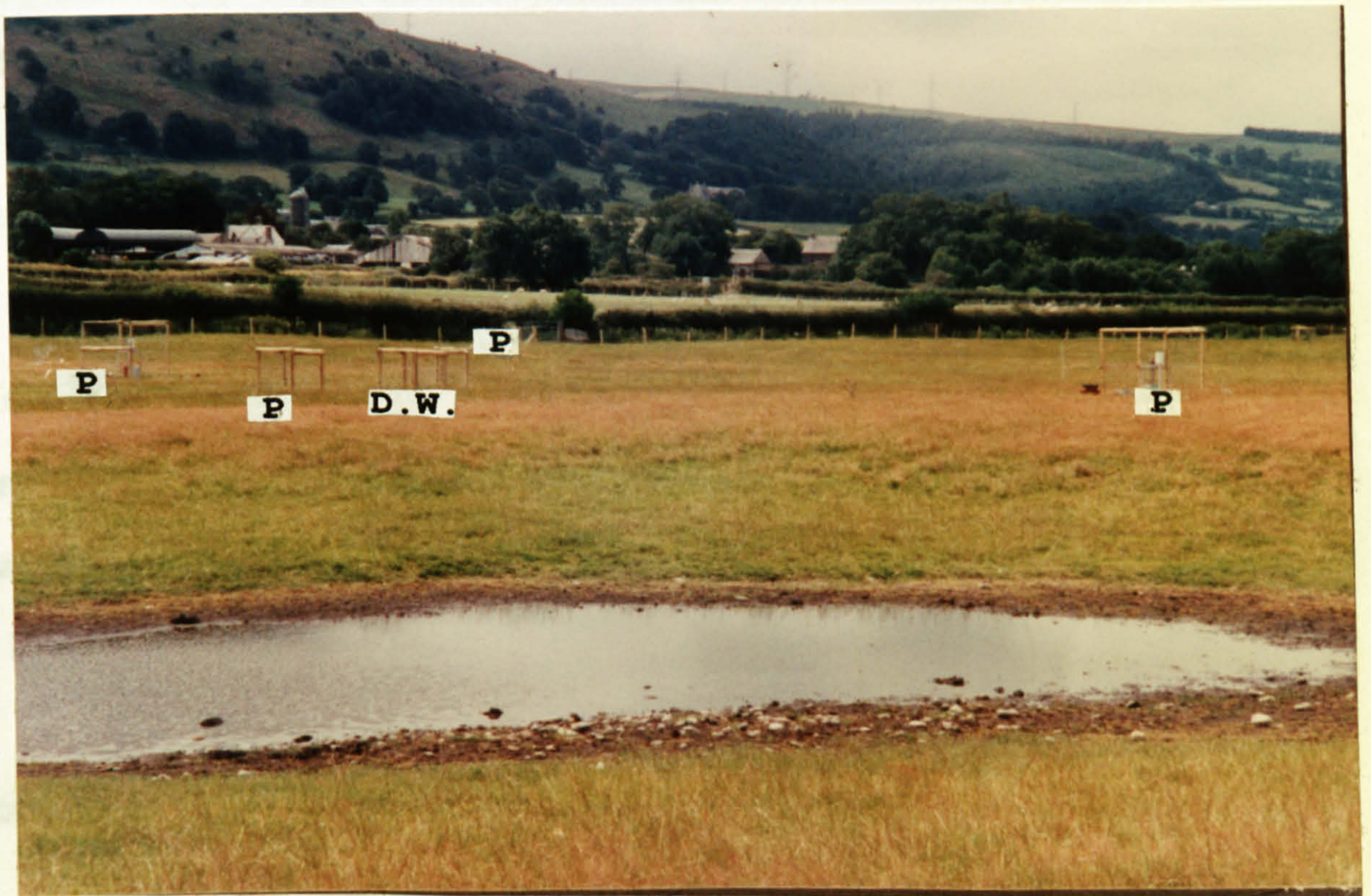
Photographic Plate 4.6.b Showing a discharging well and piezometers. D.W = Discharging well, P = Piezometer.
