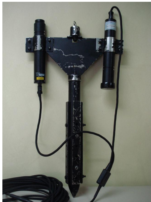
Figure 2.3: Satlantic Hyper OCR downwelling (right) and upwelling (left) radiometers are mounted on a horizontal T-plane frame.
