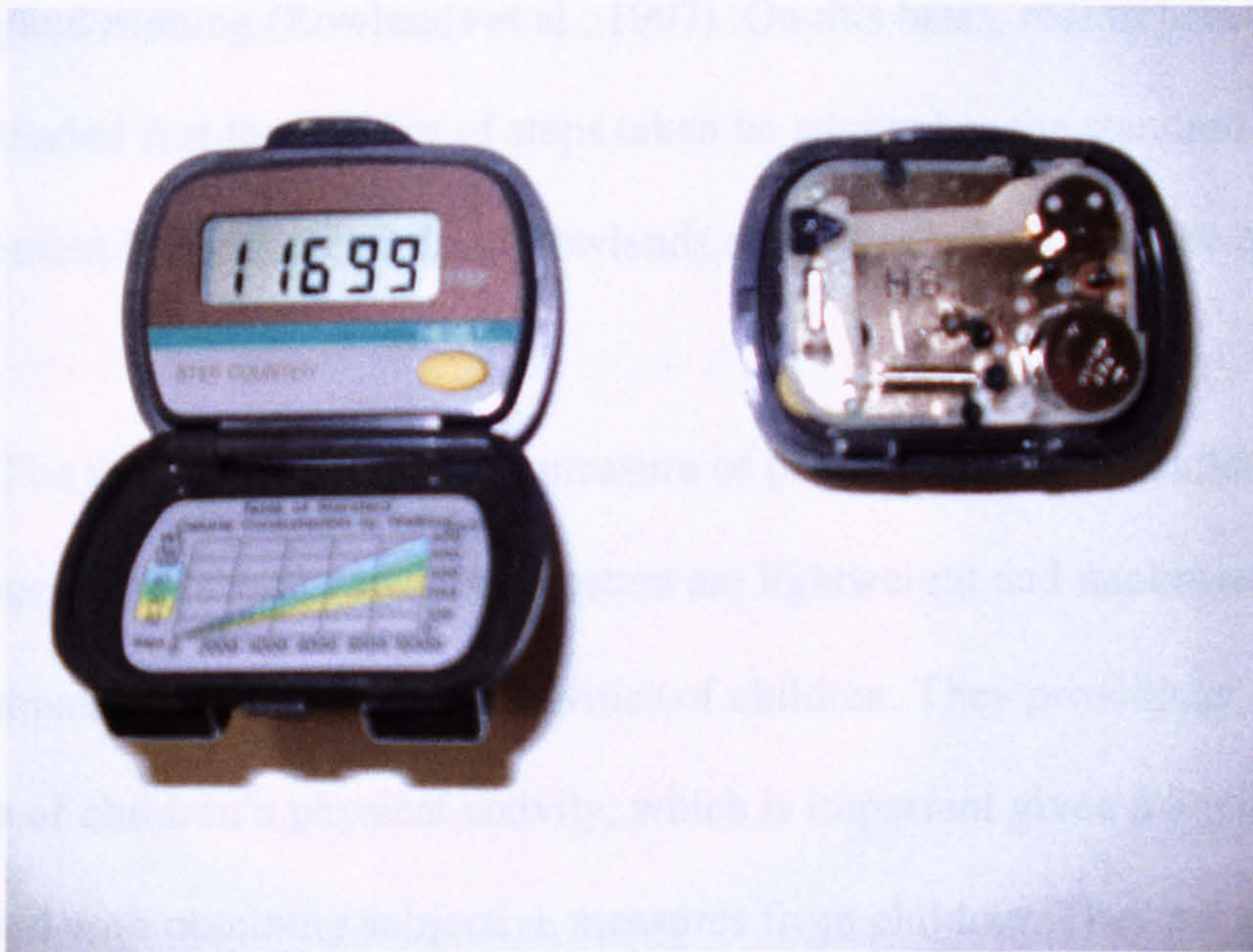
Figure 2.1. The Yamax Digiwalker SW-200 pedometer (Tokyo, Japan), on the left with the case open so that the display may be viewed, and on the right with the back removed to show the internal mechanism.
