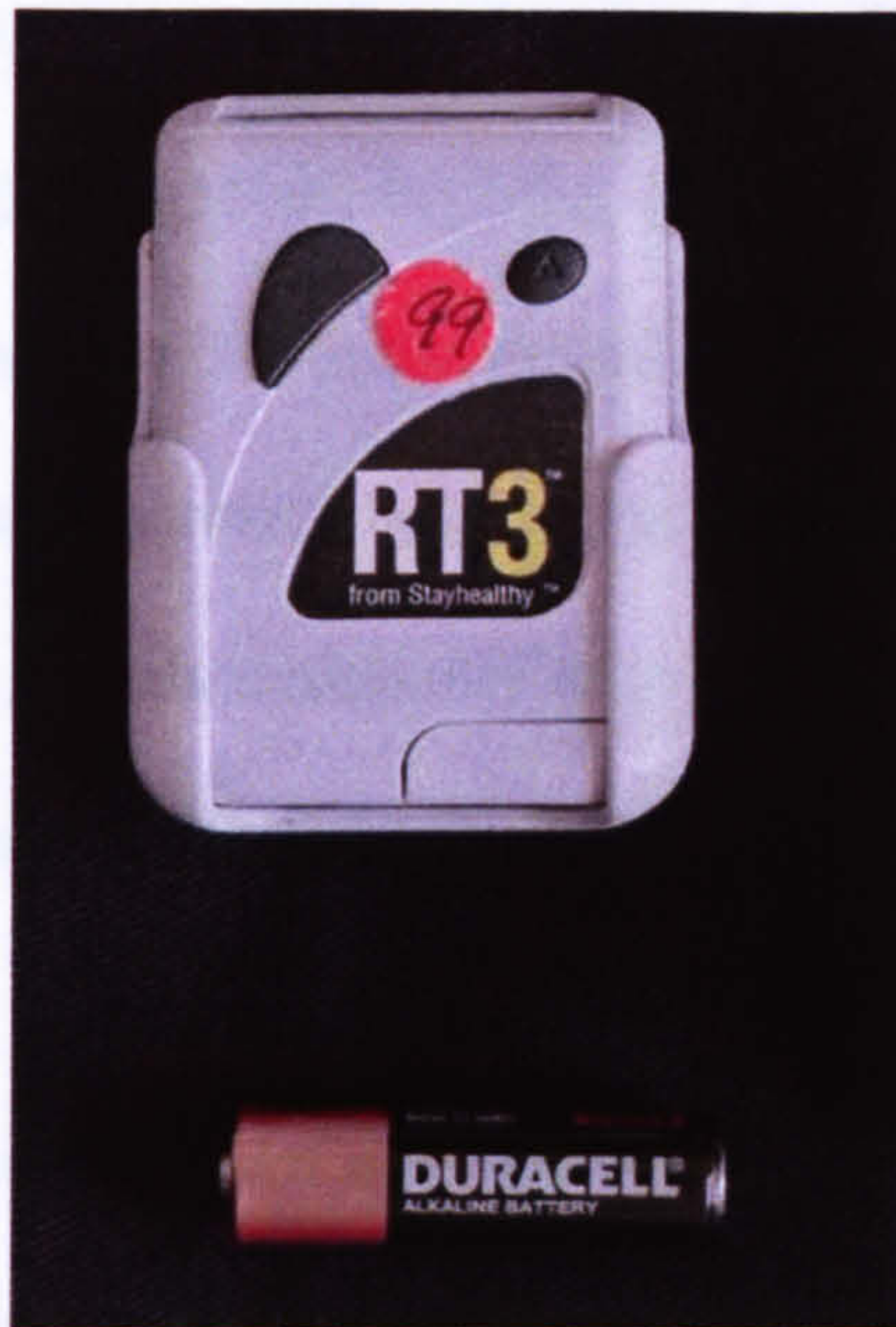
Figure 2.2. The external appearance of the RT3 triaxial accelerometer, with an AAA battery also shown.
