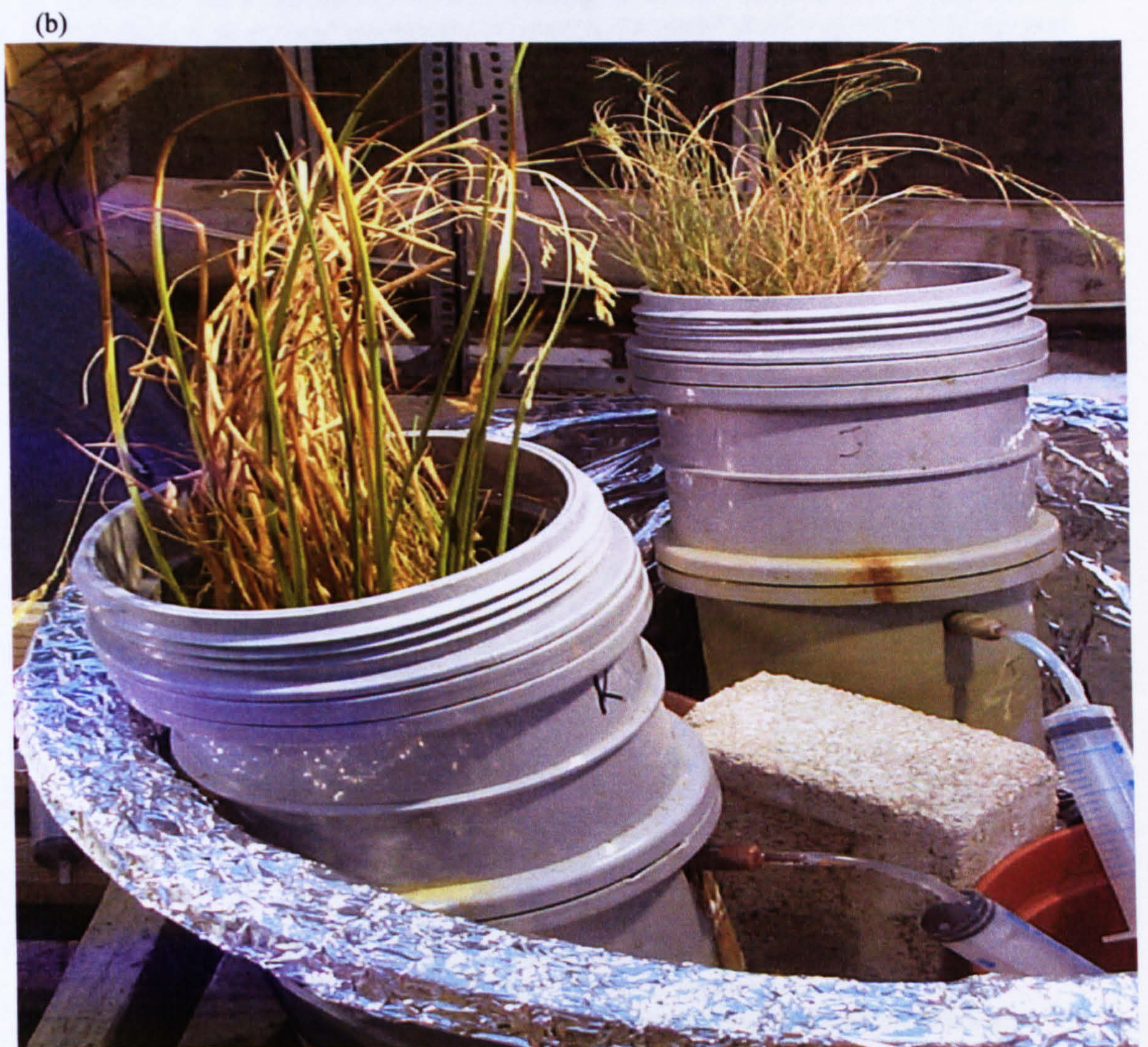
Figure 4.11 showing perfusion systems for maintaining intact peat cores (a) inside ^{13}\text{CO}_2 pulse labelling isotope chambers & (b) with lateral sampling ports for leachate collection.
