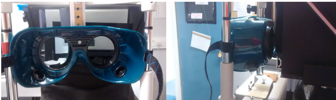
Figure 2.1.2. – The chin and forehead rest. The image on the left shows the goggles straight on. A black cardboard septum ensured that the right eye could not view the images for the left eye and vice versa. The image on the right shows the side of the glasses, illustrating the chin rest below.
