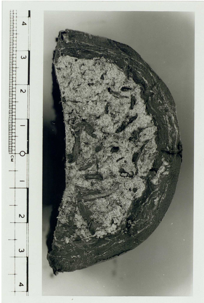
Fig.3.25 Photograph showing the disturbed 'outer' zone and bioturbation within fine sands and silts of vibrocore 51/-07/199 from the central Celtic Sea.
