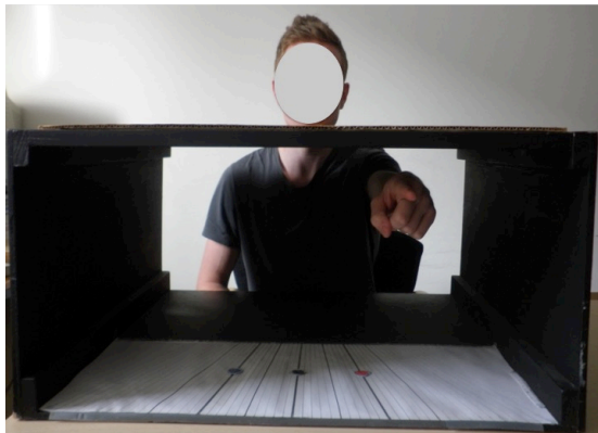
Figure 3.2a. Open loop pointing: Markings under the lid (in-situ) facilitate pointing accuracy measurement by the experimenter.
