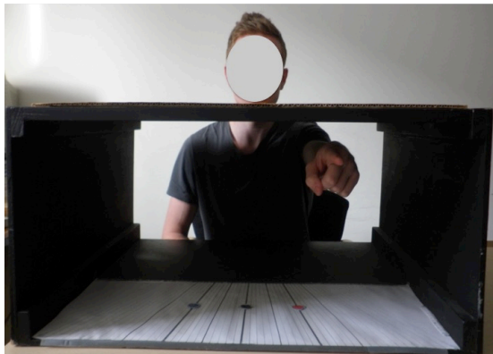
Figure 3.2a. Open loop pointing: Markings under the lid (in-situ) facilitate pointing accuracy measurement by the experimenter.
