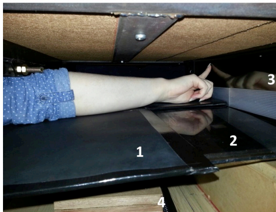
Figure 2.3: Apparatus underside view with handboard in place for finger location task. 1) Movable top handboard, 2) perspex covered bottom board attachable to main frame, 3) touchscreen, 4) partial view of height-adjustable support (under handboard) Note: photo is for illustrative purposes, the hand and fingers were relaxed during experimental task.
