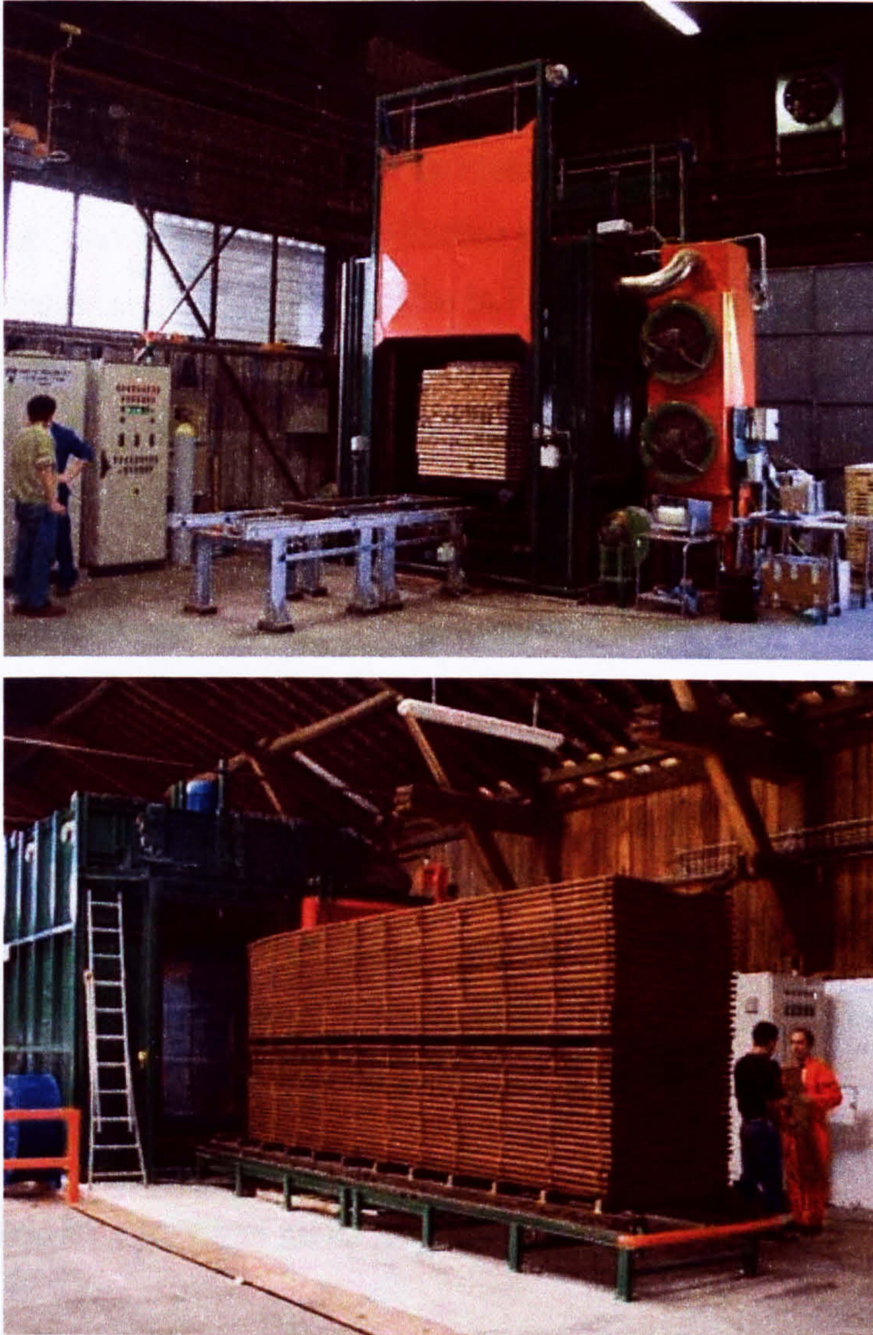
Figure 2.1 The process for the thermal modification of wood in France
