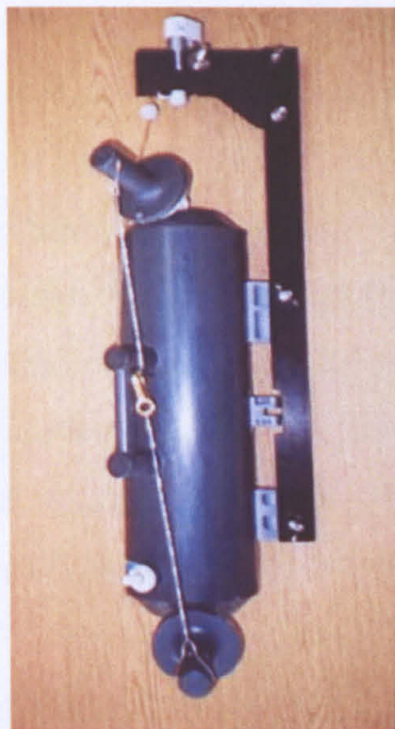
Fig. 4.07 A Niskin bottle which is used to collect water samples for gravimetric analysis.
