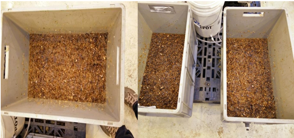
Figure 2. Wood chips soaked lignin was prepared at 5, 10 and 15% w/v concentrations used in Chapter 3.
