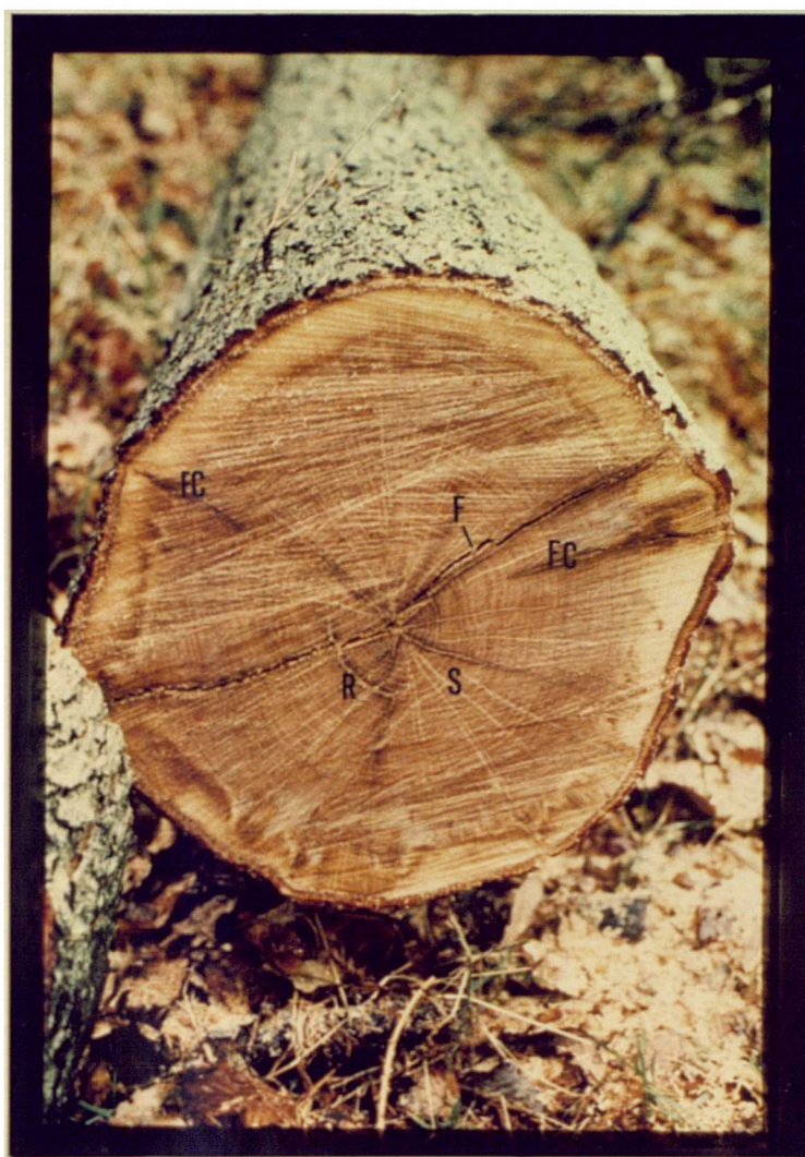
Plate 3.9. Cross section of oak butt showing frost-cracks (FC) and associated ribs; star shake (S), ring shake (R) and a felling crack (F) are also present.
