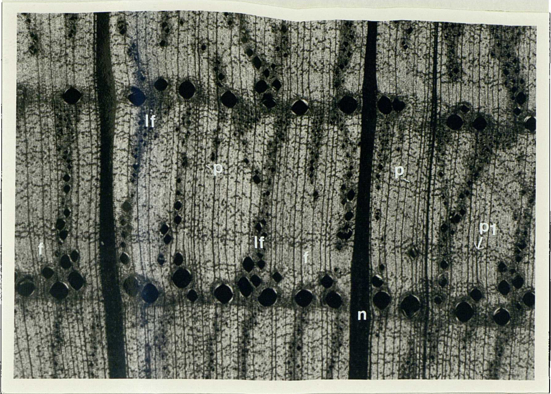
Plate 5.1. Cross-section of 1971 ring of oak. x 20.
