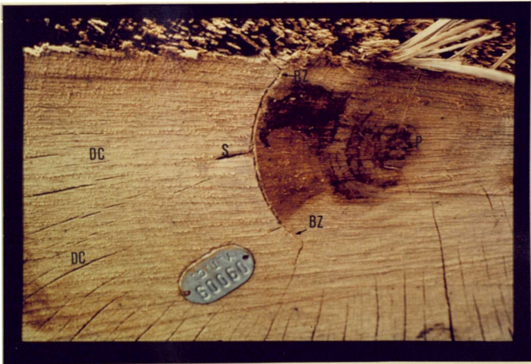
Plate 3.6. Cross-section of oak butt showing pith (P) and compartmentalised rot behind barrier zone (BZ). Ring shake has formed at barrier zone, and star shake (S) is developing from ring shake. The causative wound was below level of section. The small splits (DC) are drying checks.
