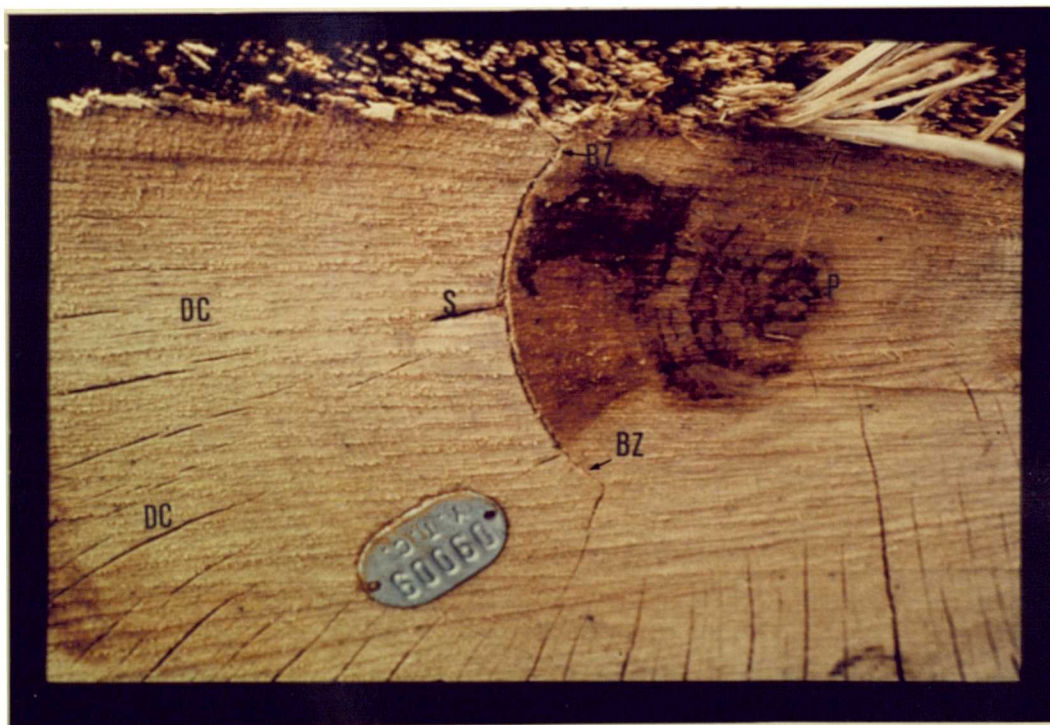
Plate 3.6. Cross-section of oak butt showing pith (P) and compartmentalised rot behind barrier zone (BZ). Ring shake has formed at barrier zone, and star shake (S) is developing from ring shake. The causative wound was below level of section. The small splits (DC) are drying checks.
