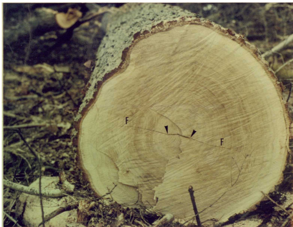
Plate 3.8. Sound oak butt, showing heart crack (between arrows; extended by felling shock, F).
