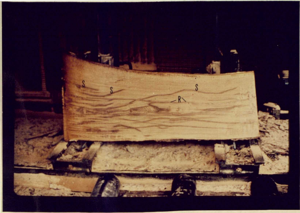
Plate 3.3. Star shakes (S) and ring shake (R), seen in longitudinal section of oak log.
