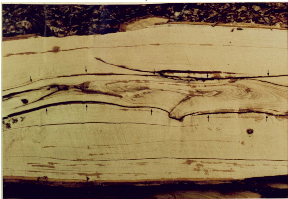
Plate 3.4. Ring shake in sweet chestnut ( Castanea sativa ), seen in longitudinal section, following a complete annual ring (arrows).
