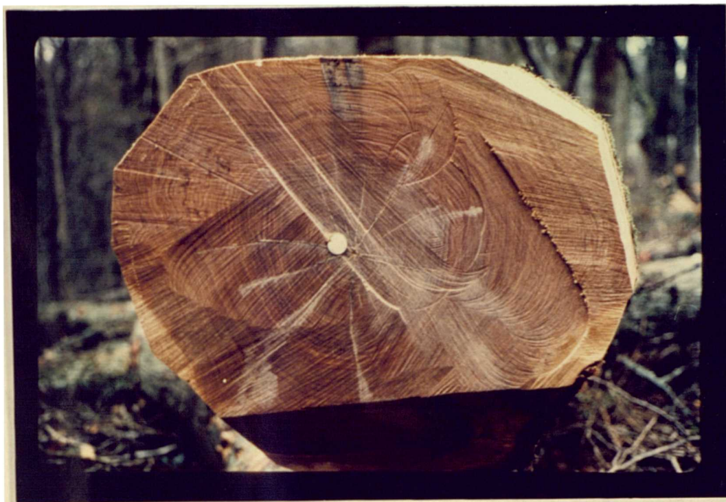
Plate 3.1. Star shake, seen in cross-section of oak butt. Note white stain spreading from shake splits.
