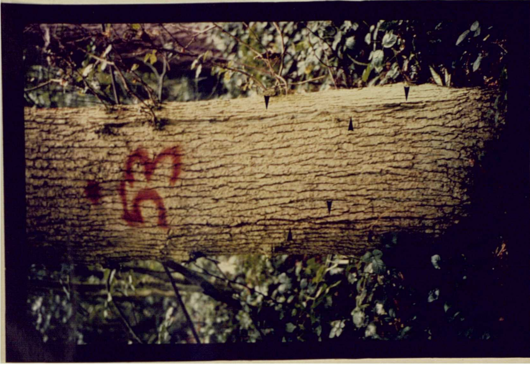
Plate 3.16. Healed cracks on oak bole which may indicate a shaken interior.
