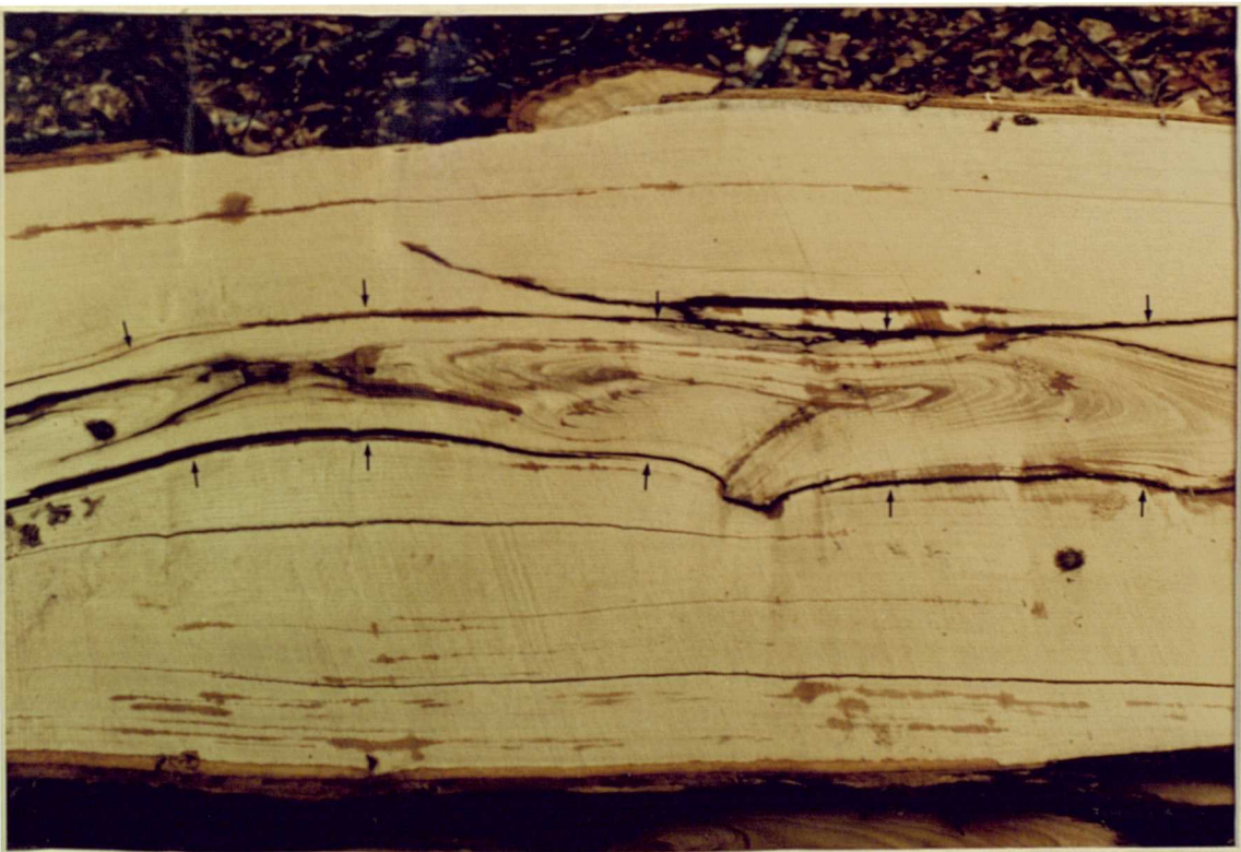
Plate 3.4. Ring shake in sweet chestnut ( Castanea sativa ), seen in longitudinal section, following a complete annual ring (arrows).
