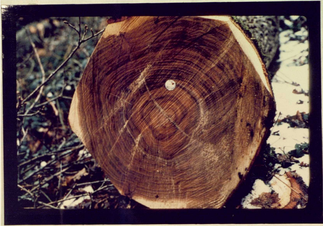
Plate 3.11. Mineral stain (dark banding) in shaken oak.
