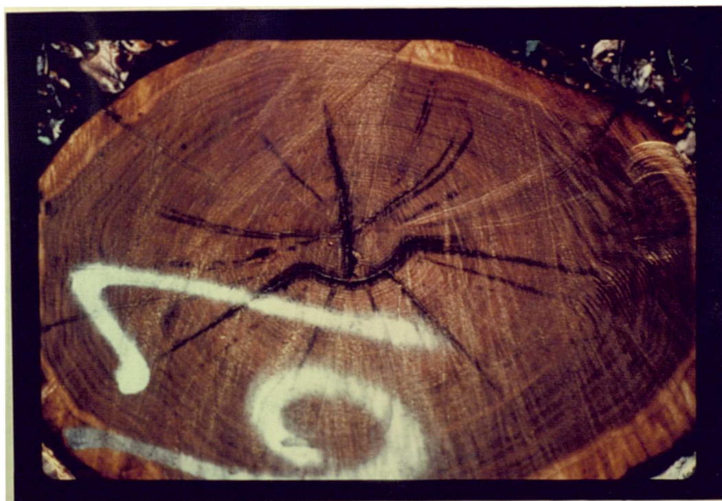
Plate 3.2. Ring and star shakes, seen in cross section (stump) of oak. Shakes are dark-stained; some star shakes run from the ring shake, without any origin at the pith.
