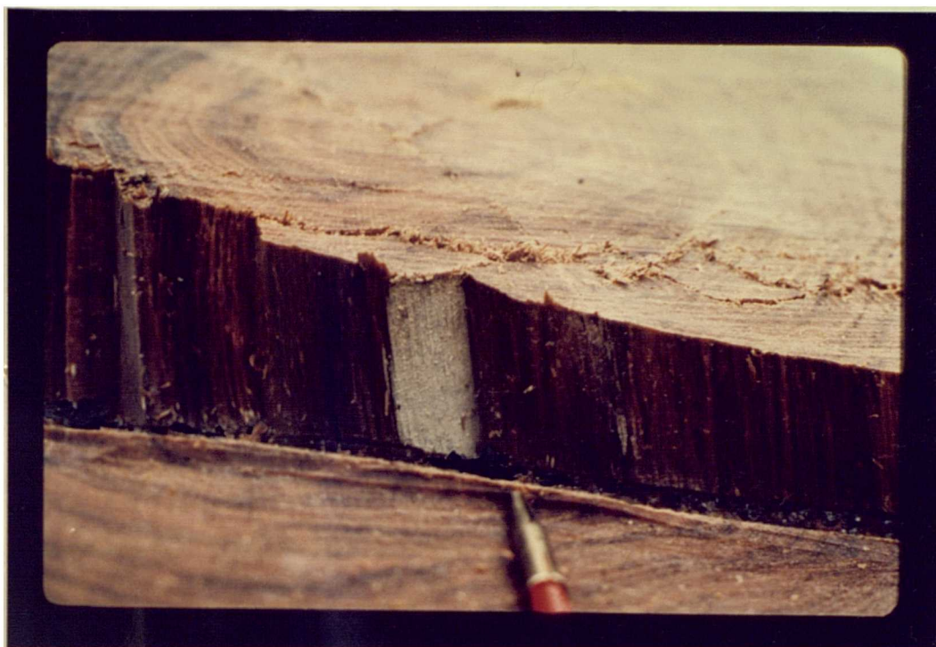
Plate 3.7. Felling hinge on oak stump, showing chalky, white deposit on tangential longitudinal surface.
