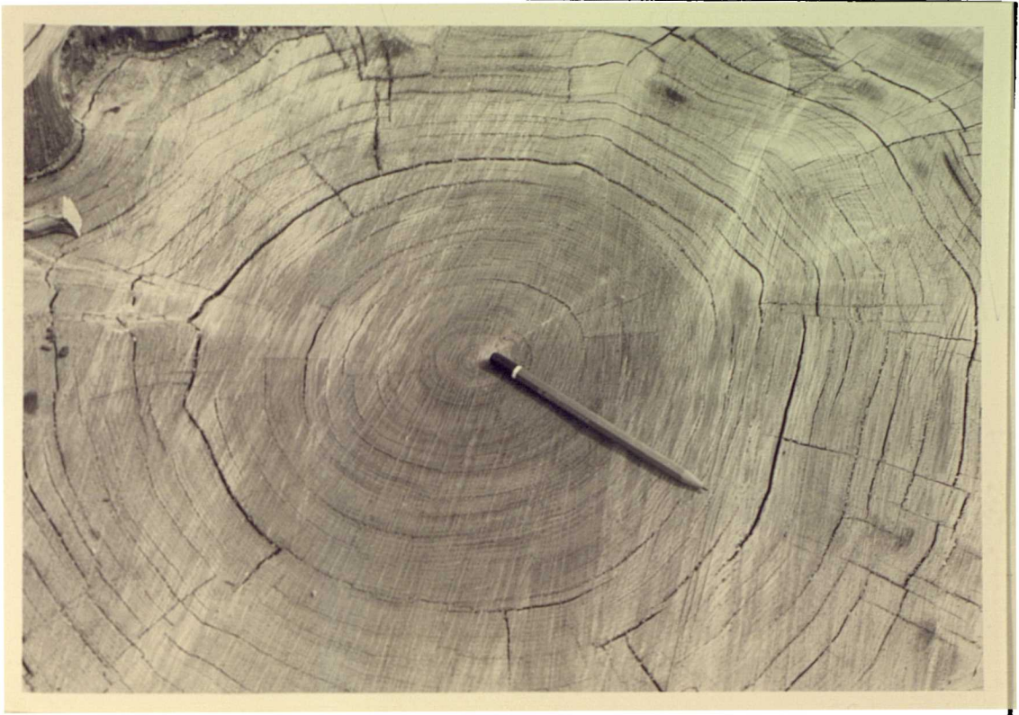
Plate 3.5. Ring shake in sweet chestnut, seen in cross-section. (Pencil for scale = 14 cm long).
