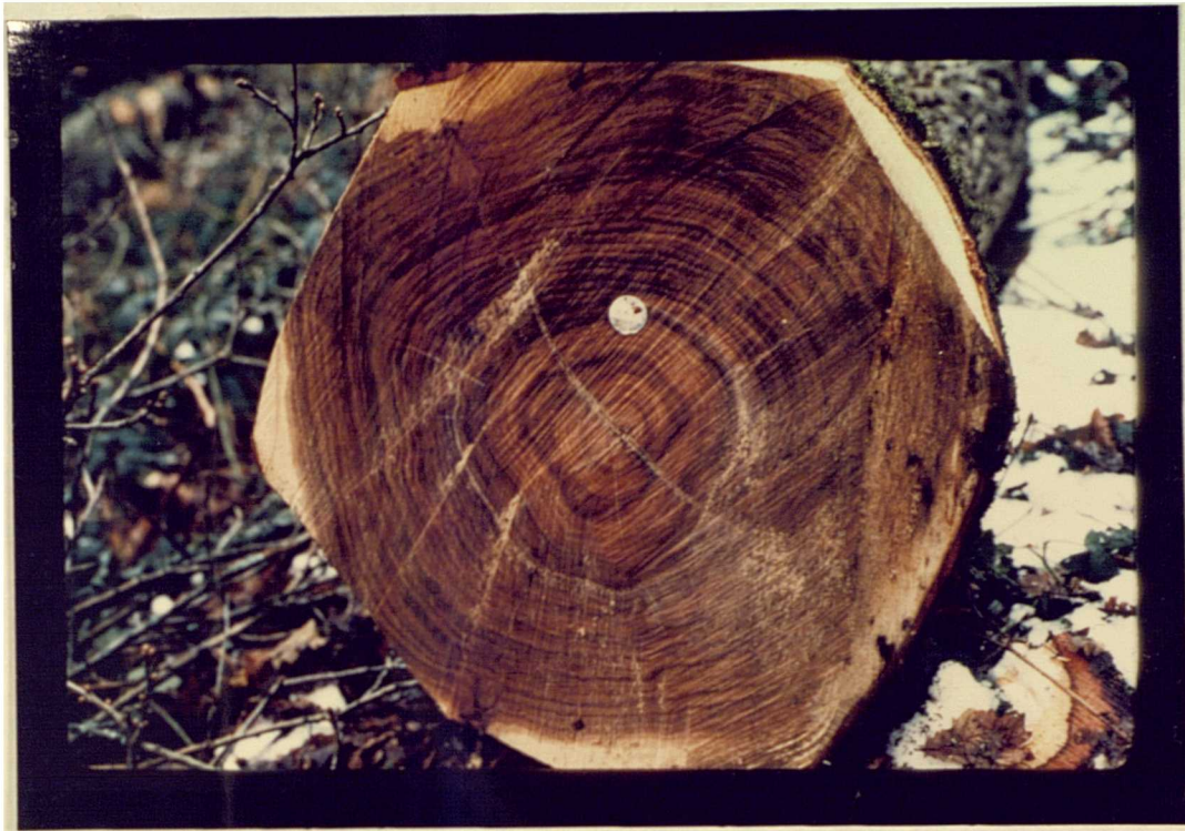
Plate 3.11. Mineral stain (dark banding) in shaken oak.
