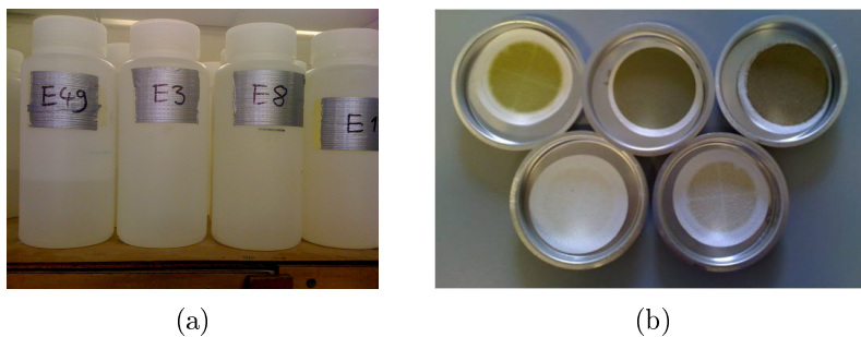
Figure 3.7: Examples of (a) water samples collected and (b) post-processed SPM filter papers
