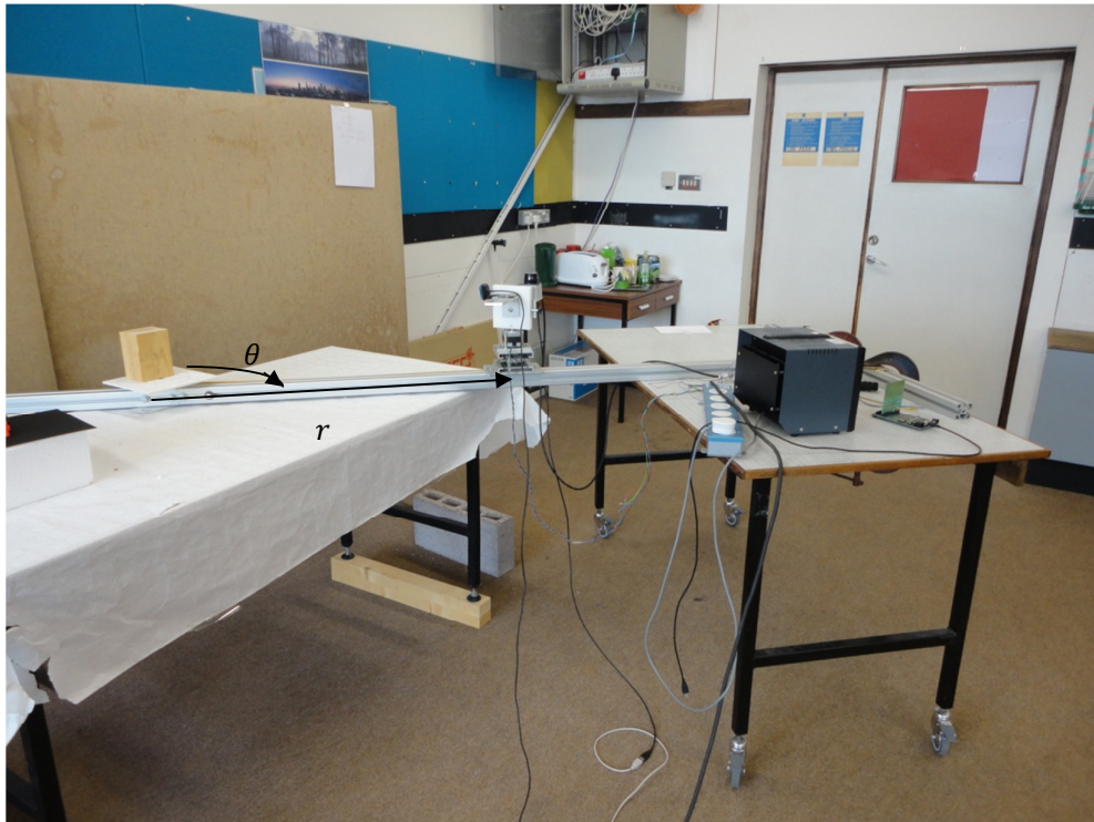
Figure 34 – 2 nd Test rig pivoting around target
