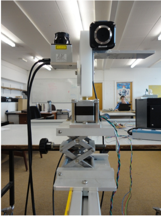
Figure 36 – Second test rig with Sensor suite mounted on simulated UAV
