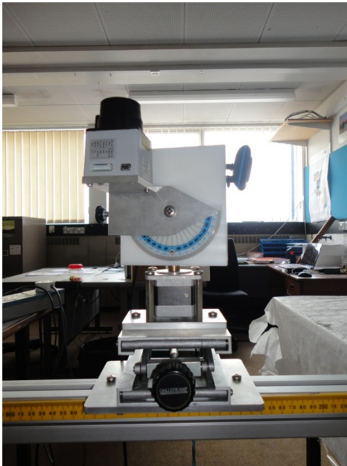
Figure 35 – Second test rig with Sensor suite mounted on simulated UAV
