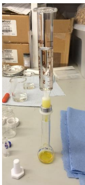
Figure 3.8: Elution of the liquid contents of a DNPH cartridge with acetonitrile using a glass syringe.
