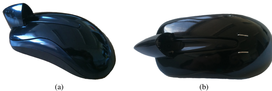
Figure 3.11: Early Shark-Fin prototype casing; (a) before attaching sensors and (b) with EDA and PPG sensors included.
