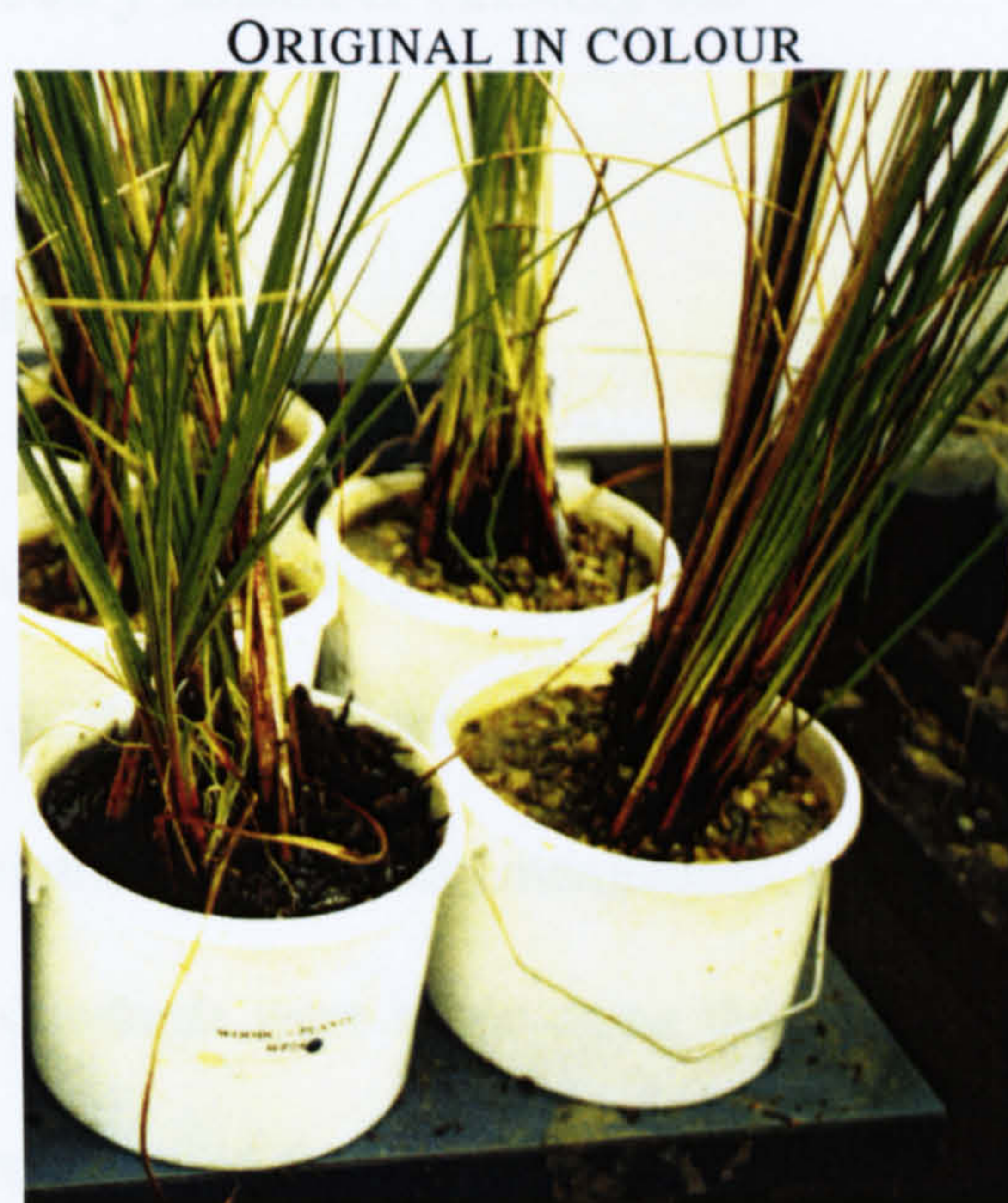
Figure 2.8: An example of planted microcosm set up, treating mine drainage water.
