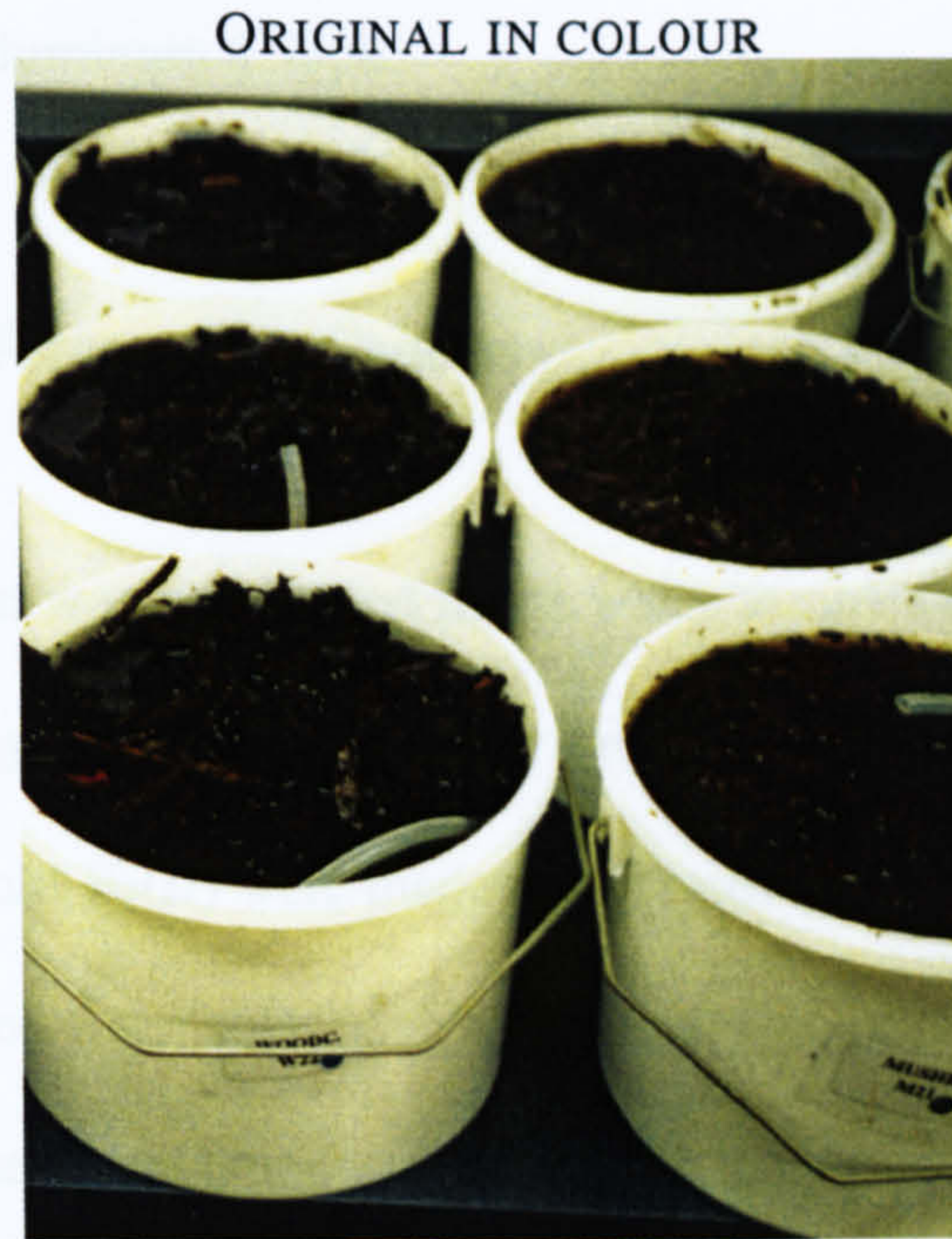
Figure 2.9: An example of unplanted microcosm treating mine drainage water.
