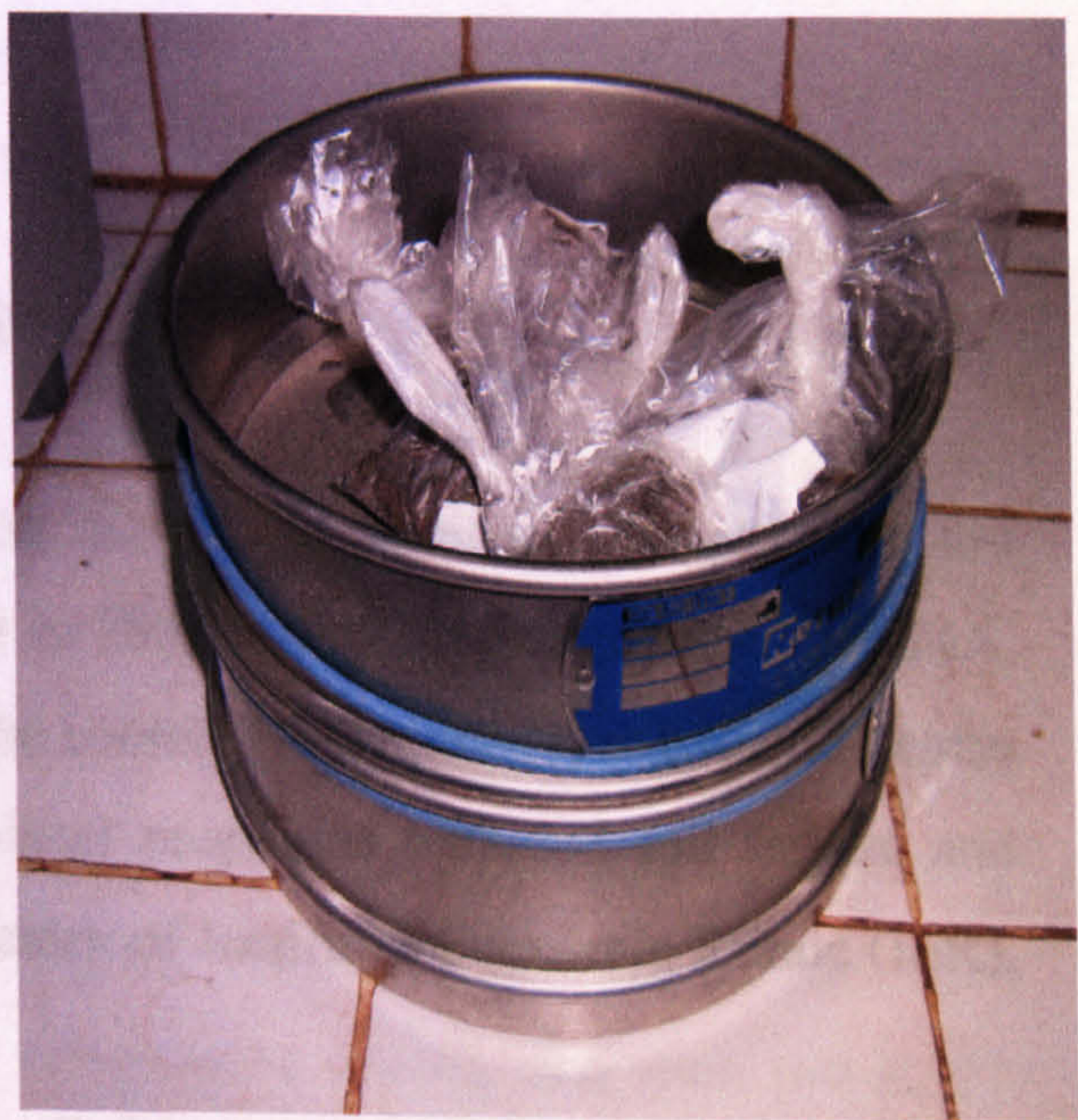
b) Sieves of different size used for washing roots
