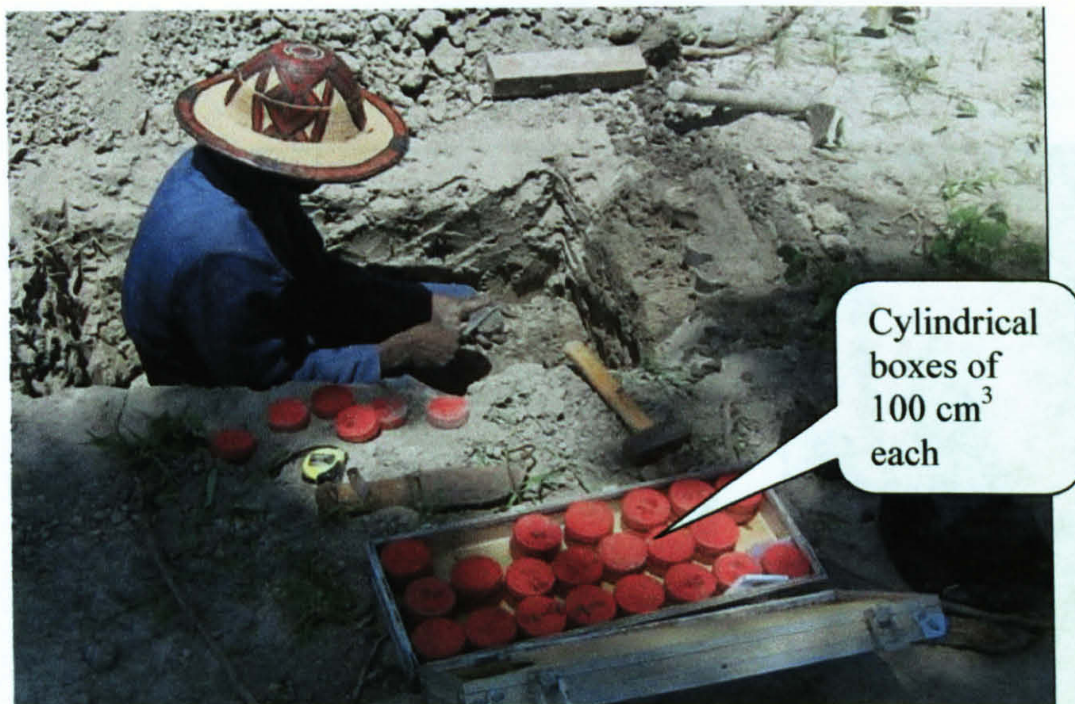
Plate 4.4: Bulk density works showing the pit for soil sampling
