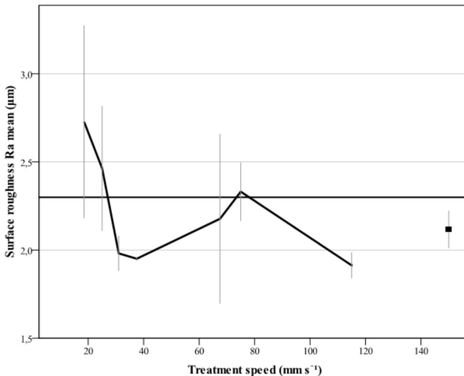
**Figure 4.30: Hot treatment surface roughness mean ( $\mu\text{m}$ ).** The mean value at the  $150\text{ mm s}^{-1}$  treatment speed refers to the samples treated twice with the speed of  $75\text{ mm s}^{-1}$ . The flat line represent the control mean ( $2.3\text{ }\mu\text{m}$ ). Error bars represent the SD ( $\pm 1$ ).
