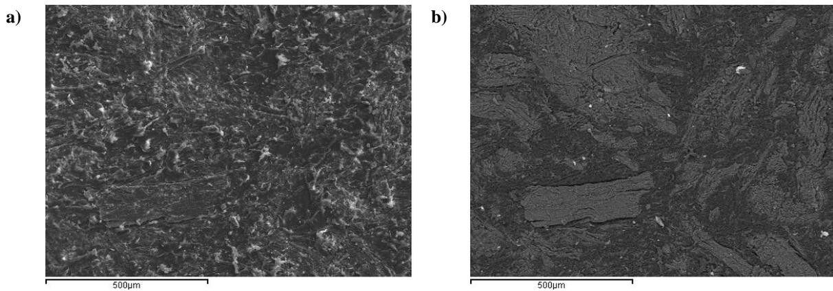
**Figure 4.12: pH 9 solution treated sample under X134 magnification (X100 equipment indication). a) photo is showing the surface under SEM backscattered electron image. b) shows a secondary electron image of the same region.**
