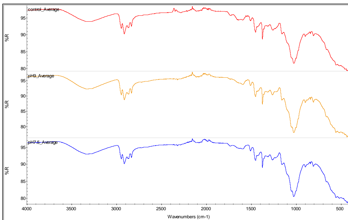
Figure 4.28: FTIR-ATR spectra of untreated samples and treated in pH 7.5 and pH 9 solution
