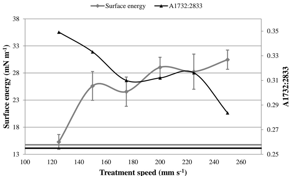
**Figure 5.18: Ester ratio ( $A_{1732:2833}$ ) compared to surface energy of the samples treated with flame. The linear lines present the surface energy (gray line) and the ester ratio (black line) control values. Error bars represent the SD (+/-).**
