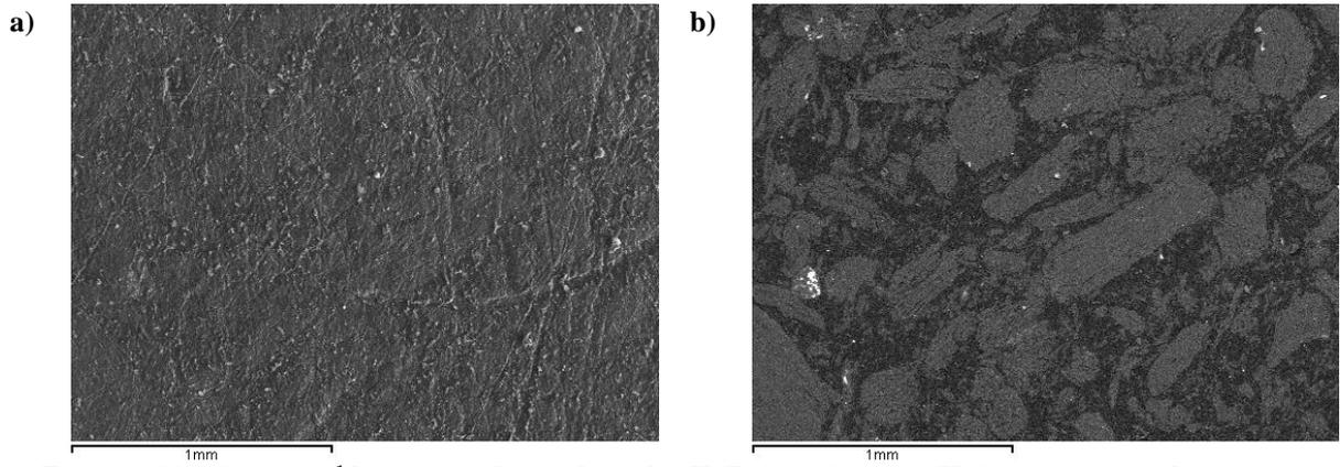
**Figure 4.31:  $18.5 \text{ mm s}^{-1}$  heat treated sample under X67 magnification (X50 equipment indication). a) Backscattered image of the surface. b) same region seen as a secondary electron image.**
