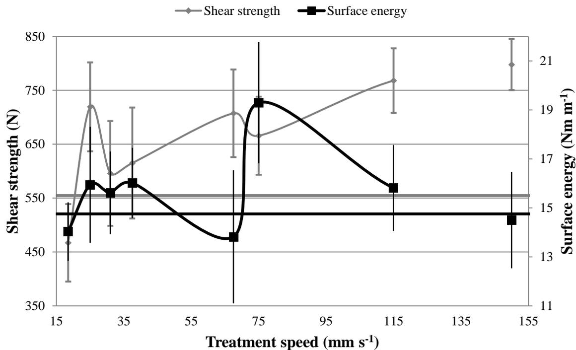
**Figure 5.12: Adhesion strength compared to surface energy of hot air treated samples. The values at the treatment speed of 150mm s<sup>-1</sup> are referring to the treatment with 2 times pass of the hot air gun with the speed of 75 mm s<sup>-1</sup>. The linear lines present the shear strength (gray line) and the surface energy (black line) control values. Error bars represent the SD (+/-1).**
