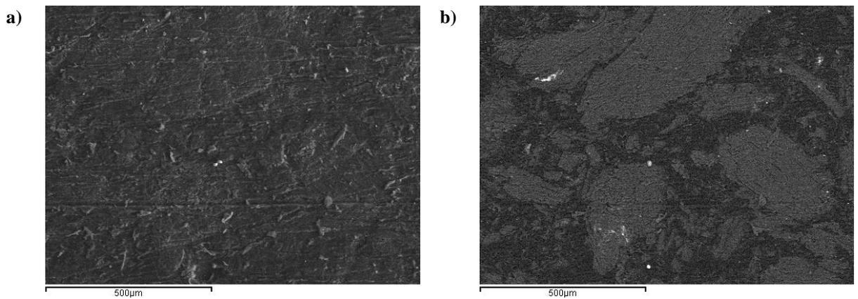
**Figure 4.52:** 30 mm s<sup>-1</sup> halogen heating lamps treated sample under X134 magnification (X100 equipment indication). a) Backscattered image of the surface. b) same region seen as a secondary electron image.
