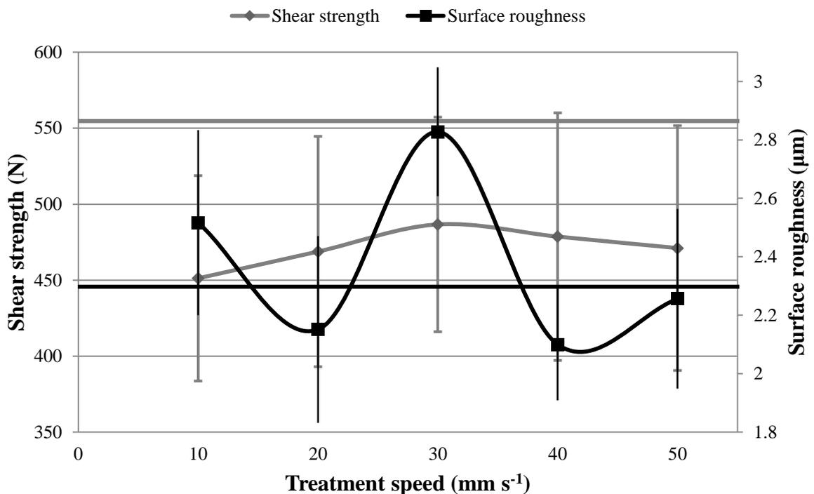
**Figure 5.4: Halogen heating lamp treatment shear strength and surface roughness chart. The linear lines present the shear strength (gray line) and the surface roughness (black line) control values. Error bars represent the SD (+/-).**
