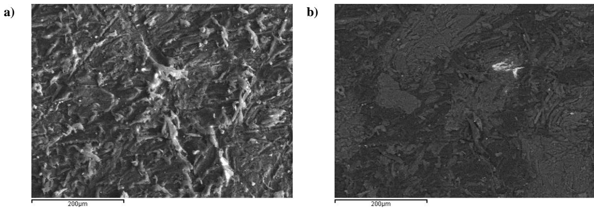
**Figure 4.34:**  $2 \times 75 \text{ mm s}^{-1}$  heat treated sample under X265 magnification (X100 equipment indication). a) Backscattered image of the surface. b) same region seen as a secondary electron image.
