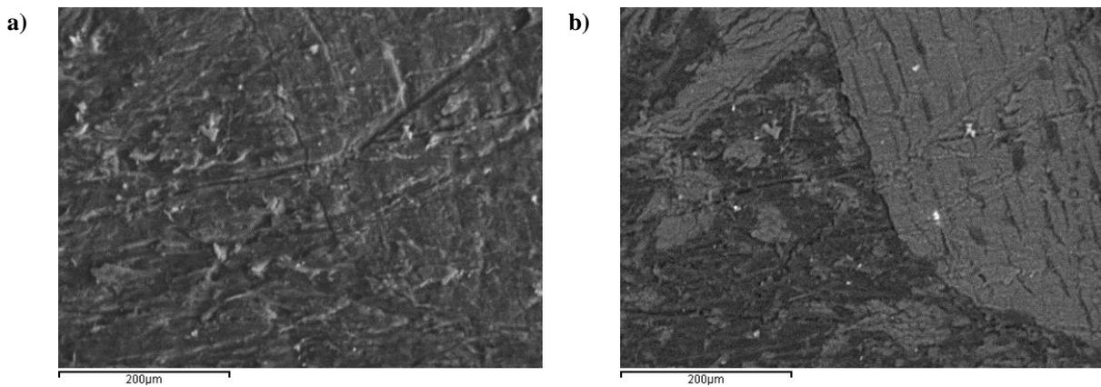
**Figure 4.50:  $10 \text{ mm s}^{-1}$  halogen heating lamps treated sample under X265 magnification (X200 equipment indication). a) Backscattered image of the surface. b) same region seen as a secondary electron image.**
