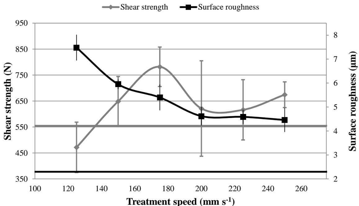
**Figure 5.3: Flame treatment shear strength and surface roughness chart. The linear lines present the shear strength (gray line) and the surface roughness (black line) control values. Error bars represent the SD (+/-).**
