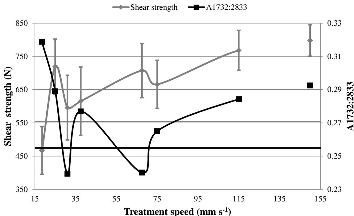
**Figure 5.13: Adhesion strength and ester ratio ( $A_{1732:2833}$ ) comparison of hot air treated samples. The values at the treatment speed of  $150\text{mm s}^{-1}$  are referring to the treatment with 2 times pass of the hot air gun with the speed of  $75\text{mm s}^{-1}$ . The linear lines present the shear strength (gray line) and the ester ratio (black line) control values. Error bars represent the SD (+/-1).**
