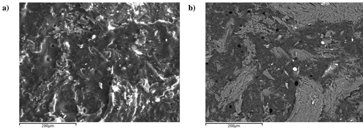
**Figure 4.43: 175 mm s<sup>-1</sup> flame treated sample under X265 magnification (X200 equipment indication). a) Backscattered image of the surface. b) same region seen as a secondary electron image.**
