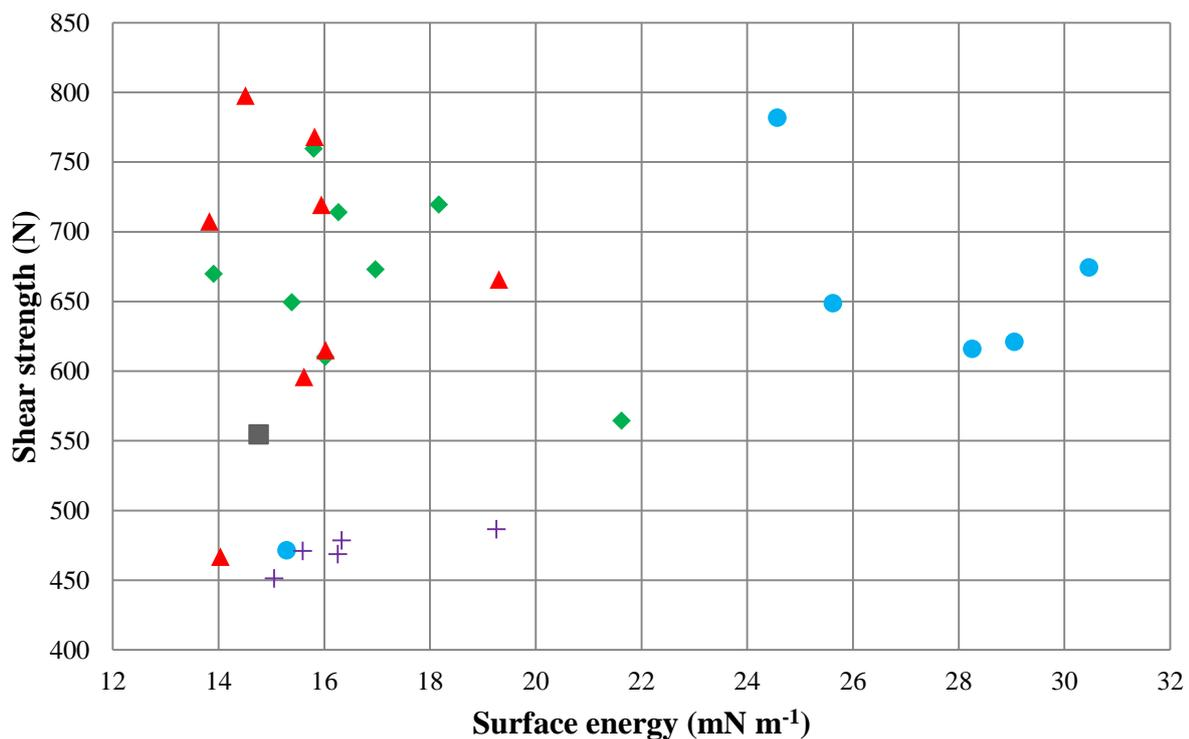
Figure 5.24: Adhesion strength and surface energy scatter graph of all the tested samples. Grey colour (■) Control, blue (●) flame treatment, red (▲) hot air gun treatment, green (◆) hydrogen peroxide treatment and purple (+) halogen heating lamps treatment.
