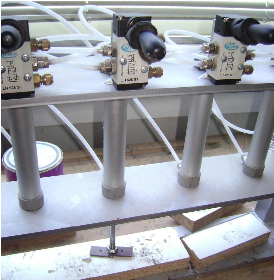
**Figure 3.9: Pneumatic clamps applying uniform pressure to a lap joint specimen.**
