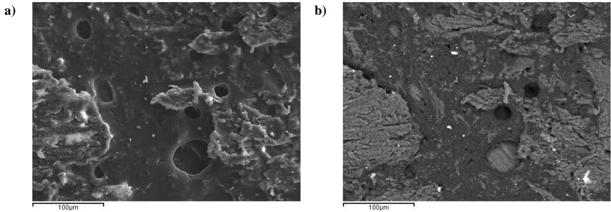
**Figure 4.41: 125 mm s<sup>-1</sup> flame treated sample under X400 magnification (X300 equipment indication). a) Backscattered image of the surface. b) same region seen as a secondary electron image.**
