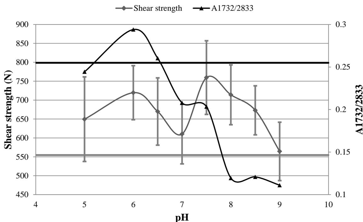
**Figure 5.7: Shear strength and ester ratio (A<sub>1732/2833</sub>) comparison of hydrogen peroxide treated samples. The linear lines present the shear strength (gray line) and the ester ratio (black line) control values. Error bars represent the SD (+/-1).**
