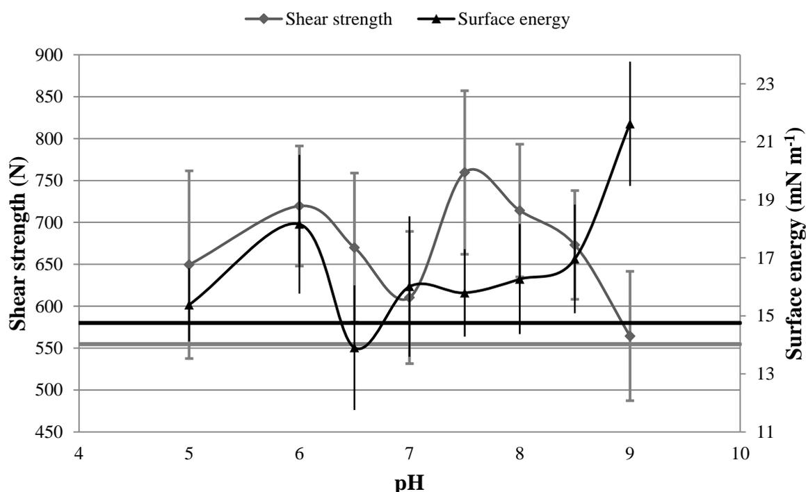
**Figure 5.6: Adhesion strength compared to surface energy of hydrogen peroxide treated samples. The linear lines present the shear strength (gray line) and the surface energy (black line) control values. Error bars represent the SD (+/-1).**
