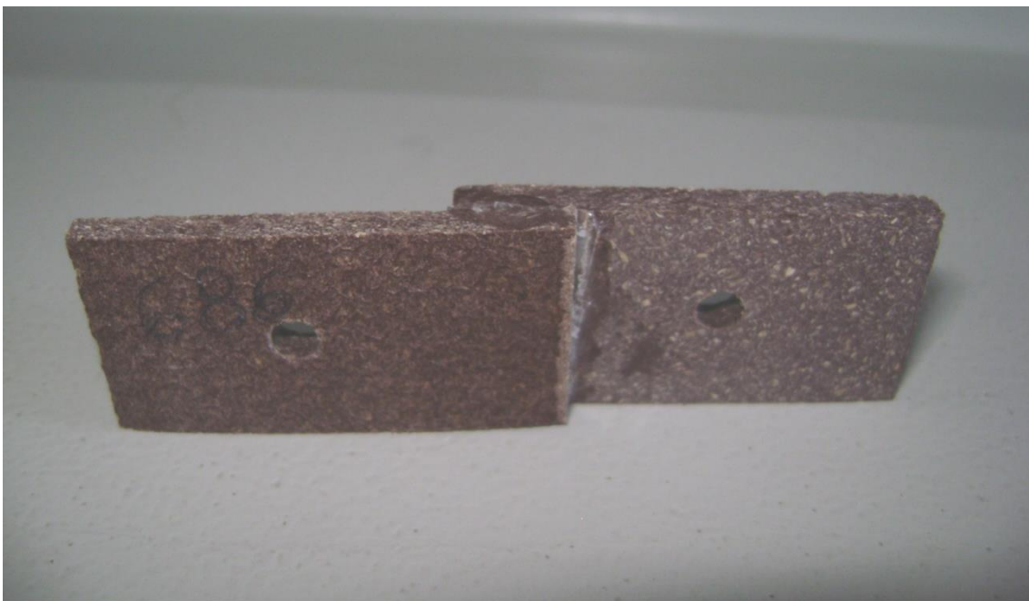
Figure 3.10: Lap joint with bonded area 10 X 20 mm, and holes to allow mounting in test machine.
