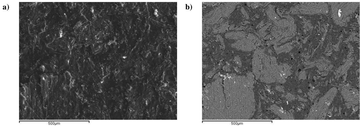
**Figure 4.42: 175 mm s<sup>-1</sup> flame treated sample under X134 magnification (X100 equipment indication). a) Backscattered image of the surface. b) same region seen as a secondary electron image.**
