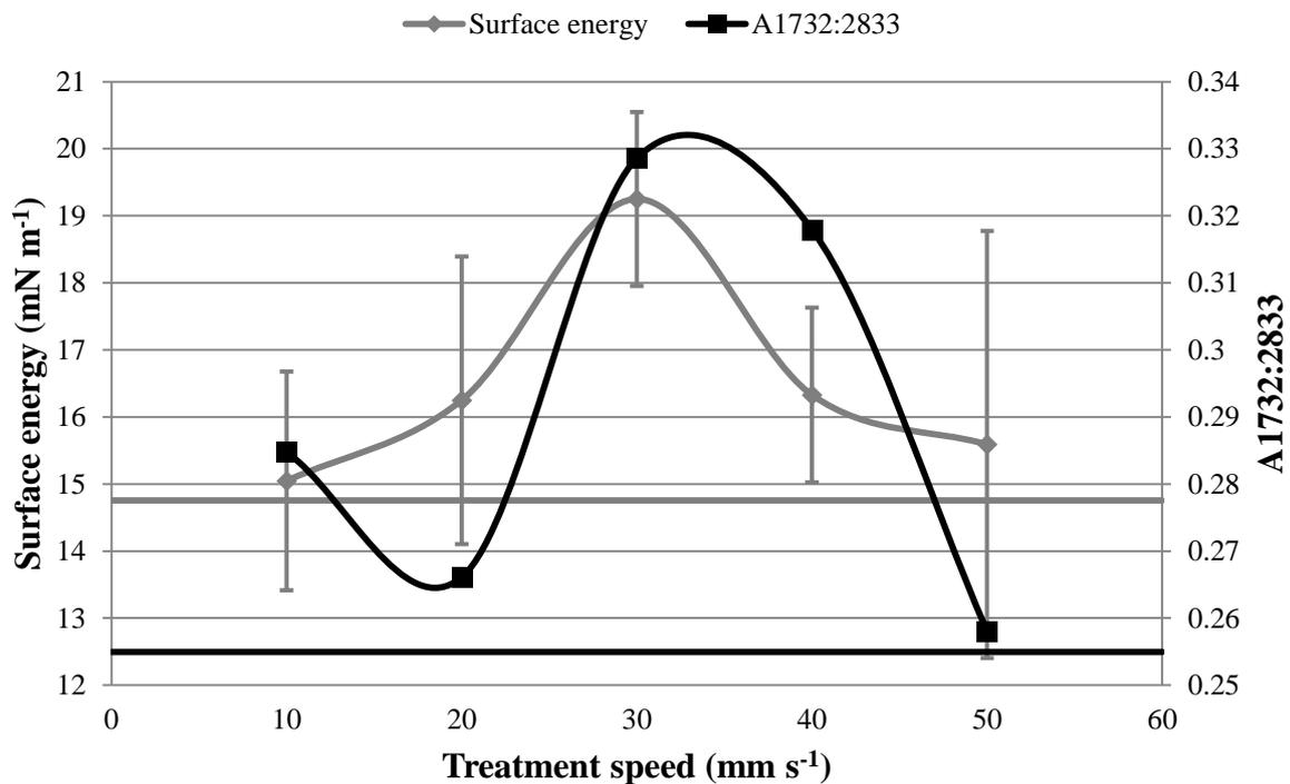
**Figure 5.22: Ester ratio ( $A_{1732:2833}$ ) compared to surface energy of the samples treated with halogen heating lamps. The linear lines present the surface energy (gray line) and the ester ratio (black line) control values. Error bars represent the SD (+/-1).**
