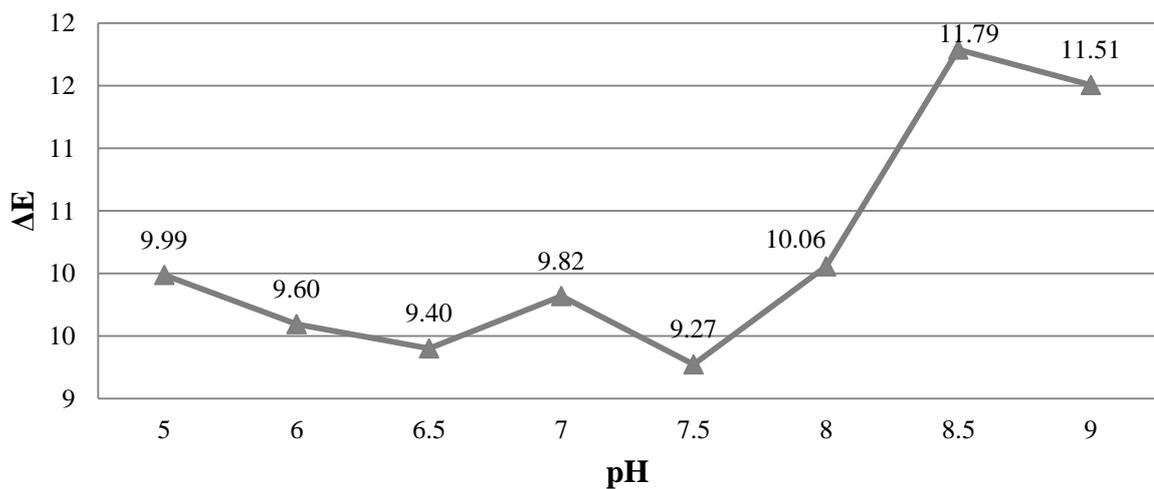
**Figure 4.65: Hydrogen peroxide treatment colour changes  $\Delta E$ .**
