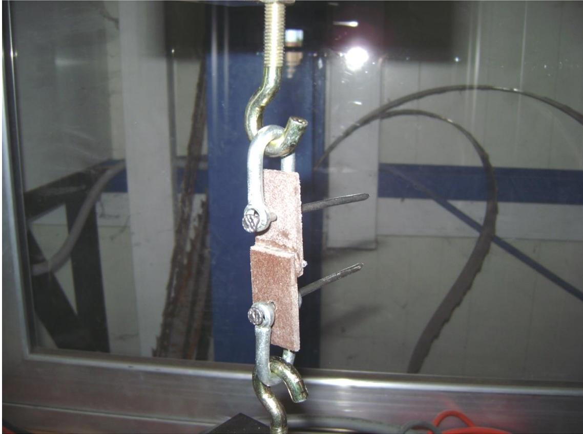
**Figure 3.12: Samples attached on the mechanical properties instrument.**
