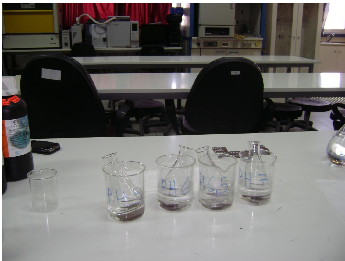
Figure 3.6: Samples placed into the hydrogen peroxide solution.
