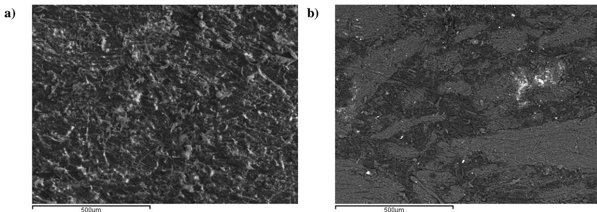
**Figure 4.6: Control sample under X134 magnification (X100 equipment indication). a) photo is showing the surface under SEM primary electron scanning. b) photo shows control sample under secondary electron scanning. The photos are from the same region.**
