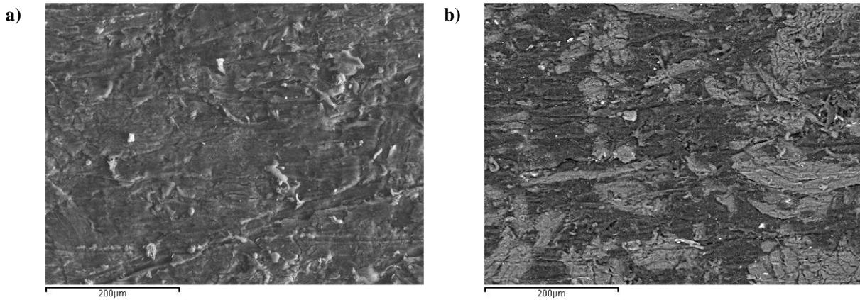
**Figure 4.53: 30 mm s<sup>-1</sup> halogen heating lamps treated sample under X265 magnification (X200 equipment indication). a) Backscattered image of the surface. b) same region seen as a secondary electron image.**
