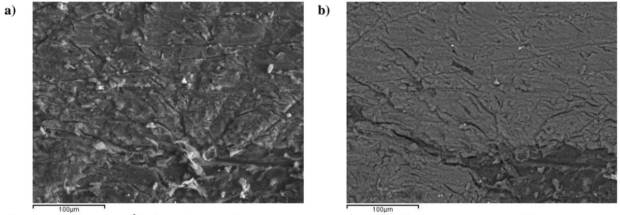
**Figure 4.51:** 10 mm s<sup>-1</sup> halogen heating lamps treated sample under X400 magnification (X300 equipment indication). a) Backscattered image of the surface. b) same region seen as a secondary electron image.
