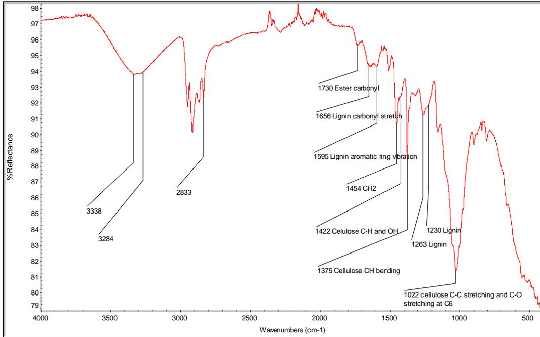
Figure 4.9: Average spectrum for untreated WPC sample, with labels showing the peaks investigated and reference peak at 2833 cm<sup>-1</sup>.
