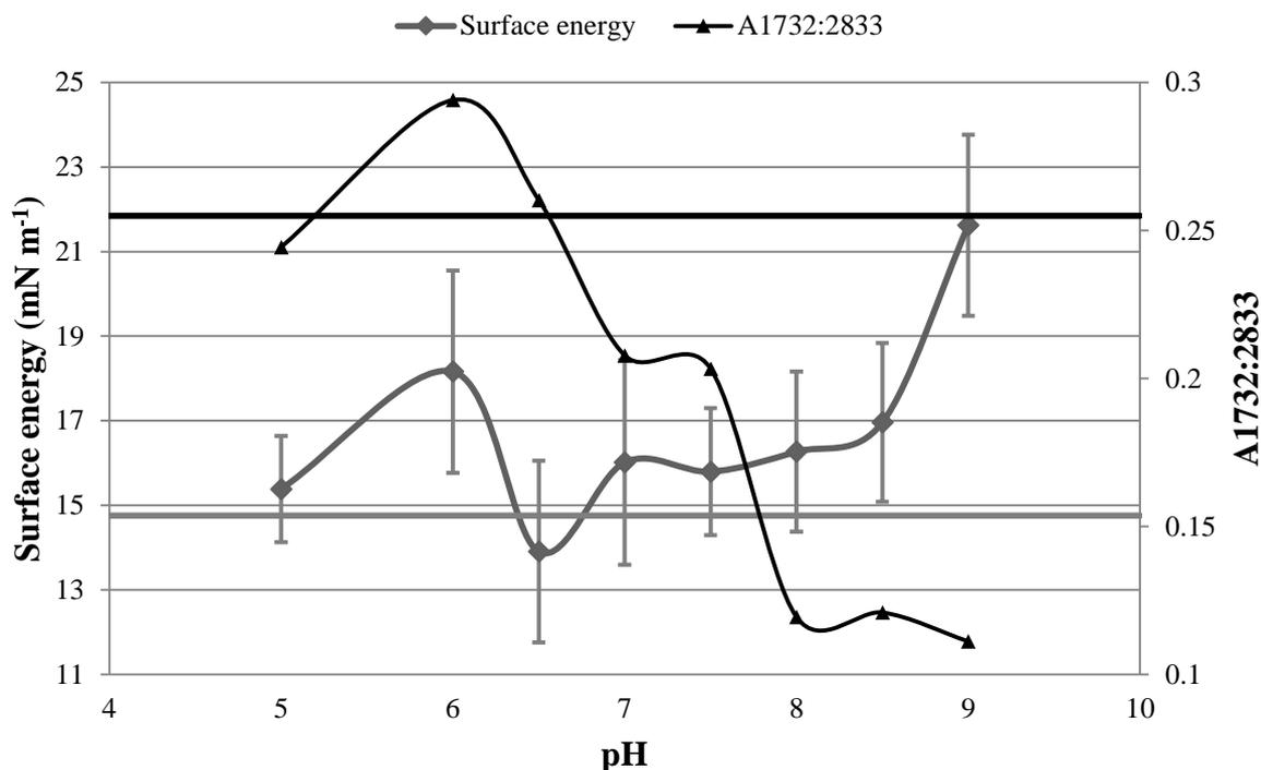
**Figure 5.10: Ester ratio ( $A_{1732/2833}$ ) compared to surface energy of the samples treated in hydrogen peroxide solutions. The linear lines present the surface energy (gray line) and the ester ratio (black line) control values. Error bars represent the SD (+/-1).**
