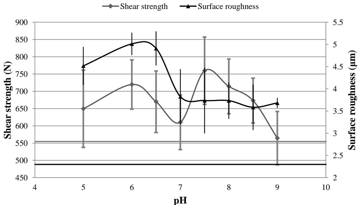
**Figure 5.1: Hydrogen peroxide treatment shear strength and surface roughness chart. The linear lines present the shear strength (gray line) and the surface roughness (black line) control values. Error bars represent the SD (+/-1).**
