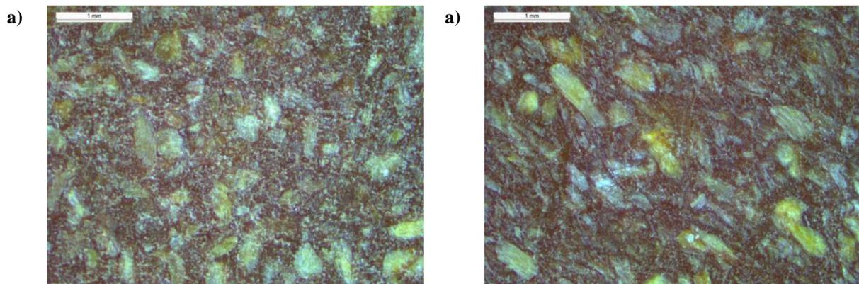
**Figure 4.75:** Light microscopy (X2.5 equipment indication). a) Sample treated with halogen heating lamps at  $10 \text{ mm s}^{-1}$ . b) Sample treated with halogen heating lamps at  $30 \text{ mm s}^{-1}$ .
