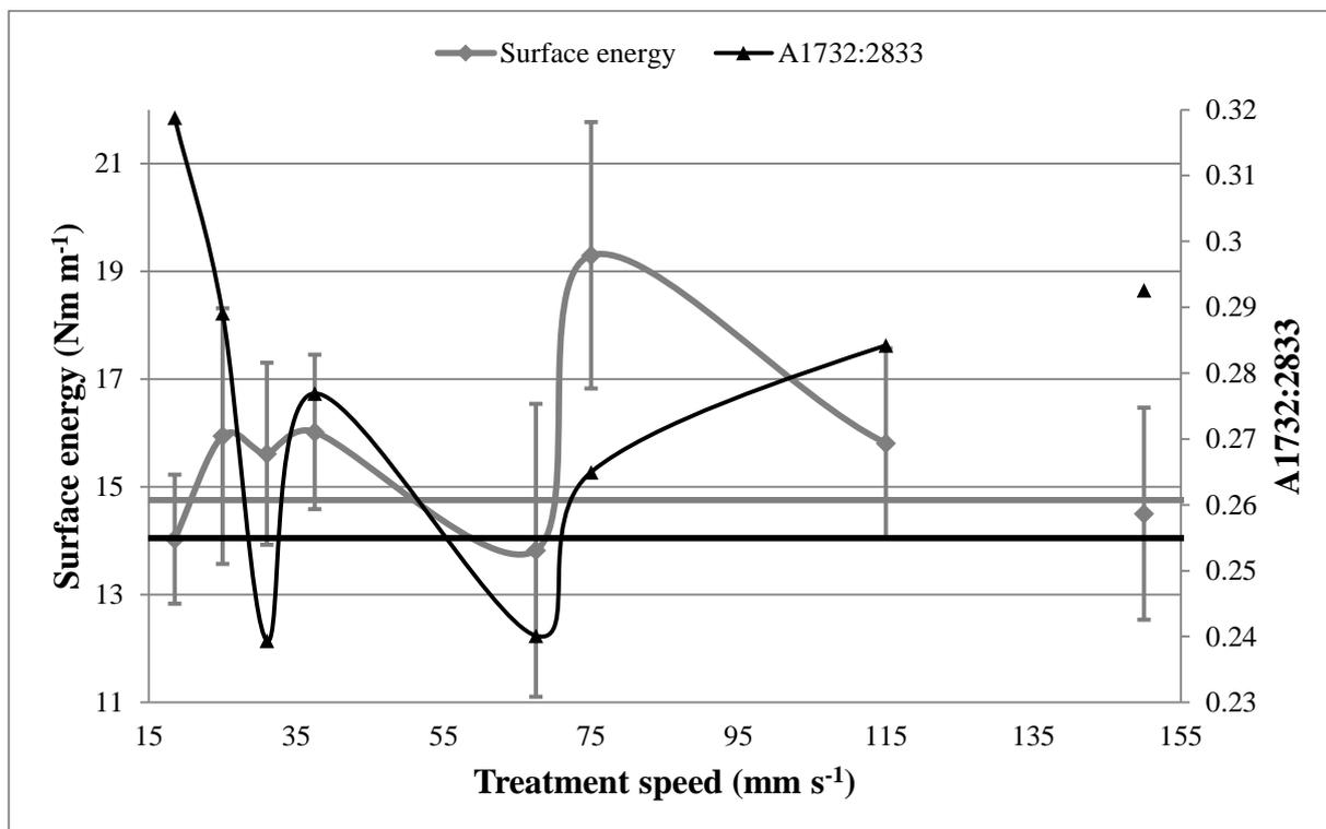
**Figure 5.14: Ester ratio ( $A_{1732:2833}$ ) compared to surface energy of the samples treated with hot air. The values at the treatment speed of  $150\text{mm s}^{-1}$  are referring to the treatment with 2 times pass of the hot air gun with the speed of  $75\text{mm s}^{-1}$ . The linear lines present the surface energy (gray line) and the ester ratio (black line) control values. Error bars represent the SD (+/-).**
