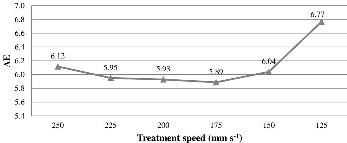
Figure 4.73: Flame treatment colour changes  $\Delta E$ .
