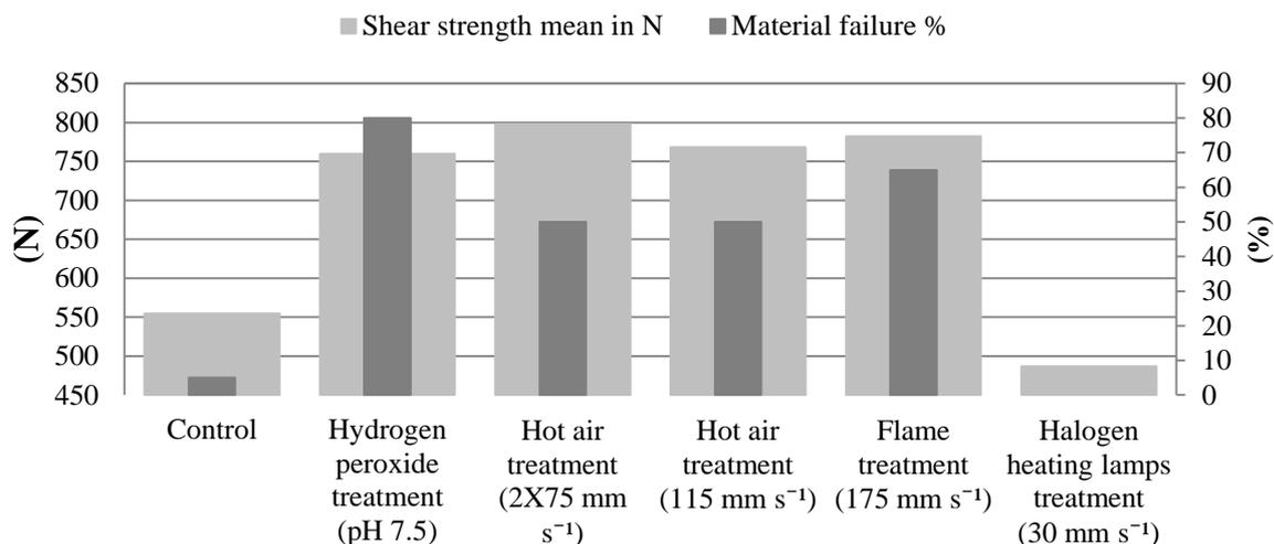
**Figure 5.27: Treatments methods shear strength means and material failure percentage. Light grey bars are showing the highest shear strength mean observed of every treatment. Darker bars are showing the percentage of the samples that failed at the material rather to the bonding.**
