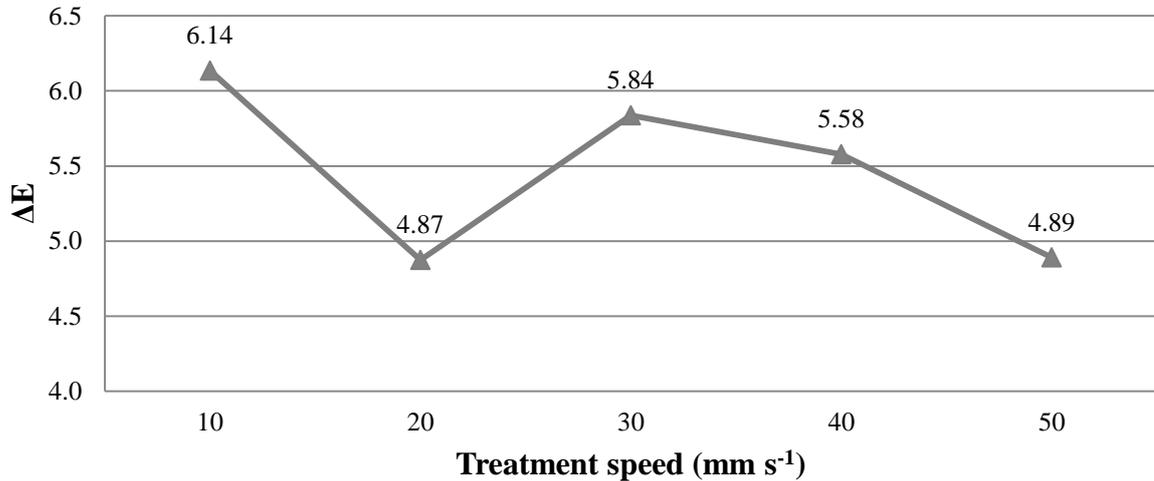
Figure 4.77: Halogen heating lamps treatment colour changes  $\Delta E$ .
