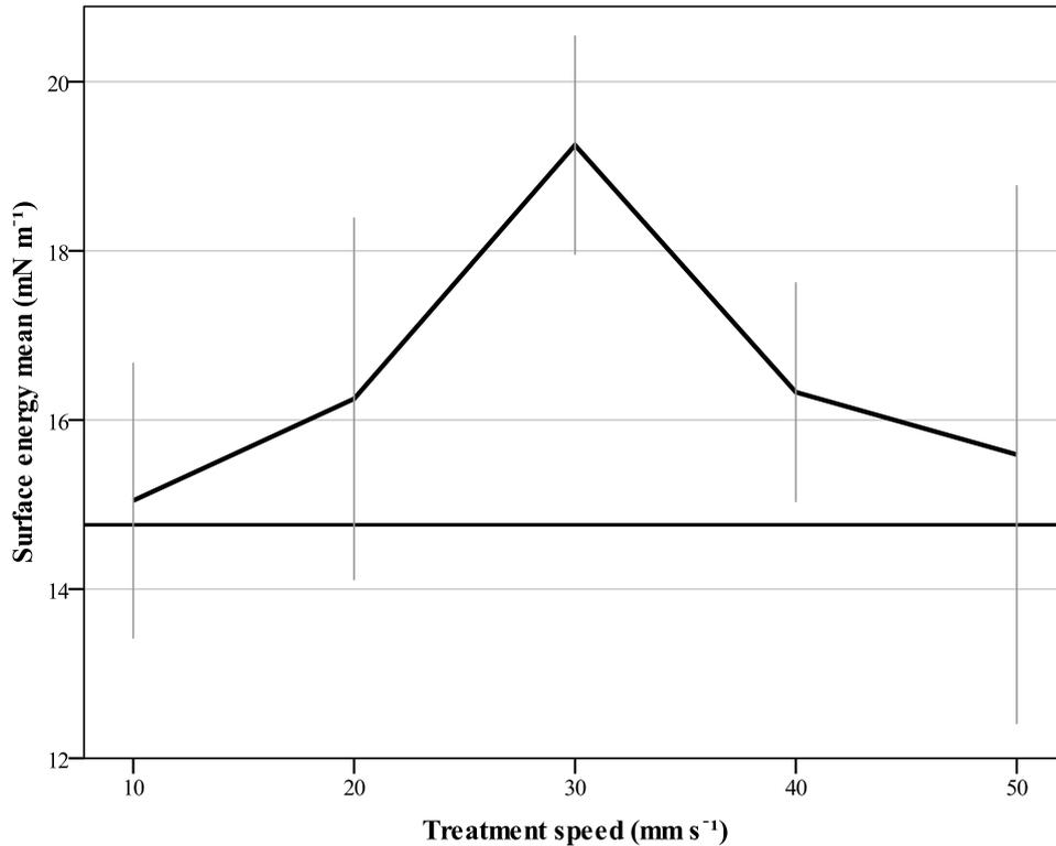
**Figure 4.55: Halogen heating lamp treatment surface energy (mN m<sup>-1</sup>). The flat line represents the control mean (14.76 mN m<sup>-1</sup>). Error bars represent the SD (+/-).**
