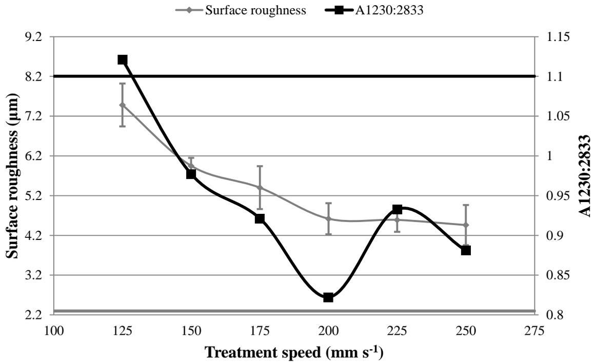
**Figure 5.19: Lignin ratio ( $A_{1230:2833}$ ) compared to surface roughness of the samples treated with flame. The linear lines present the surface roughness (gray line) and the  $A_{1230:2833}$  (black line) control values. Error bars represent the SD (+/-1).**
