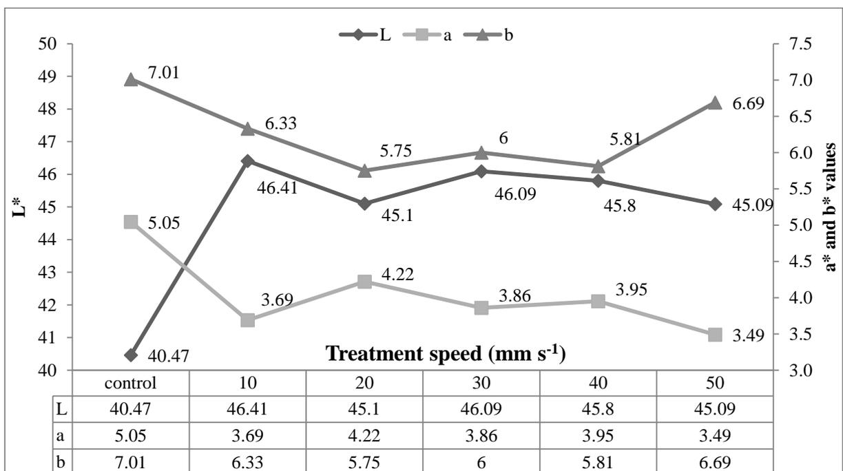
Figure 4.78: Halogen heating lamps treatment colour determination values. "a" refers to red for positive values and green for negative. "b" refers to yellow for positive values and blue for negative. "L" refers to white for 100 value and black as the value decreasing to 0.
