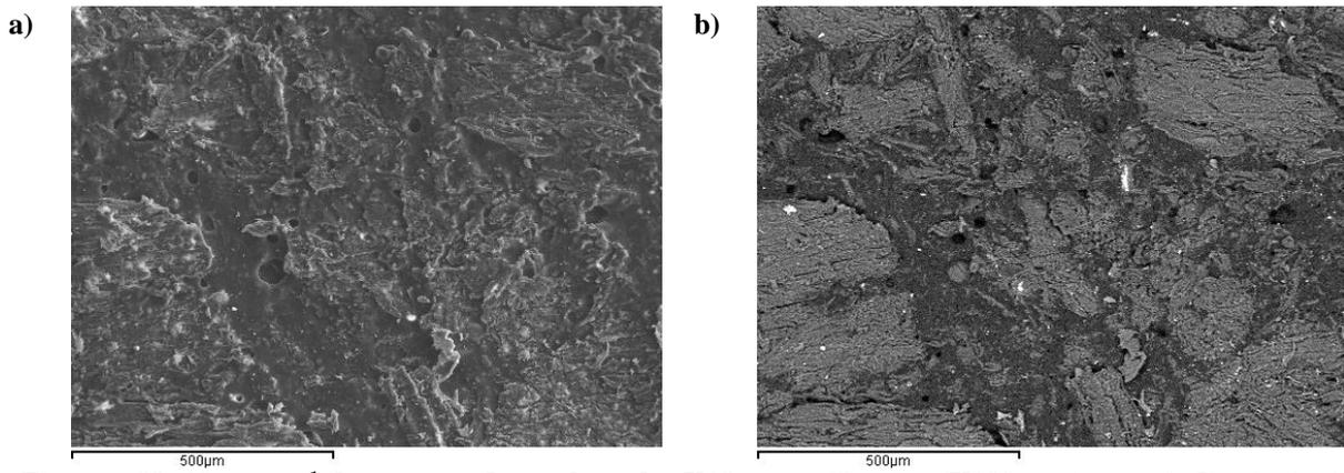
**Figure 4.39:** 125 mm s<sup>-1</sup> flame treated sample under X134 magnification (X100 equipment indication). a) Backscattered image of the surface. b) same region seen as a secondary electron image.
