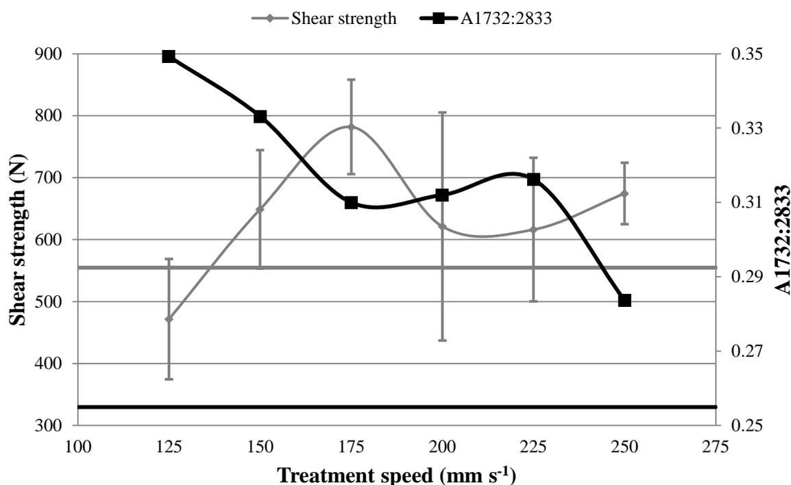
**Figure 5.17: Shear strength and ester ratio ( $A_{1732:2833}$ ) comparison of flame treated samples. The linear lines present the shear strength (gray line) and the ester ratio (black line) control values. Error bars represent the SD (+/-1).**
