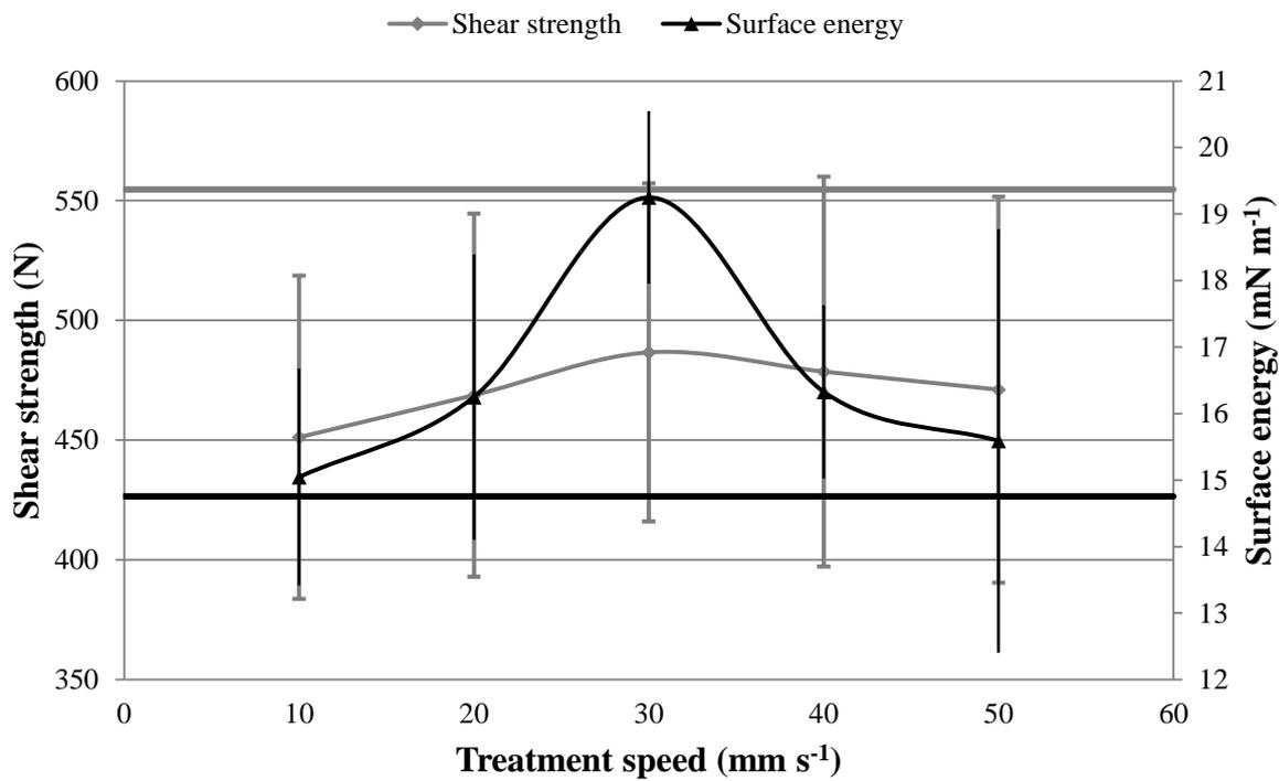
**Figure 5.20: Adhesion strength compared to surface energy of halogen heating lamp treated samples. The linear lines present the shear strength (gray line) and the surface energy (black line) control values. Error bars represent the SD (+/-1).**
