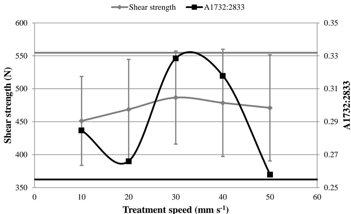
**Figure 5.21: Shear strength and ester ratio ( $A_{1732:2833}$ ) comparison of halogen heating lamps treated samples. The linear lines present the shear strength (gray line) and the ester ratio (black line) control values. Error bars represent the SD (+/-1).**
