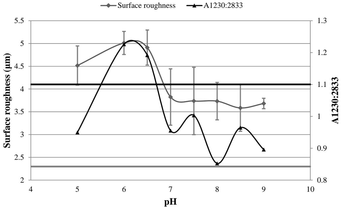
**Figure 5.11: Lignin ratio ( $A_{1230:2833}$ ) compared to surface roughness of the samples treated in hydrogen peroxide solutions. The linear lines present the surface roughness (gray line) and the  $A_{1230:2833}$  (black line) control values. Error bars represent the SD (+/-1).**
