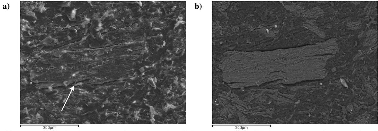
**Figure 4.13: pH 9 solution treated sample under X265 magnification (X200 equipment indication), detail of Figure 4.19. a) Backscattered image of the surface. b) same region seen as a secondary electron image. The arrow in photo a) shows the separation of wood fibre and from PP**
