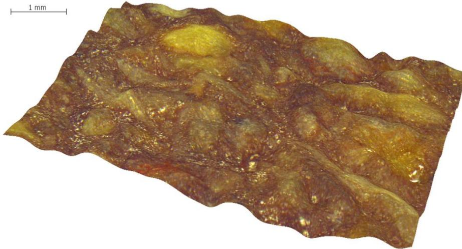
**Figure 4.72: 3D model of flame treated sample at 125 mm s<sup>-1</sup>.**
