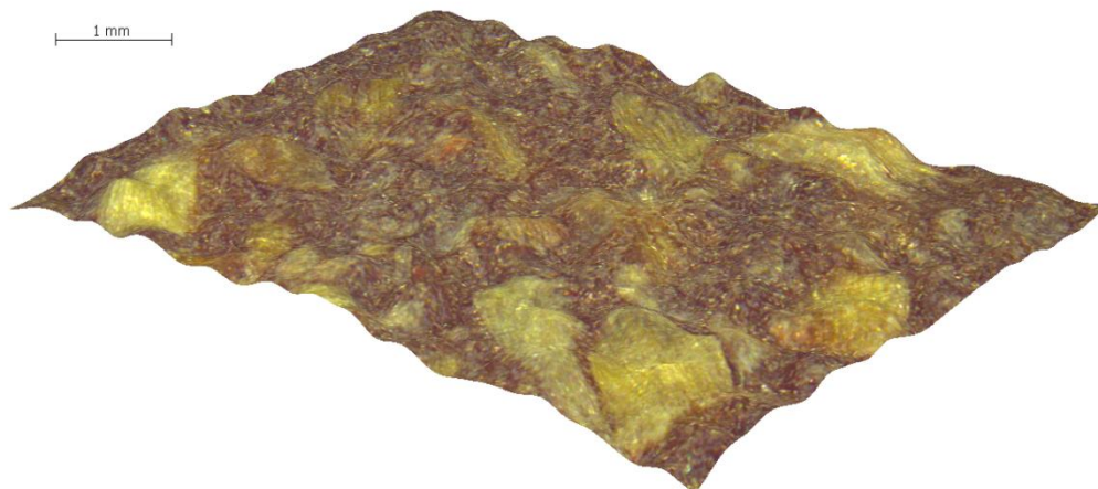
Figure 4.76: 3D model of halogen heating lamps treated sample with the speed of 10 \text{ mm s}^{-1} .
