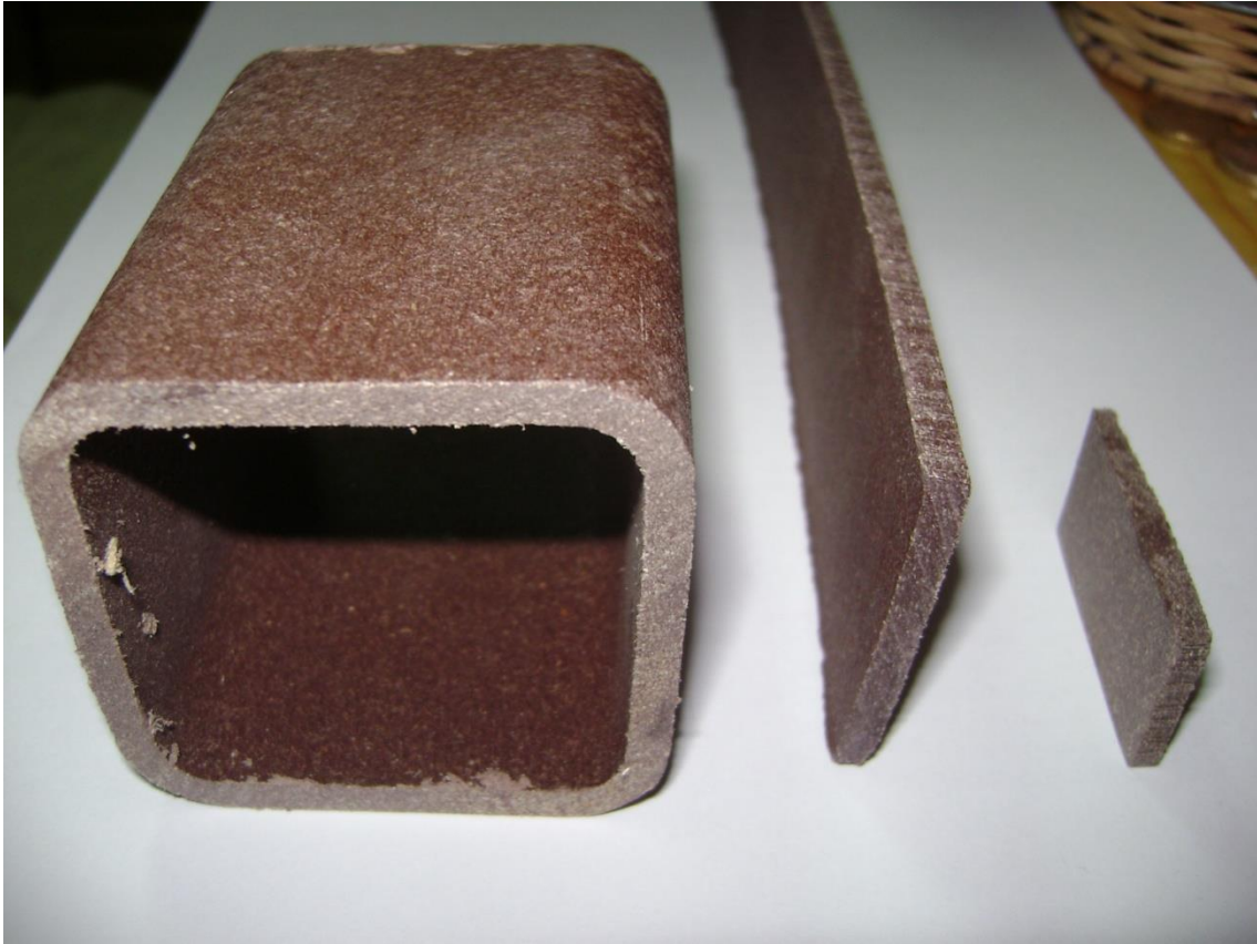
Figure 3.1: WPC pipe sliced to prepare flat strips sample.
