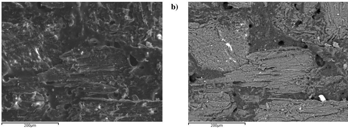
**Figure 4.40:** 125 mm s<sup>-1</sup> flame treated sample under X265 magnification (X200 equipment indication). a) Backscattered image of the surface. b) same region seen as a secondary electron image.
