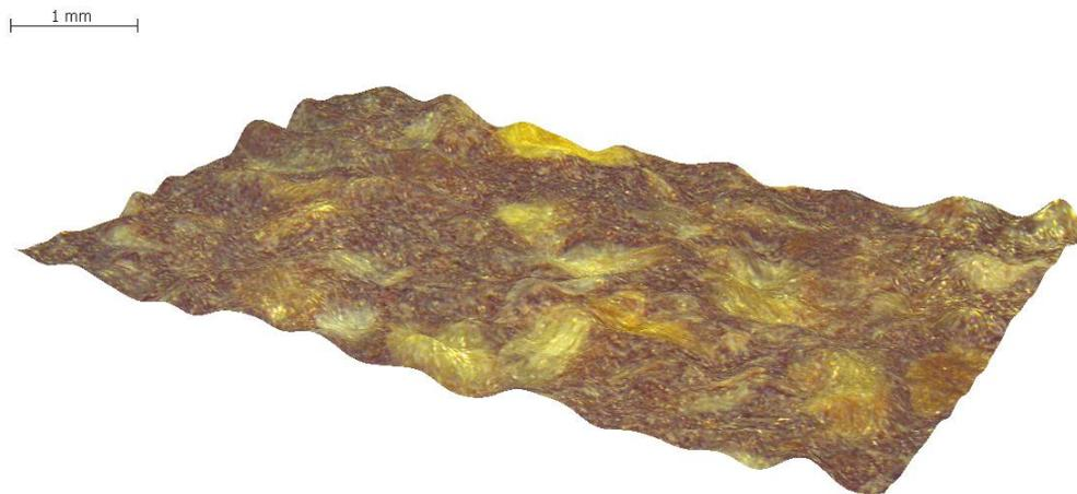
Figure 4.68: 3D model of hot air treated sample with 2 passes at 75 mm s<sup>-1</sup>.
