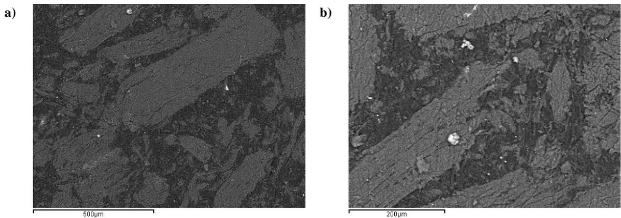
**Figure 4.32: Secondary electron image of  $18.5 \text{ mm s}^{-1}$  heat treated sample under X134 magnification (X100 equipment indication) a) and under X265 magnification (X200 equipment indication) b).**
