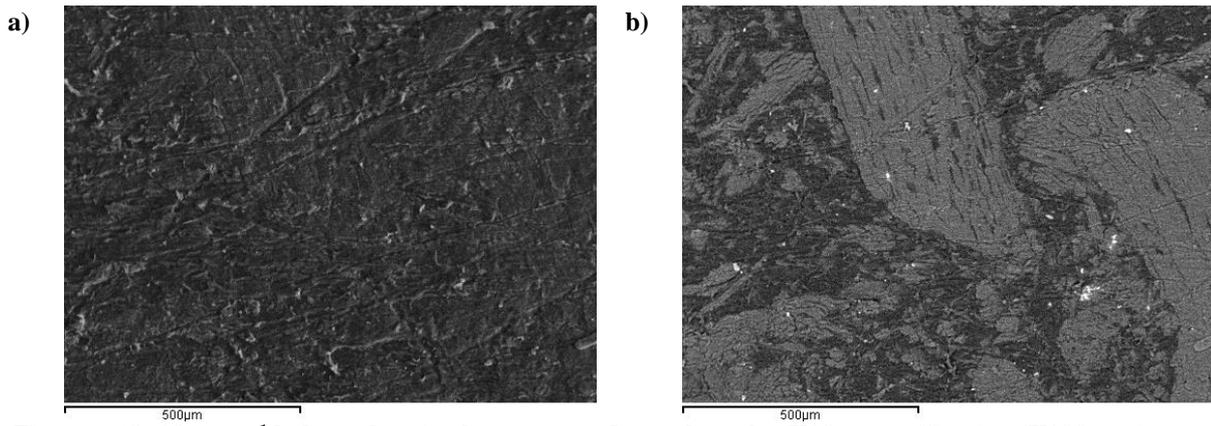
**Figure 4.49:  $10 \text{ mm s}^{-1}$  halogen heating lamps treated sample under X134 magnification (X100 equipment indication). a) Backscattered image of the surface. b) same region seen as a secondary electron image.**
