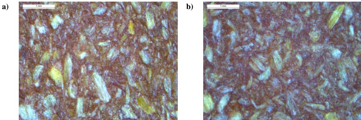
**Figure 4.71: Light microscopy (X2.5 equipment indication). a) Flame treated sample with the speed of 125 mm s<sup>-1</sup>. b) Flame treated sample at 250 mm s<sup>-1</sup>.**
