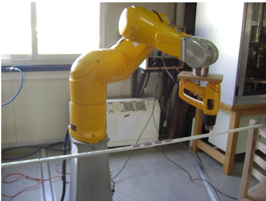
Figure 3.7: Hot air treatment.
