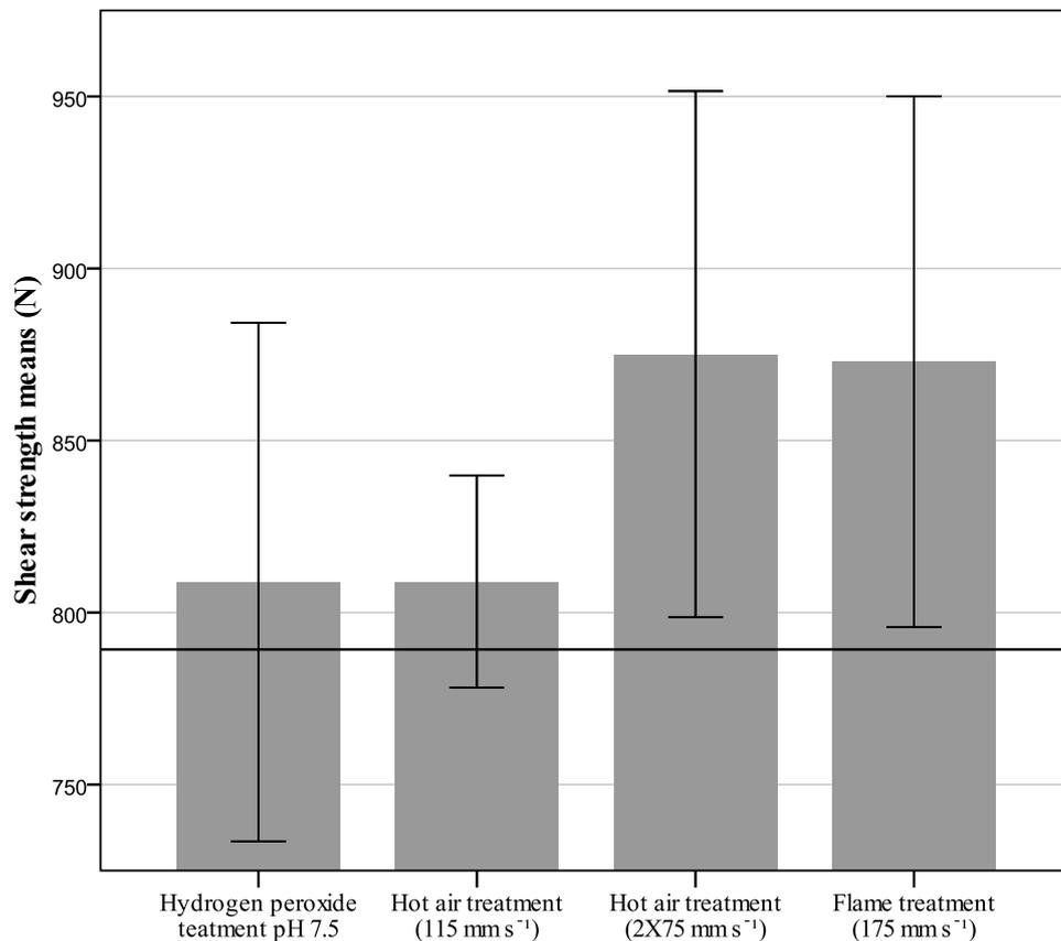
**Figure 5.28: Mean values of the samples failed on the material rather the bonding line. The linear line present the shear strength of the only control sample which failed in the material (789.26 N). Error bars presenting the SD (+/-1).**
