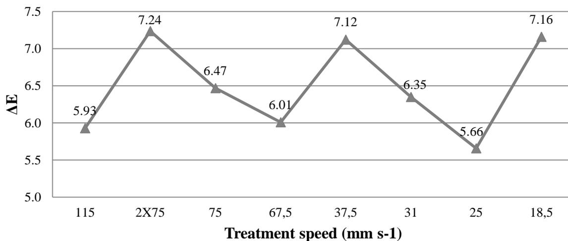
Figure 4.69: Hot air treatment colour changes  $\Delta E$ .
