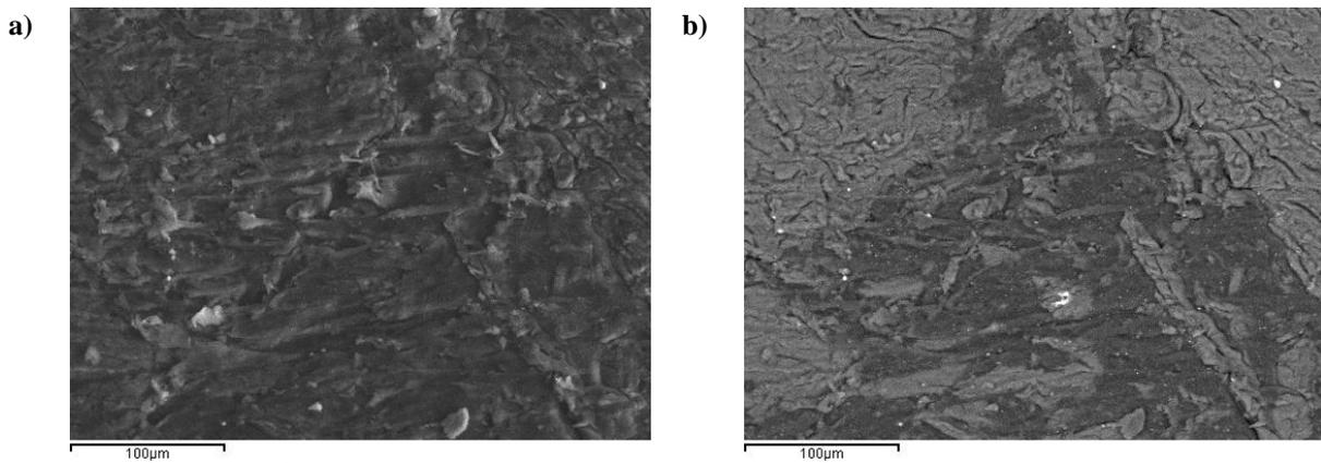
**Figure 4.54: 30 mm s<sup>-1</sup> halogen heating lamps treated sample under X400 magnification (X300 equipment indication). a) Backscattered image of the surface. b) same region seen as a secondary electron image.**
