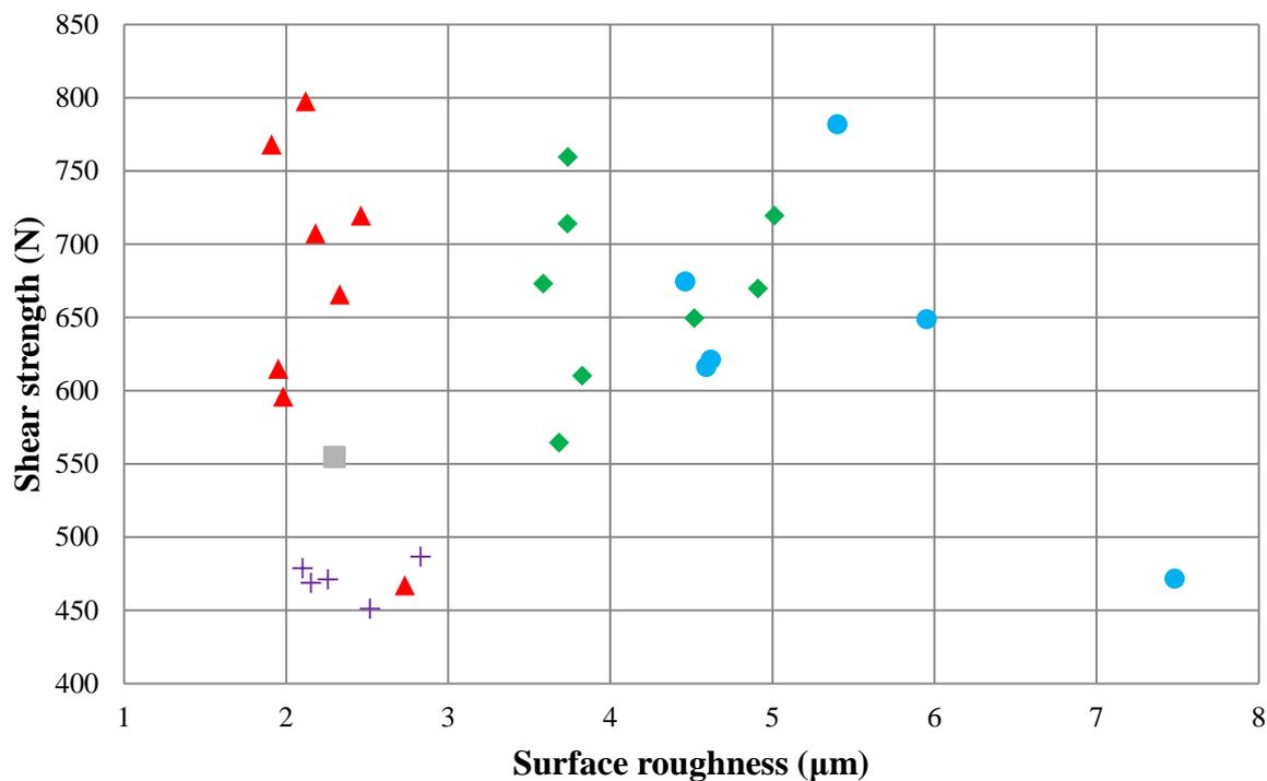
**Figure 5.5: Surface roughness and adhesion strength of all the treated and control samples. Grey colour (■) Control, blue (●) flame treatment, red (▲) hot air gun treatment, green (◆) hydrogen peroxide treatment and purple (+) halogen heating lamps treatment.**
