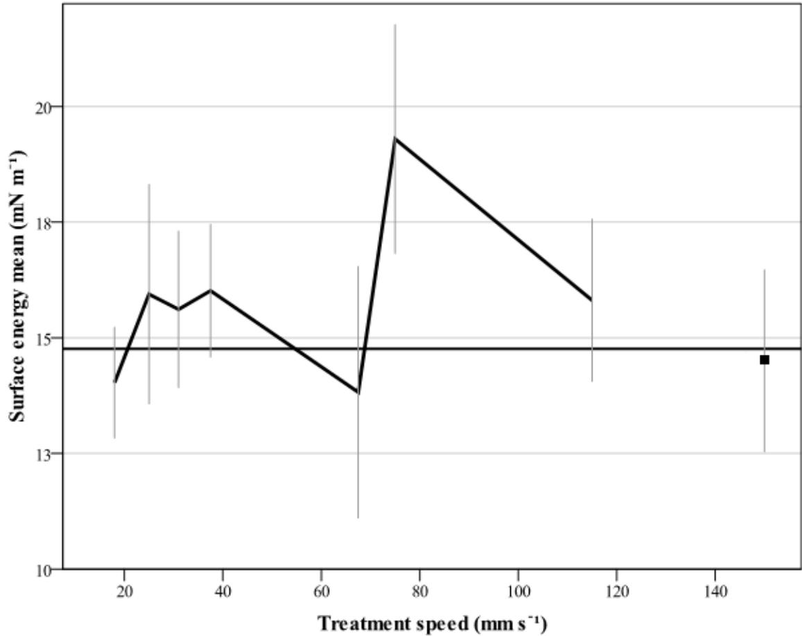
**Figure 4.35: Hot air treatment surface energy (mN m<sup>-1</sup>). The mean value at the 150 mm s<sup>-1</sup> treatment speed refers to the samples treated twice with the speed of 75 mm s<sup>-1</sup>. The flat line represent the control value (14.76 mN m<sup>-1</sup>). Error bars represent the SD (+/-).**
