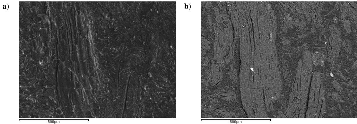
**Figure 4.11: pH 9 solution treated sample under X134 magnification (X100 equipment indication). a) photo is showing the surface under SEM backscattered electron image. b) photo shows a secondary electron image of the same region**
