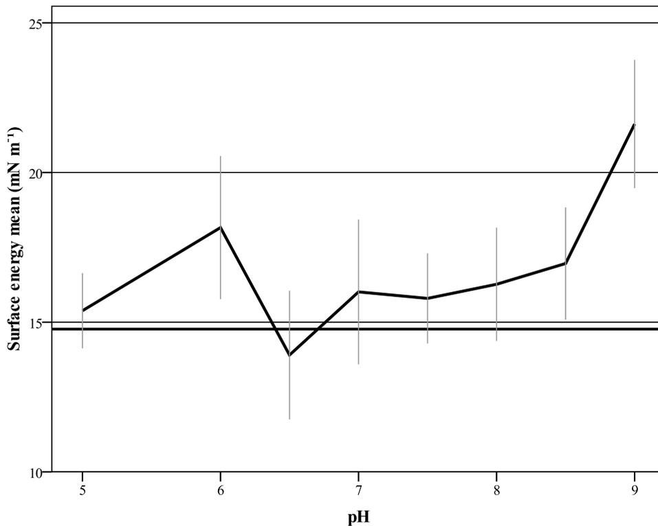
**Figure 4.27: Effect of pH and hydrogen peroxide treatment on surface energy ( $\text{mN m}^{-1}$ ). The flat line represent the control mean ( $14.76 \text{ mN m}^{-1}$ ). Error bars represent the SD ( $\pm 1$ ).**
