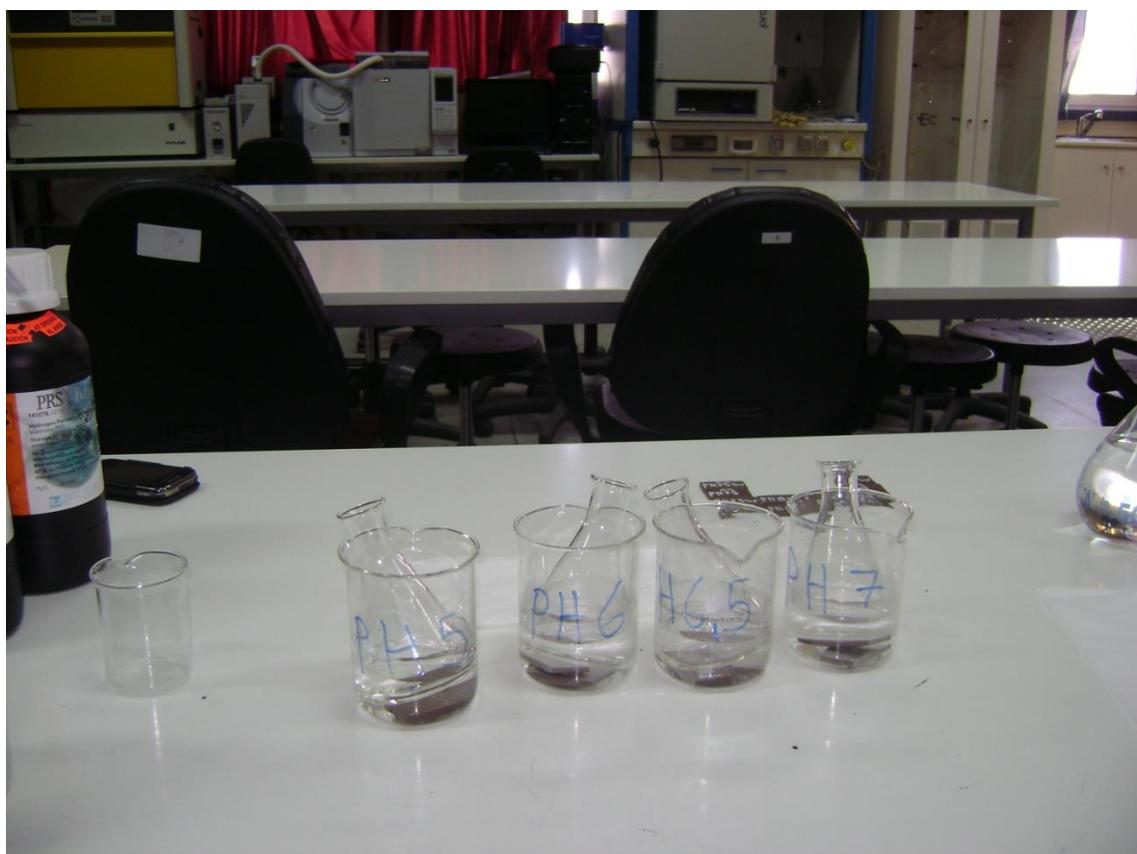
**Figure 3.6: Samples placed into the hydrogen peroxide solution.**
