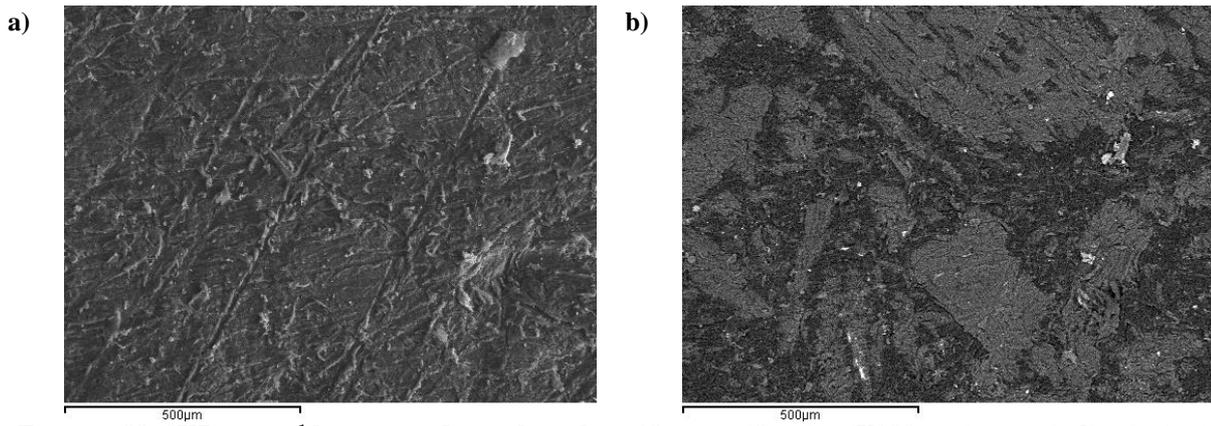
**Figure 4.33:**  $2 \times 75 \text{ mm s}^{-1}$  heat treated sample under X134 magnification (X100 equipment indication). a) Backscattered image of the surface. b) same region seen as a secondary electron image
