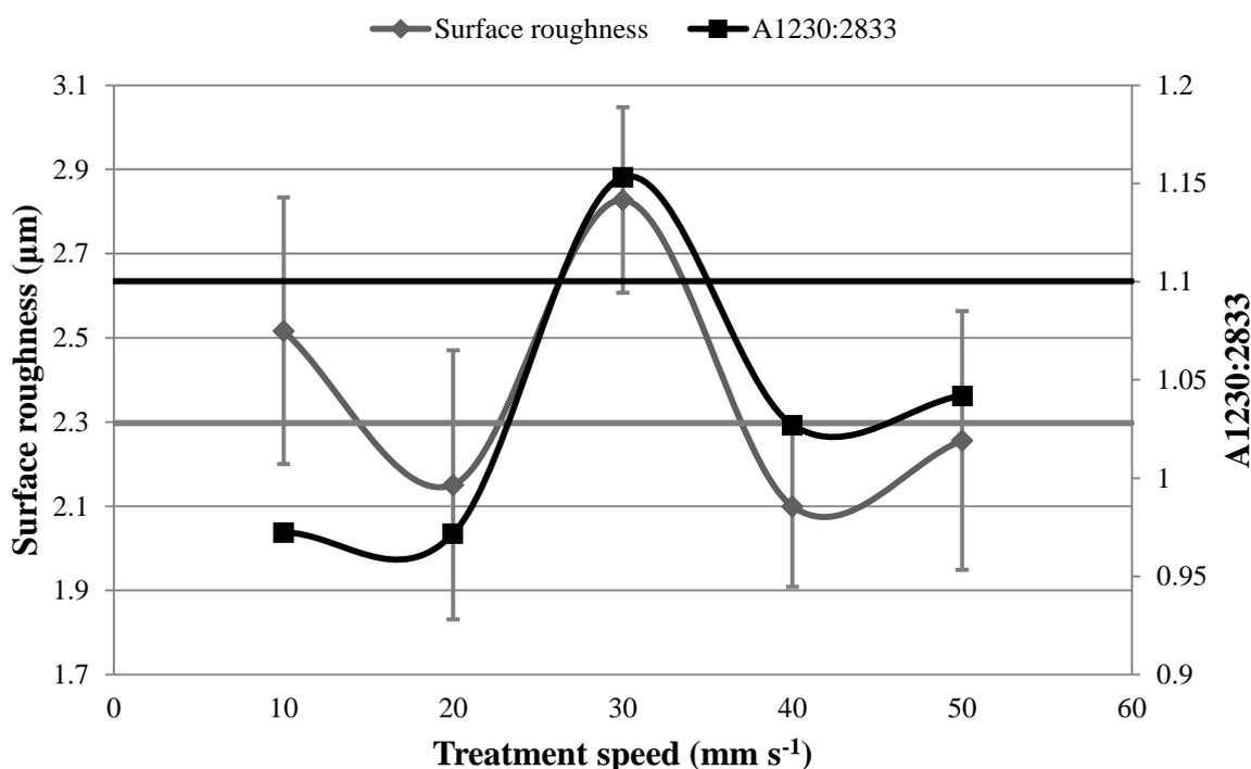
**Figure 5.23: Lignin ratio ( $A_{1230:2833}$ ) compared to surface roughness of the samples treated with halogen heating lamps. The linear lines present the surface roughness (gray line) and the  $A_{1230:2833}$  (black line) control values. Error bars represent the SD (+/-1).**
