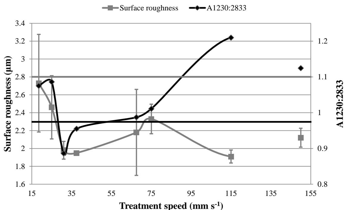
**Figure 5.15: Lignin ratio ( $A_{1230:2833}$ ) compared to surface roughness of the samples treated with hot air. The values at the treatment speed of  $150\text{ mm s}^{-1}$  are referring to the treatment with 2 times pass of the hot air gun with the speed of  $75\text{ mm s}^{-1}$ . The linear lines present the surface roughness (gray line) and the  $A_{1230/2833}$  (black line) control values. Error bars represent the SD (+/-1).**
