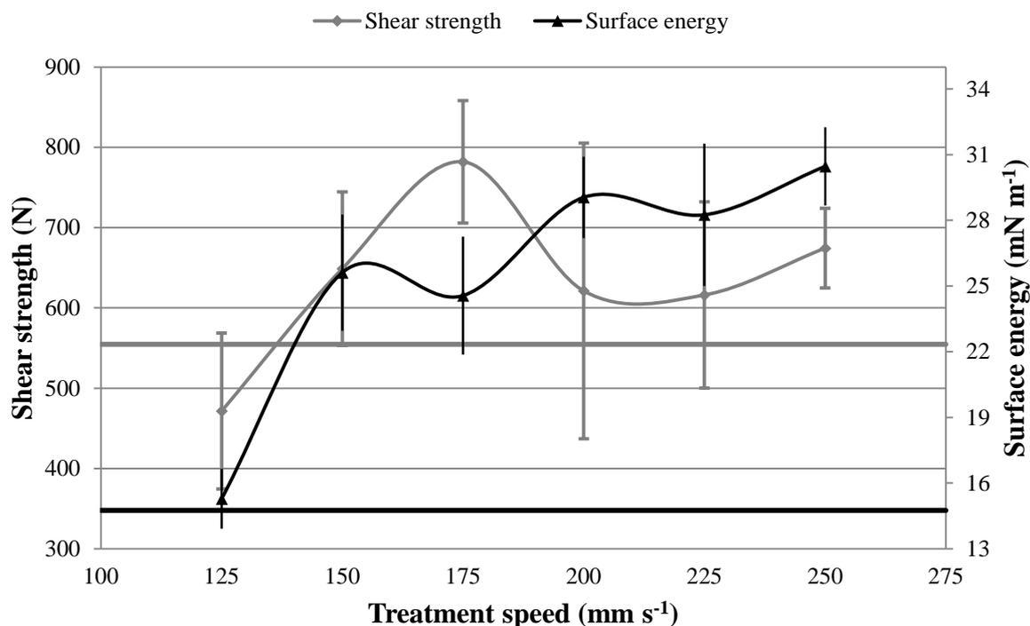
**Figure 5.16: Adhesion strength compared to surface energy of flame treated samples. The linear lines present the shear strength (gray line) and the surface energy (black line) control values. Error bars represent the SD (+/-1).**
