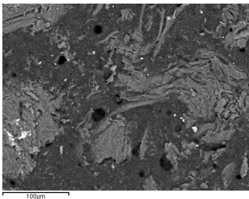
**Figure 4.44: Secondary electron scanning microscopy of 175 mm s<sup>-1</sup> heat treated sample under X400 magnification (X300 equipment indication).**
