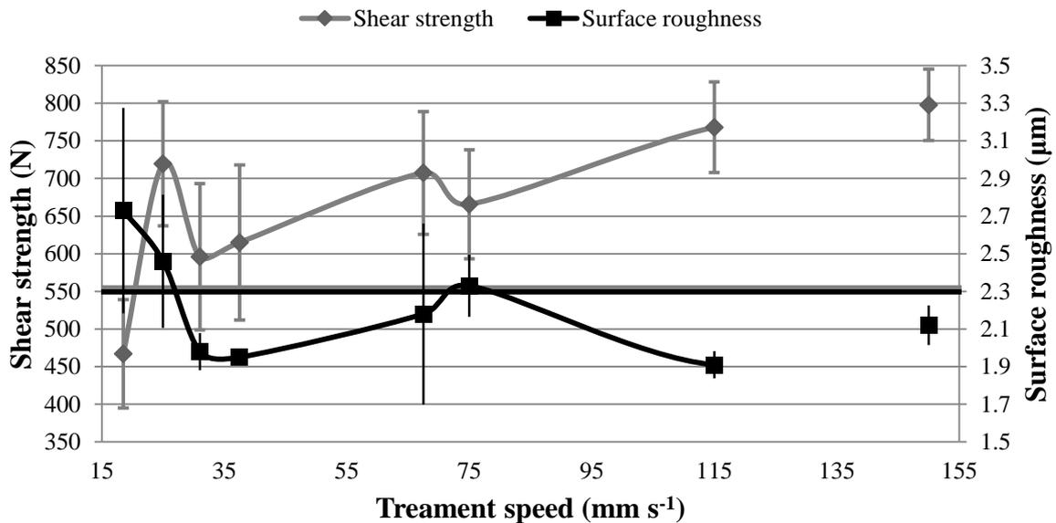
Figure 5.2: Hot air treatment shear strength and surface roughness chart. The values at the treatment speed of 150  $\text{mm s}^{-1}$  are referring to the treatment with 2 times pass of the hot air gun with the speed of 75  $\text{mm s}^{-1}$ . The linear lines present the shear strength (gray line) and the surface roughness (black line) control values. Error bars represent the SD (+/-1).
