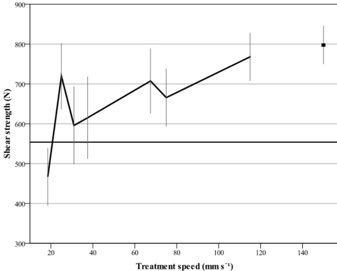
**Figure 4.3: Hot air treatment lap joint tensile strength (N). The mean value at the 150 mm s<sup>-1</sup> treatment speed refers to the samples treated twice with the speed of 75 mm s<sup>-1</sup>. The flat line present the control mean value (554.70 N). Error bars represent the SD (+/-1).**
