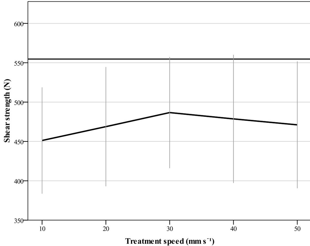
**Figure 4.5: Halogen heat lamp treatment lap joint tensile strength (N). The flat line present the control mean value (554.70 N). Error bars represent the SD (+/-1).**
