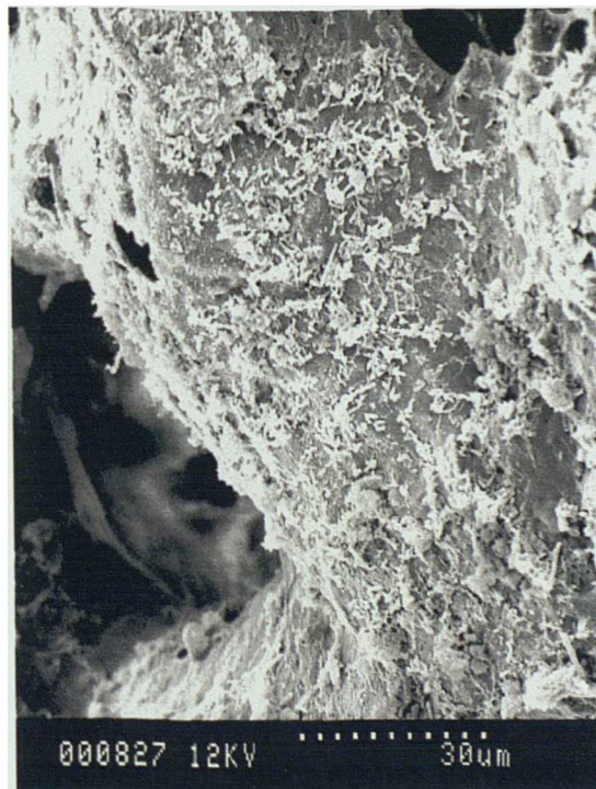
Figure 5.1 Scanning electron micrographs (SEMs) of Poraver beads used for colonising aSRB in bioreactor systems (Kolmert, 1999). Scales are shown in \mu\text{m} . (a) A Poraver bead before colonisation; figure shows the porosity of the solid matrix. (b) The surface of a Poraver bead colonised with aSRB.
