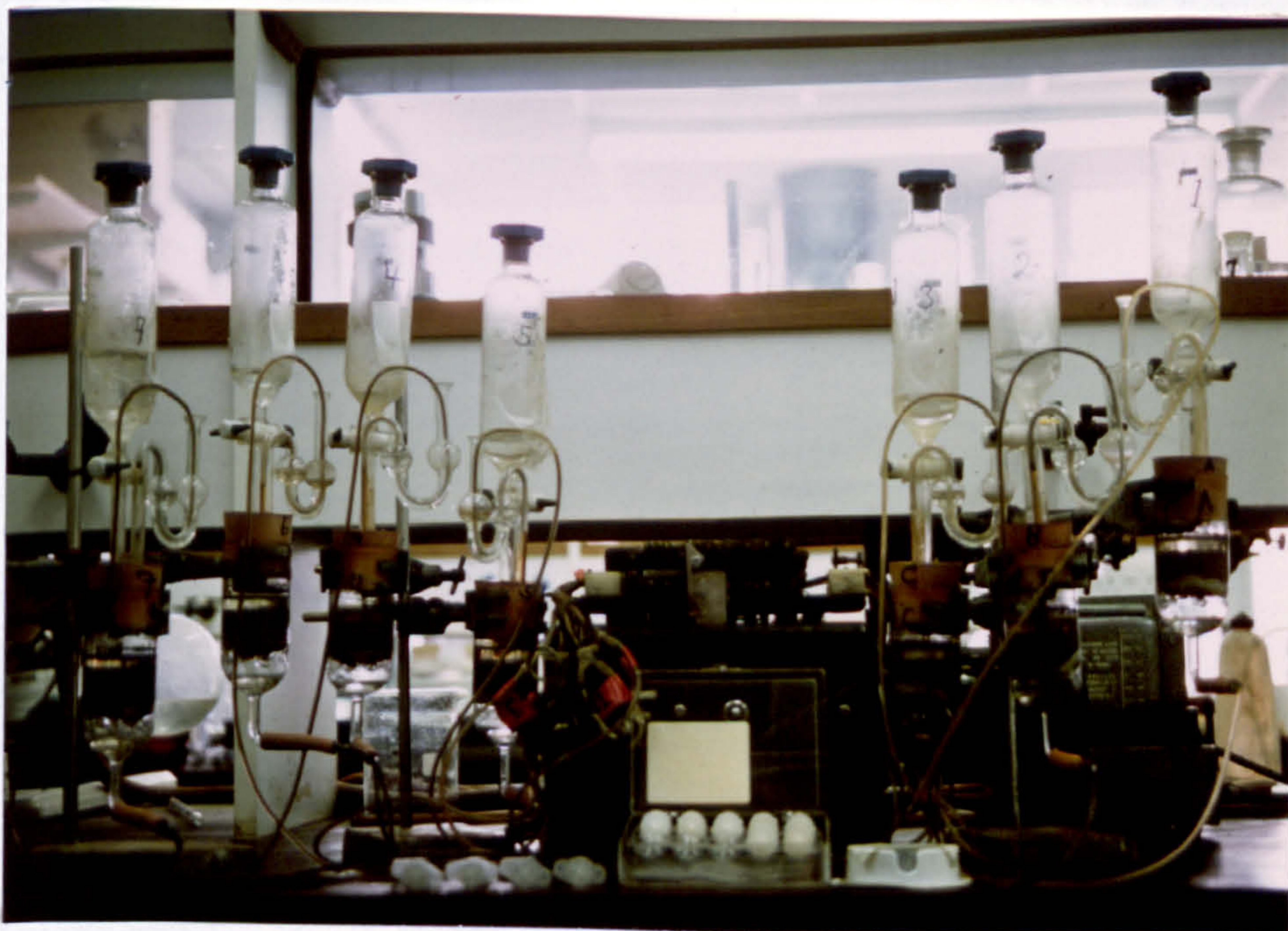
Photo 2.3.1 shows the anaerobic culture equipment
