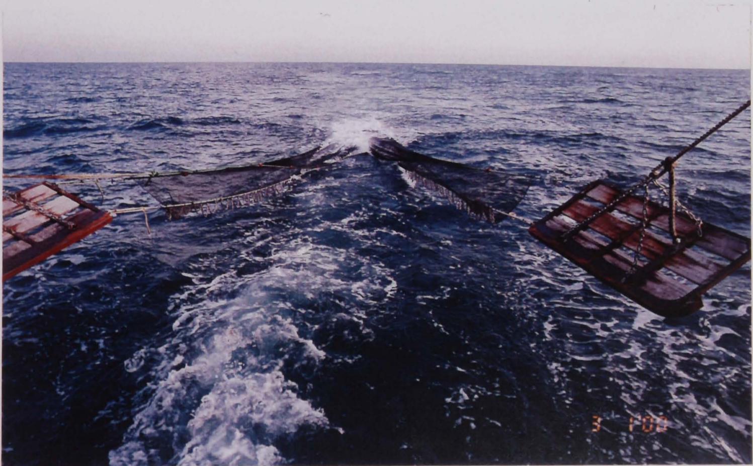
Photograph 2.2. A 29 metre foot-rope Gulf of Mexico flat otter board trawl, in operation during the present study. The two metre otter boards are shown.
