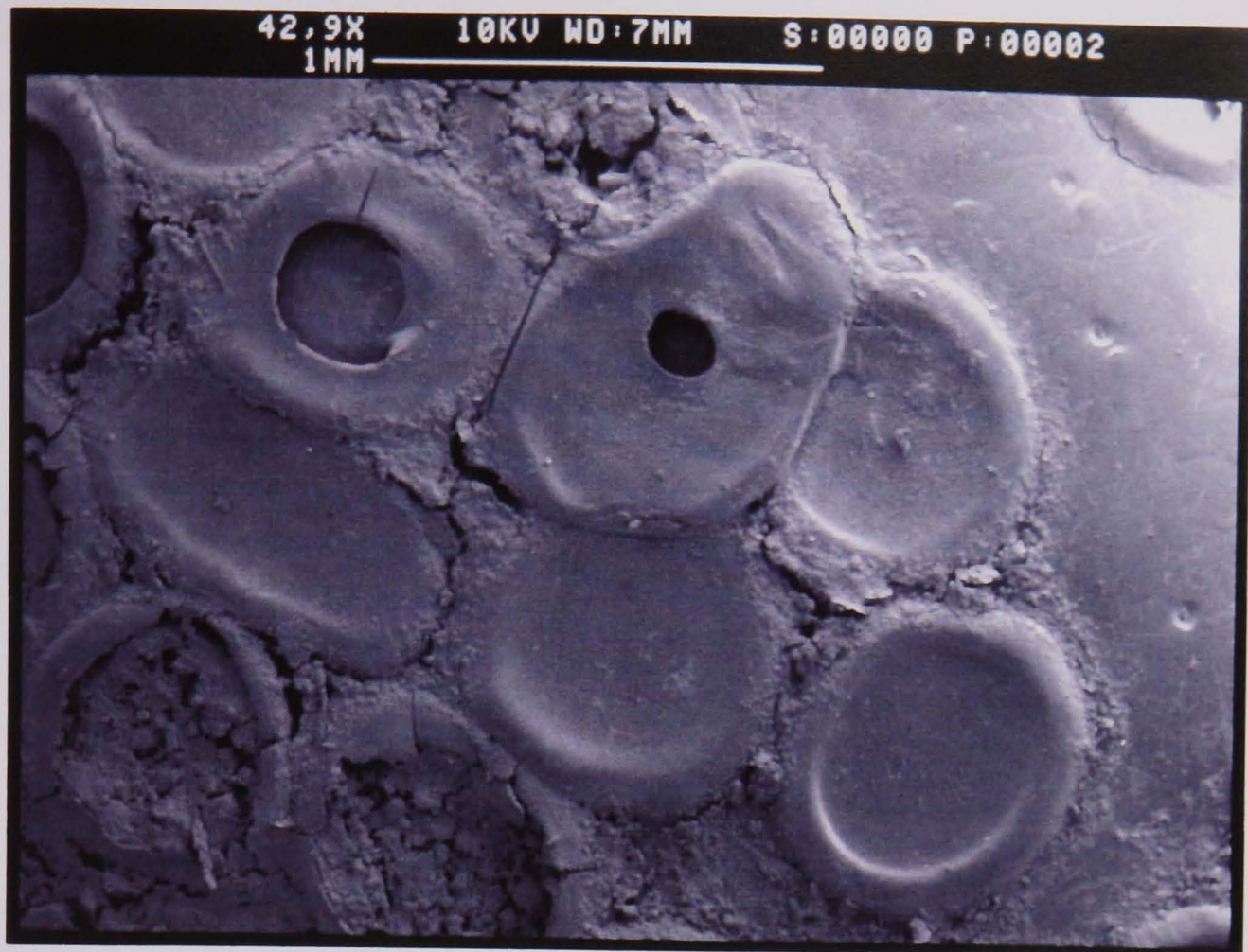
Photograph 6.3. Scanning electron micrograph to illustrate the dense bacterial biofilm on the cuticle that causes the Pink Spot Shell Disease for Portunus pelagicus in Bahraini waters.
