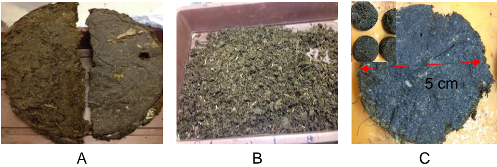
Photos of intact crust and homogenies crust during oxidation study. A, Original crust obtained from winter storage in PVC container. Left side; crust bottom surface, Right side; top crust surface; B, Homogenized crust that was sieved through 56 mm sieves. C: Intact crust in a disc form with 5 cm diameter prepared by using 5 cm diameter soil metal bulk density ring.
