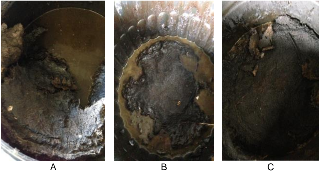
Figure 6.2 Crust formed from 90 litres barrel over 6 months' periods and treated with AFEM additives.
