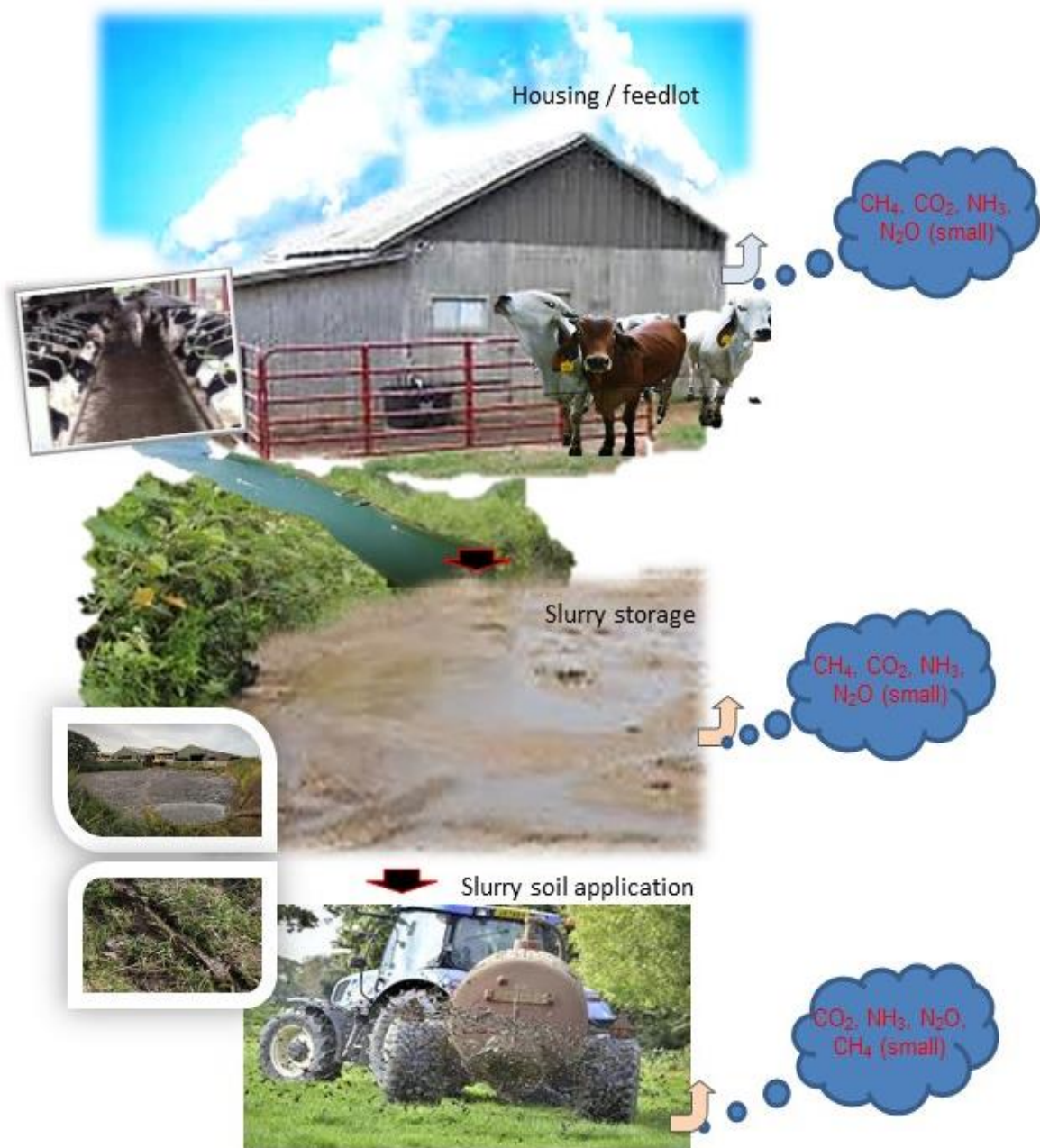
Figure 2.3 Schematic diagrams of common cattle slurry management and GHG pollution.
