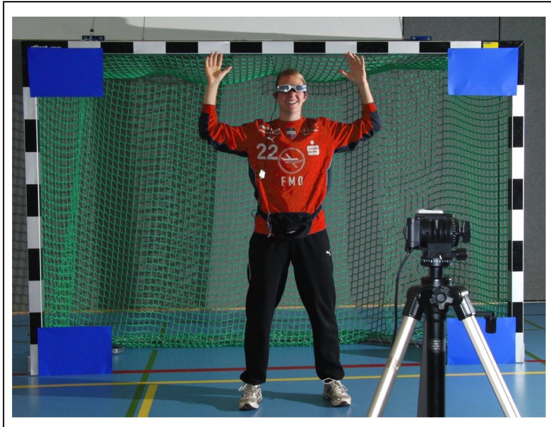
Figure 2.7: Virtual handball; note the blue detection patches in the four corners of the goal; picture courtesy of Bolte et al. (2010).
