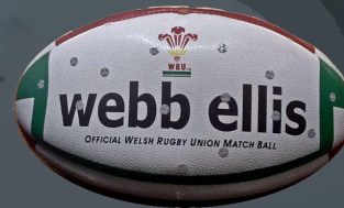
Match Rugby Ball with Reflective Markers Applied for Optical Tracking
