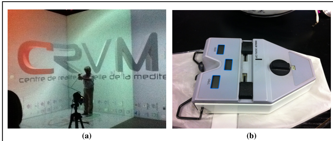
Figure 4.6: (a) Calibrating the ART system with the calibration wand. (b) The Essilor Digital CRP used to measure participant's interpupillary distance.
