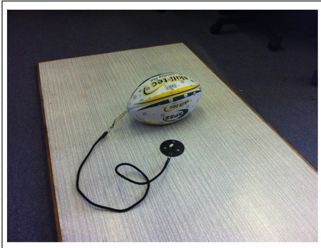
Figure 3.4: Skill-tec training ball anchored to the ground with a large flat board.
