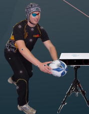
Physics modelled virtual ball follows trajectory the real ball would have PST captures position and speed of ball as thrown – ball is tethered
