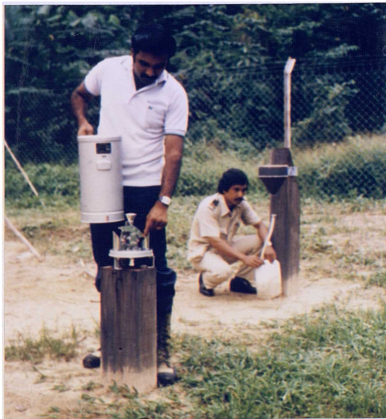
Plate 4.2 Recording and storage raingauges installed in BEW
