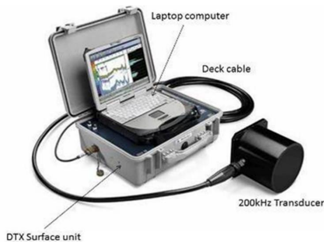
Figure 2.1 Biosonics DTX Split beam echosounder (200 kHz) used for all the surveys in this thesis.
