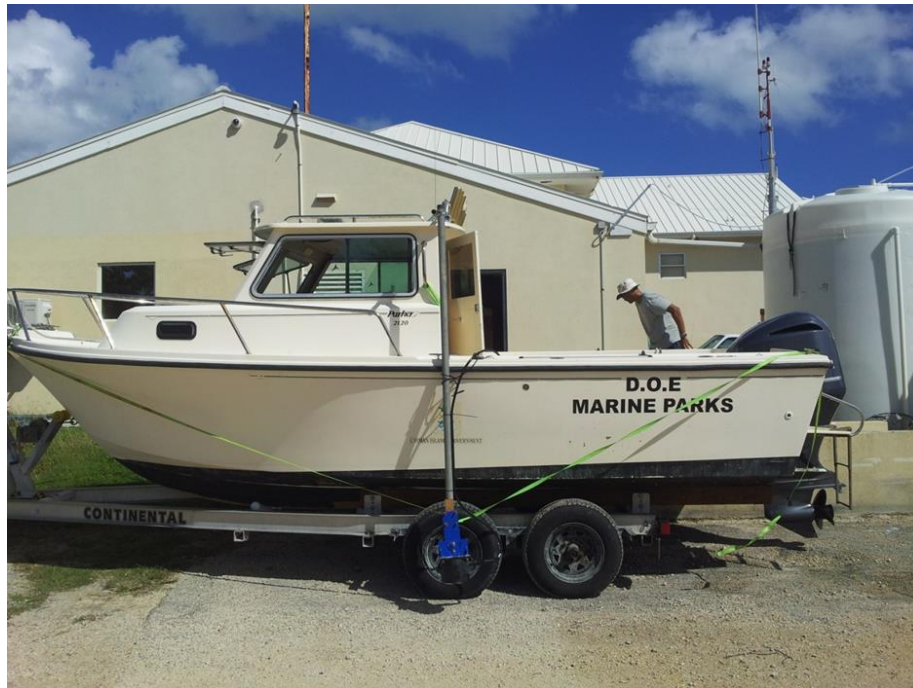
Figure 2.2 Example of how the echosounder transducer was pole mounted over the side of the survey vessels.
