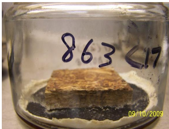
Figure 5.1: Arrangement of boards for fungi exposure test: (A) virulence of fungi, (B) decay of wood particles, and (C) decay of particleboards
