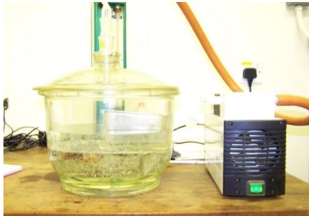
Figure 3.2: Water absorption apparatus
