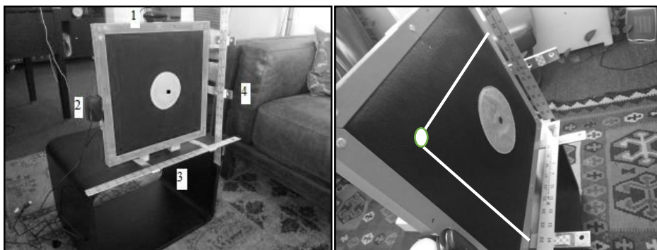
Figure 1. (1) x-axis webcam, (2) y-axis webcam, (3) x-axis ruler, (4) y-axis ruler.
