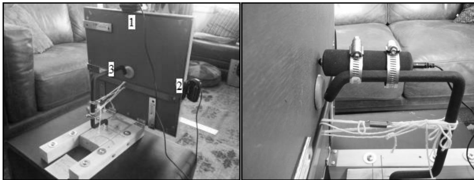
Figure 2. (1) x-axis webcam, (2) y-axis webcam, (3) push-button switch.
