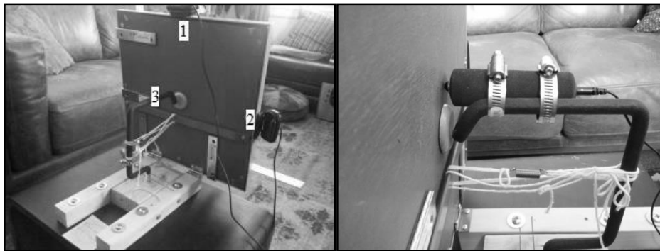
Figure 2. (1) x-axis webcam, (2) y-axis webcam, (3) push-button switch.
