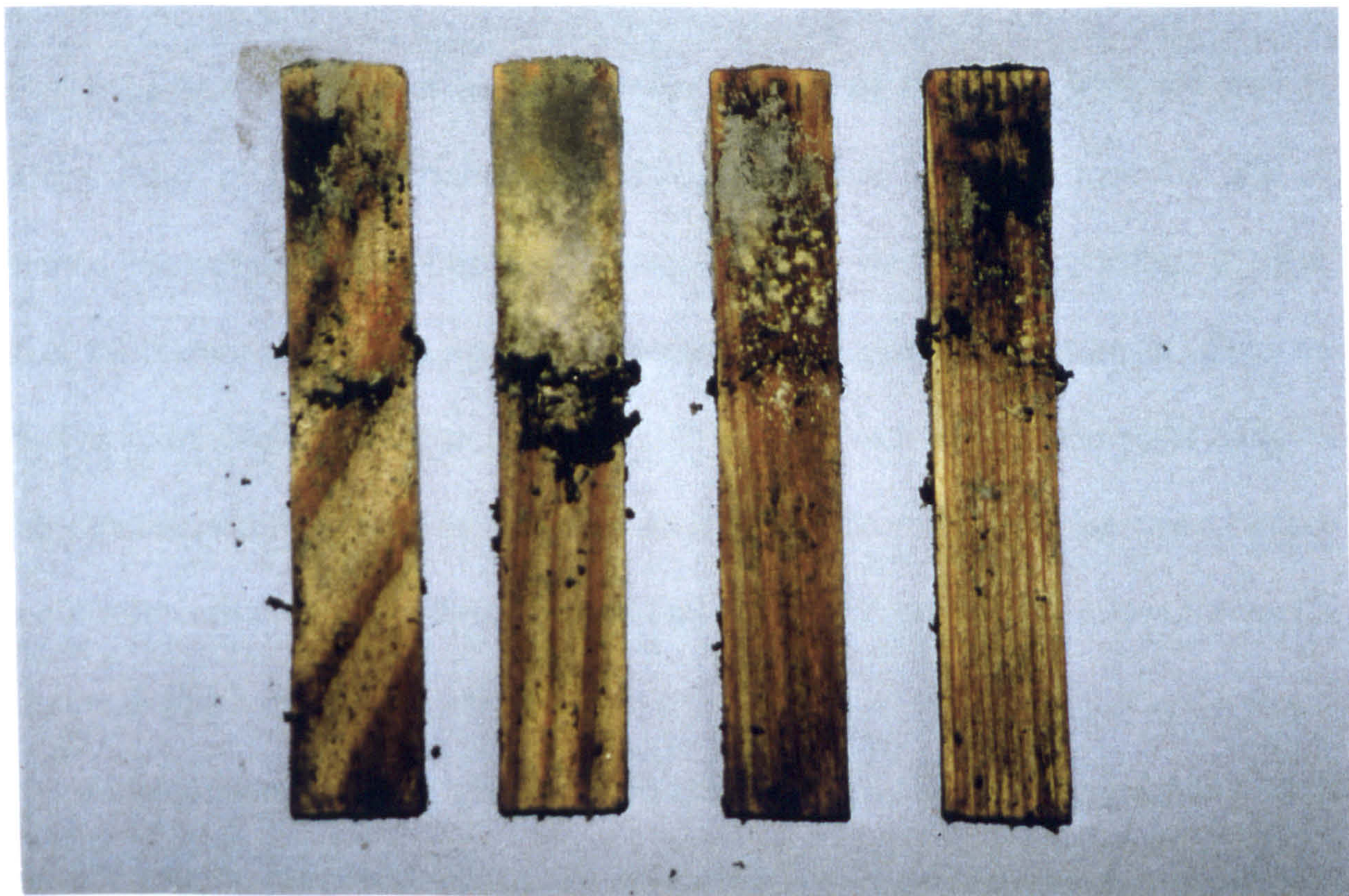
Plate 7.1 Mould growth on succinic anhydride modified stakes.
