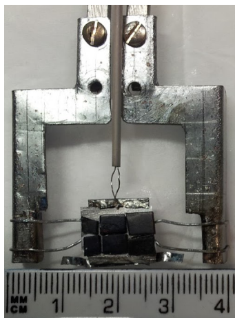
Figure 5.2: Samples mounted on heating stage for NEXAFS characterisation.
