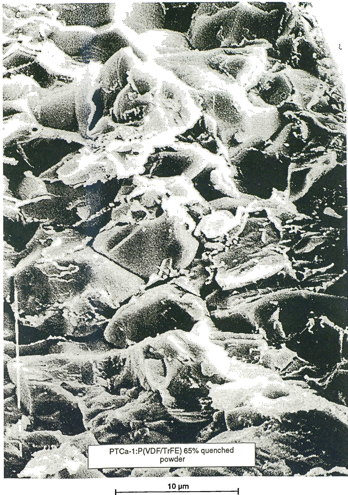
Figure 3.16 - SEM micrographs of a composite made from PTCa-1 quenched powder at 65% loading. Magnification: x5150.
