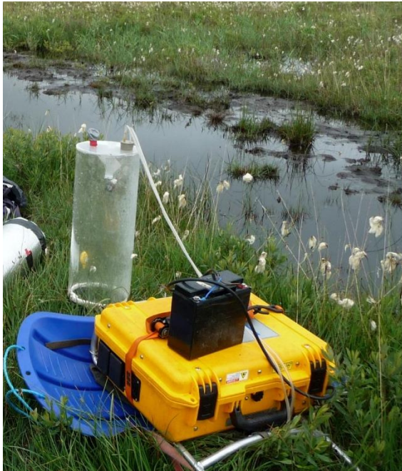
Fig. B1: Manual chamber measurement set up; Clear Perspex chamber (NEE) equipped with fan and pressure equalisation balloon attached to the Los Gatos Ultra Portable GHG Analyser. Picture taken on the bund in RW-15.
