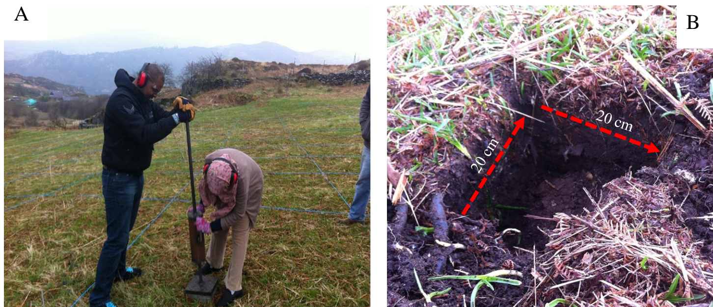
Figure 20. (A) Stainless steel square hollow section (20 cm x 20 cm x and 30 cm) being inserted into the soil to collect sample (B) Sample core removed
