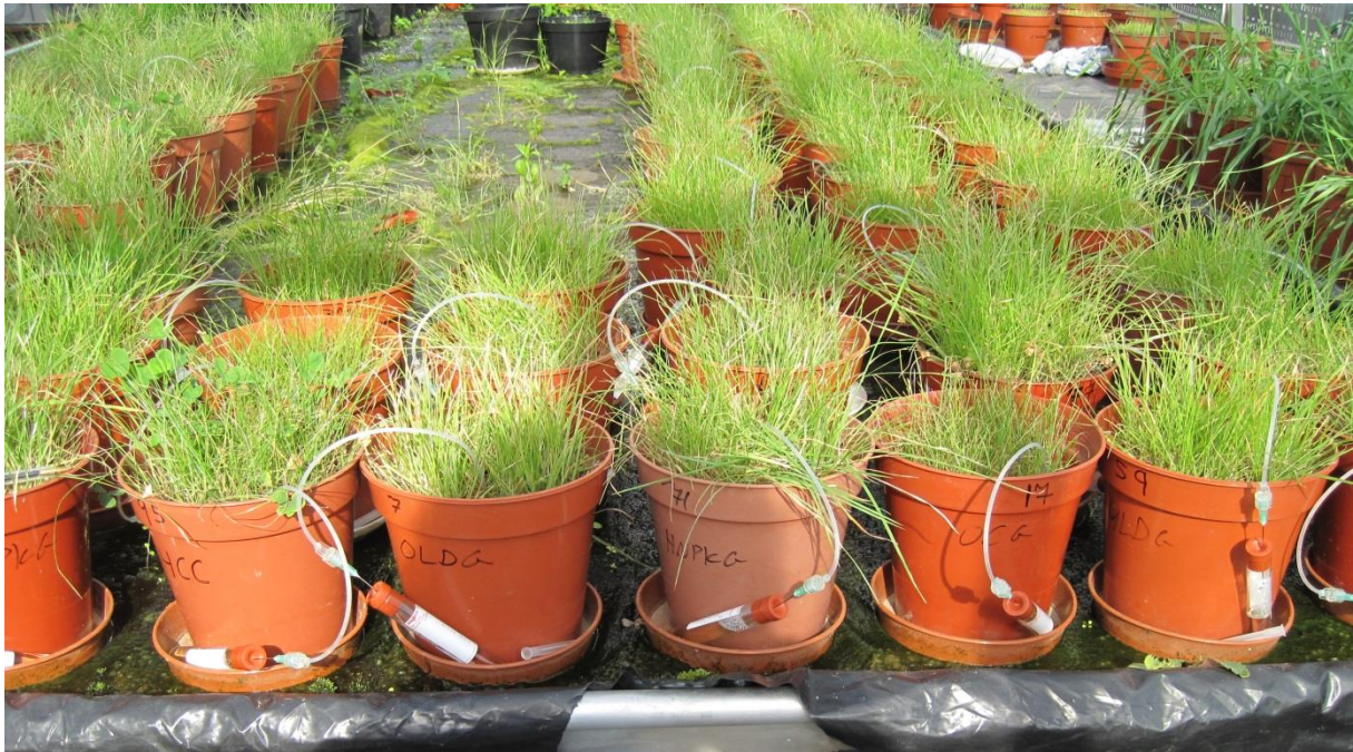
Picture 4.3: Pots with Rhizon® samples and vacuum tubes attached from nutrient analysis
