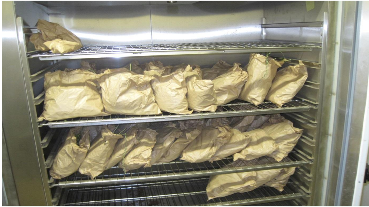
Picture 6.4: Wet samples (each 300 g from one meter squared plot), dried for further analysis
