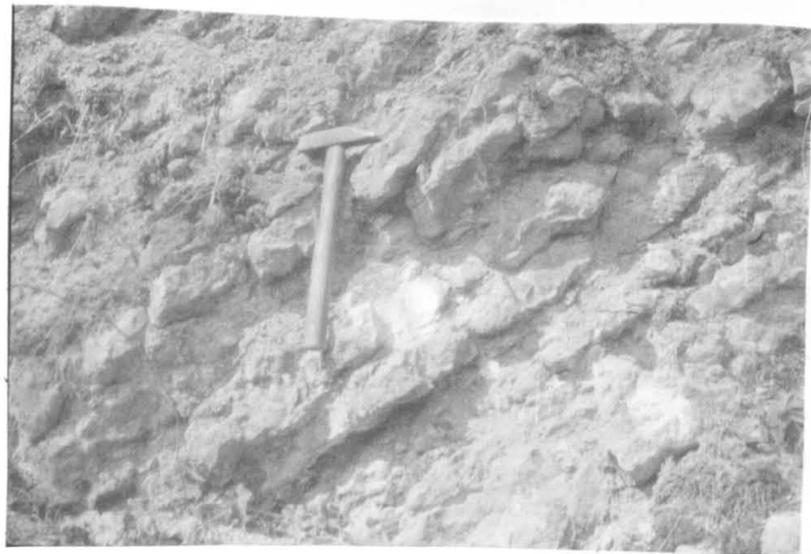
Fig. 87 Fownhope Quarry 2. View of blocky limestone alternating with shale in the higher horizons.
